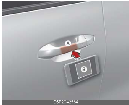
[A]: Door handle authentication pad [B]: NFC antenna (Backside of the smart phone) (The antenna position differs depending on models.)
