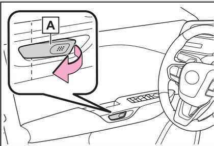
Pull the manual release handle **A** twice to open the door.
