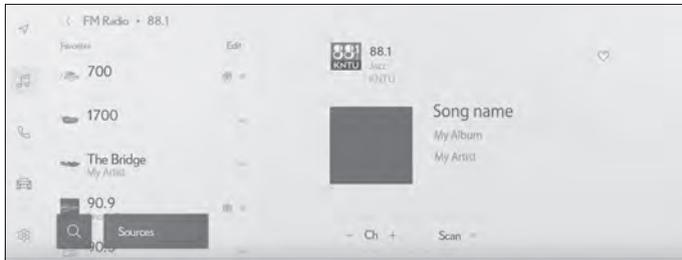
“Ch”: Touch “-” or “+” to search for the receivable broadcasting stations. Touch and hold to jump to the next frequency with available radio signal. When released, the broadcasting station closest to that position with the best reception sensitivity is selected automatically.
