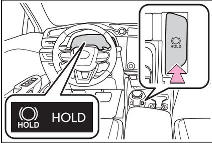
Turns the brake hold system on
