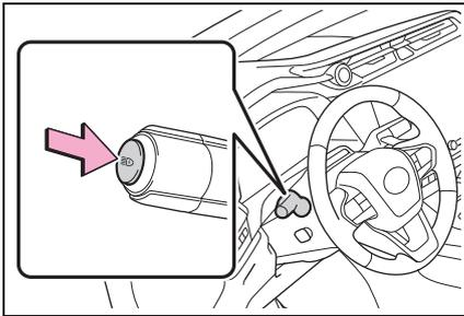
Press the Automatic High Beam switch.
