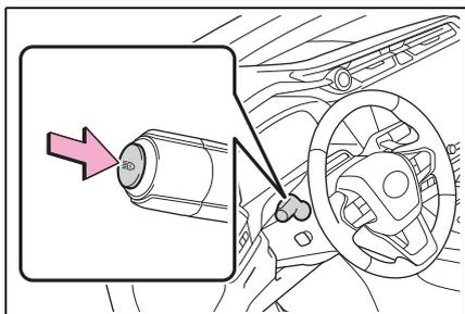
Press the Adaptive High-beam System switch.
