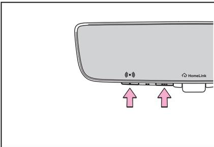
Press and hold the 2 outer HomeLink<sup>®</sup> buttons for 10 seconds. Check that the HomeLink<sup>®</sup> indicator light changes from continuously lit in orange to rapidly flashing in green. All codes registered to memory will be erased.
