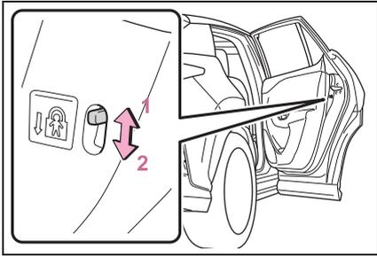
The door cannot be opened from inside the vehicle when the lock is set.
