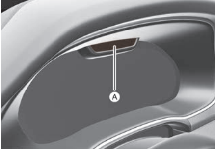
[A] Interior view camera
