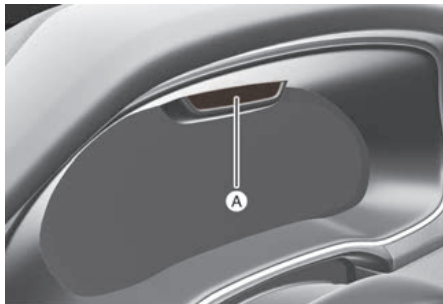
[A] Interior view camera
