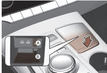
[A] Indicator light [B] Charging pad
