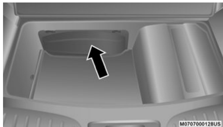
Jack Storage Location
