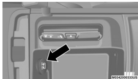
Front Center Console Outlet
