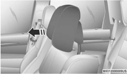
Active Head Restraint (Tilted)
