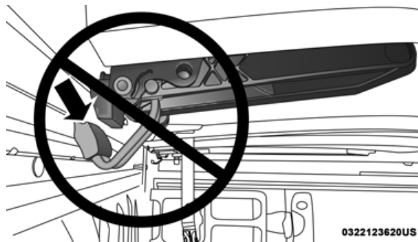
Improper Clamp Position
