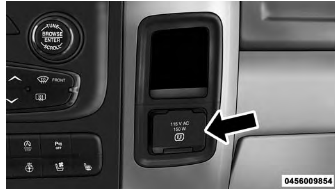
Power Inverter Outlet
