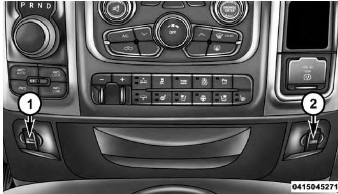
Power Outlets — Center Stack
