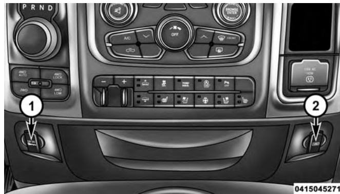
Power Outlets — Center Stack
