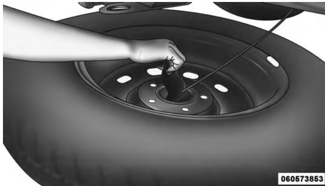
Reinstalling The Retainer
