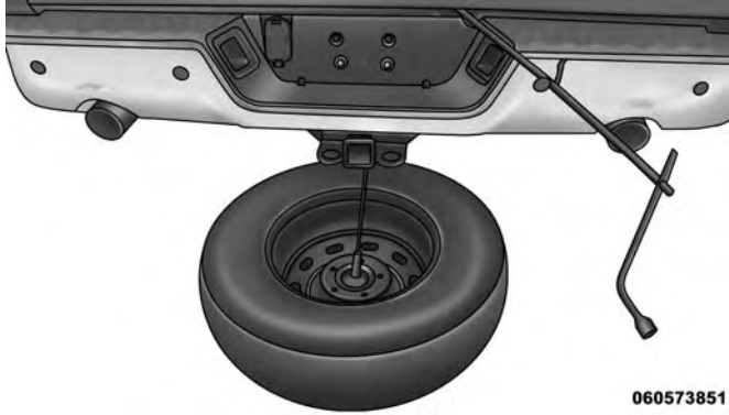
Pulling The Spare Tire Out
