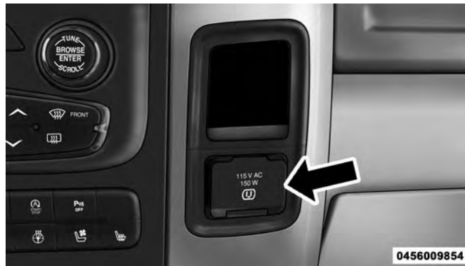
Power Inverter Outlet
