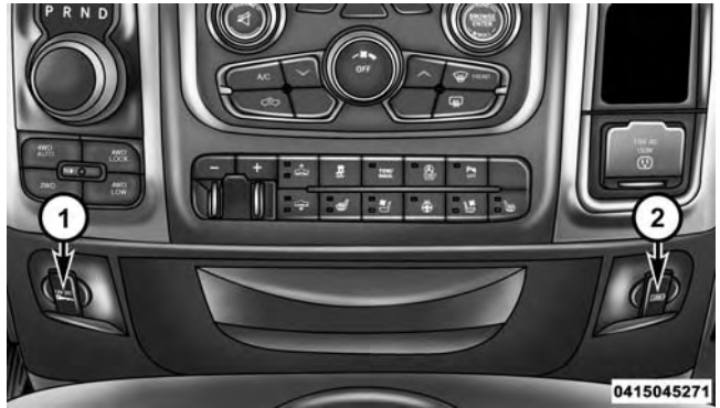
Power Outlets — Center Stack
