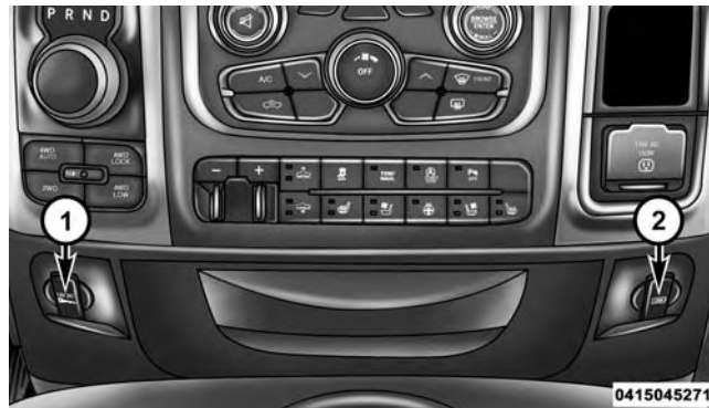
Power Outlets — Center Stack
