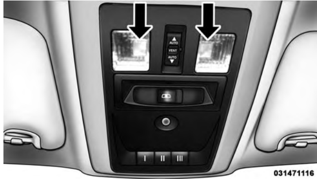
Front Courtesy/Reading Lights
