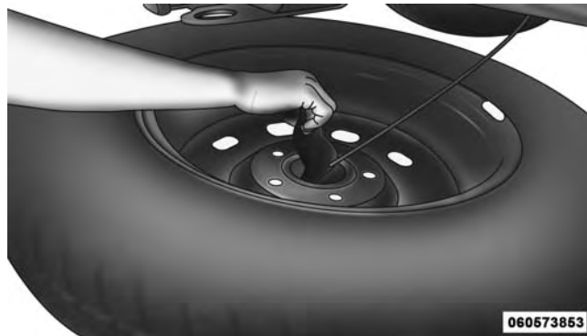
Reinstalling The Retainer
