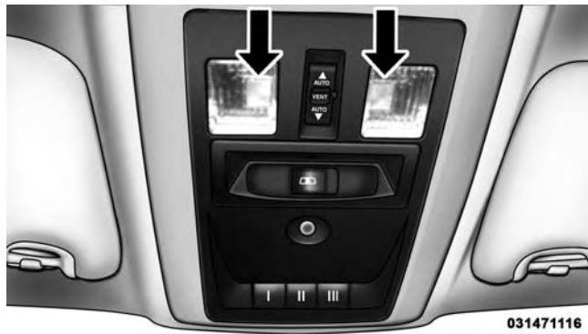
Front Courtesy/Reading Lights
