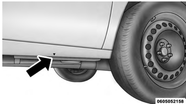
Front Jacking Location
