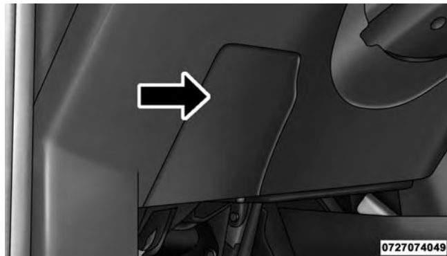
Fuse Panel Cover
