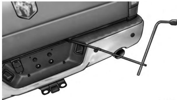
Wheel Wrench And Jack Extension Tube Assembled
