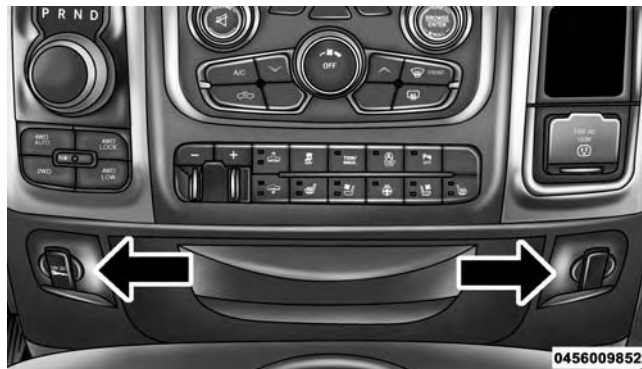
Power Outlets — Center Stack
