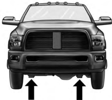
4x4 Front Jacking Location
