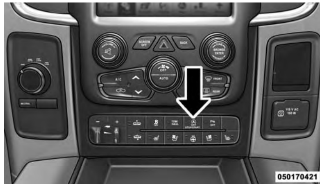
STOP/START OFF Switch
