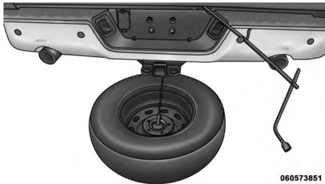
Pulling The Spare Tire Out
