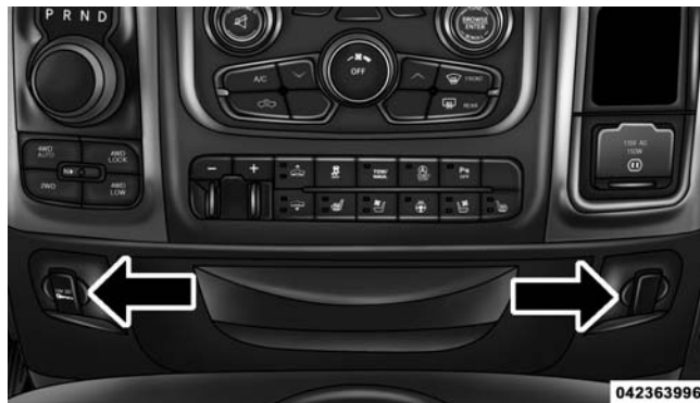
Power Outlets — Center Stack
