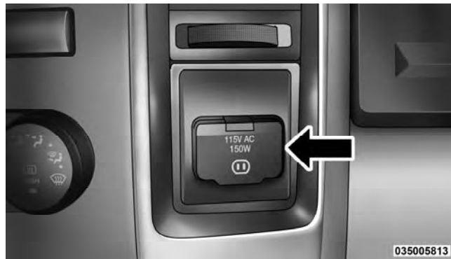
Power Inverter Outlet
