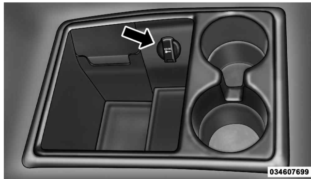
Power Outlet — Floor Storage Bin
