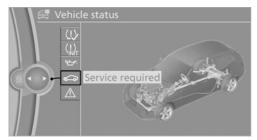
The maintenance system provides information on required maintenance measures and thus provides support in maintaining road safety and the operational reliability of the vehicle.
