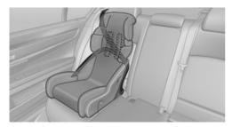
The rear safety belts and the safety belt for the front passenger can be locked to prevent extension in order to permit attachment of child restraint fixing systems.
