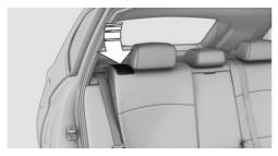
Reach into the recess and pull the lever toward the front. Engage the backrest in the desired position or fold it down.
