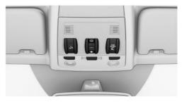
The indicator lamp for the front passenger airbags indicates the operating state of the front passenger airbags.
