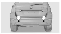
The anchorage points are under the covers in the bumper. Remove the covers, refer to page 260.
