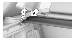
2. Pull the cover back, up and out of the lateral brackets on both sides, arrow 2.
