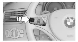
Press the computer button in the turn signal lever.
