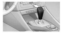
A lock prevents you from inadvertently engaging selector lever positions R and P. To cancel the lock, press the button on the front of the selector lever, see arrow.
