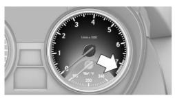
Never force the engine speed up into the red warning field, see arrow. In this range, the fuel supply is interrupted to protect the engine.
