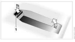
2. Insert the snap-in adapter at the front, arrow 1, and press down, arrow 2, until it engages.
