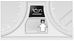
⚠ The symbol indicates that Check Control messages have been stored. The Check Control messages can be displayed later.
