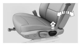
Pull lever 3 and apply your weight to the backrest or lift it off, as necessary.
