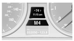
The transmission position is displayed and the engaged gear, such as M4, is displayed in manual mode.
