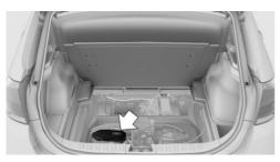
The tool kit is stowed under the cargo floor panel and storage compartment in the cargo area.
