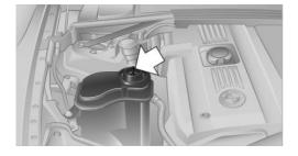
The filling level indicator 1 in the filler neck indicates the coolant level. The coolant level is correct if it is between the arrows of the respective reservoir label 2.
