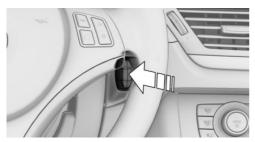
Insert the remote control all the way into the ignition lock.
