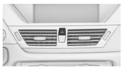
The button for the hazard warning system is located on the center console.
