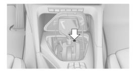
Using the screwdriver from the tool kit, refer to page 247, press the red lever while moving the selector lever to the desired position with the button pressed.
