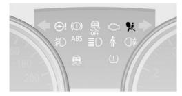
When the ignition is switched on,, refer to page 58, the warning lamp comes on briefly to indicate that the entire airbag system and the belt tensioners are operational.
