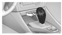
Push the selector lever to the left out of transmission position D.
