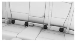
The mounts for the lower LATCH anchors are located behind the indicated cover caps.
