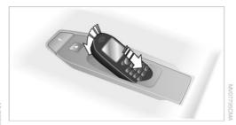
The battery is charged beginning with the radio ready state of the vehicle.
