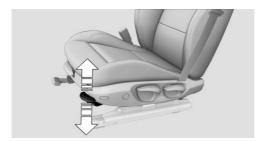
Pull the lever and apply your weight to the seat or lift it off, as necessary.
