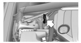
The so-called starting aid terminal in the engine compartment acts as the battery's positive terminal. Pull the cover up and off.
