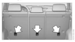
There are three mounting points, see arrows, for the upper retaining strap of LATCH child restraint fixing systems.
