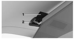
Attach the hooks 1 at the bottom of the retaining straps into the eyelets on the rear seat backrest, arrow, on both sides.
