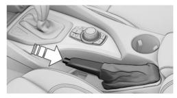
Pull up slightly, press the button, and lower the lever.
