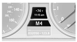
The selector lever position is displayed and the engaged gear, such as M4, is displayed in manual mode.
