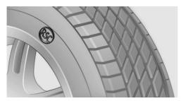
RSC label on the tire sidewall.
