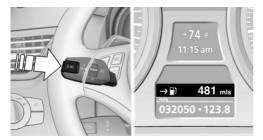
Press the computer button on the turn signal lever.
