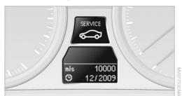
The remaining driving distance and the date of the next scheduled service are displayed briefly immediately after you start the engine or switch on the ignition. The current service requirements can be read out from the remote control by the service specialist.
