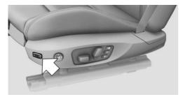
The width of the backrest can be changed with the side wings to adjust the side support to your own needs.
