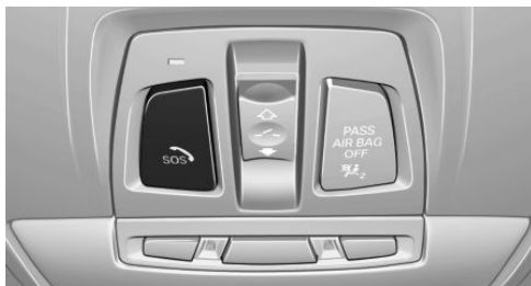
SOS button in the roofliner
