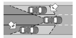
Two radar sensors in the rear bumper monitor the area behind and next to the vehicle starting from a preset minimum speed.
