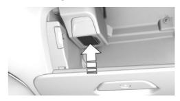
Remove cover of the fragrance cartridge to be inserted. Touch the cover on its top to push it away from the fragrance cartridge, arrow 1.
