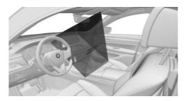
The gestures are captured by a camera in the roofliner.
