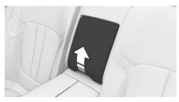
Push the cover up until it engages. There is a storage compartment underneath.
