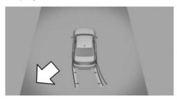
The respective boundary area in the PDC view flashes red, if vehicles are detected by the sensors.
