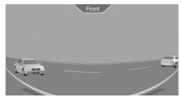
The system provides an early look at cross traffic at blind driveways and intersections. Road users concealed by obstacles to the left and right of the vehicle can only be detected
