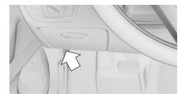
There is an OBD socket on the driver's side for checking the primary components in the vehicle's emissions.
