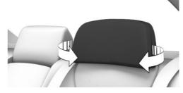
Fold the side extensions on the head restraint forward for increased lateral support in the resting position.
