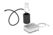
Screw the filling hose of the sealant container onto the tire valve of the nonworking wheel.
