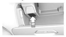
Fragrance cartridge, arrow 1: corresponds to the first fragrance indicated on the Control Display. Fragrance cartridge, arrow 2: corresponds to the second fragrance indicated on the Control Display.
