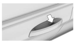
Touch the grooved surface on the handle of a closed vehicle door, arrow, with your finger and hold it there without grasping the door handle.
