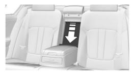
3. Pull handle down, arrow 1, and fold panel forward, arrow 2.
