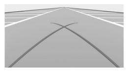
Turning circle lines can only be superimposed on the rearview camera image together with pathway lines.
