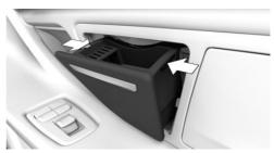
Grasp the insert on the side, arrows, and remove it.
