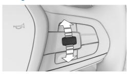
On the right side of the steering wheel, turn the thumbwheel to activate the corresponding list.
