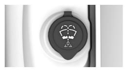
All washer nozzles are supplied from one reservoir in the engine compartment.
