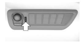
Thumbwheel for changing the air flow direction.
