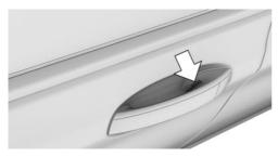
Touch the grooved surface on the handle of a closed vehicle door, arrow, with your finger for approx. one second without grasping the door handle.
