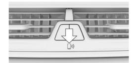
The NFC antenna is in the instrument panel below the hazard warning flashers.
