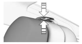
The head restraint folds into the topmost position. Close the pushbutton on the lower tab and the pushbutton on the bottom of the head restraint.
