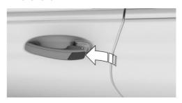
Guide one finger of the other hand from the back under the lid, push the palpable release outward and remove the lid.
