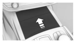
Push the cover forward until it engages behind the cup holders. Push the cover forward again until it engages behind the storage compartment.
