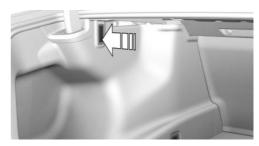
A multi-function hook is located on the left side in the trunk. Press on the multi-function hook and turn until it engages.
