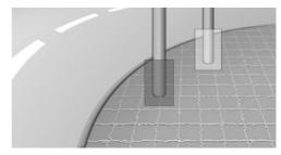
Obstacles behind the vehicle are detected by the PDC sensors.
