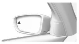
The lamp in the exterior mirror flashes if vehicles are detected by the rear sensors and the vehicle is moving backwards.
