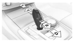
Briefly push the selector lever in the desired direction, beyond a resistance point if needed.
