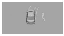
Obstacle markings are displayed sideways on the vehicle to protect the vehicle sides.
