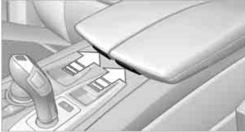
Push cover down slightly and press the button. The cover folds upward.
