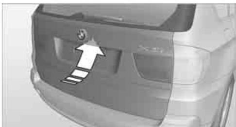
Press the button on the liftgate or the
