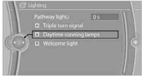
Daytime driving lamps are activated and are stored for the remote control currently in use.
