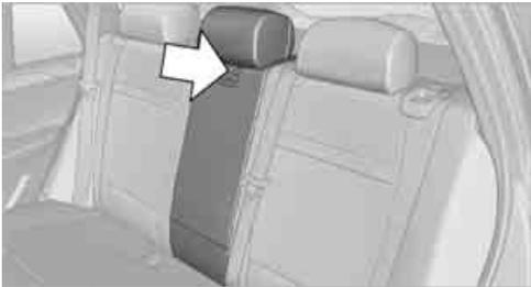
Unlock the center armrest with the button in the lower section of the opening and fold down.
