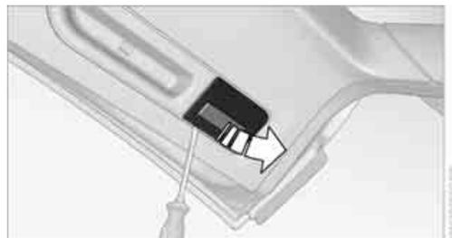
2. Push the catch on the bulb holder to the left, arrow, and remove it.
