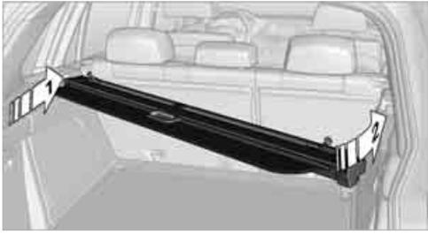
1. Lay on the case on the left-hand side and push it forward, arrow 1.
