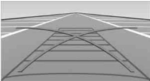
2. Turn the steering wheel so that the pathway lines coincide with the corresponding turning line.
