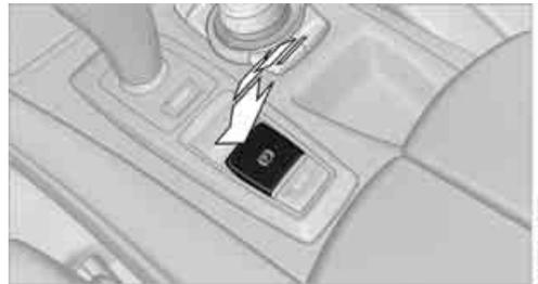
Press the button with the brake depressed.
