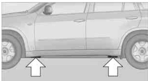
2. Guide the jack head into the rectangular recess of the jacking point when cranking up, refer to illustration detail.
