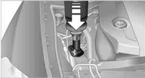
3. The reservoir is full when the fill level in the bottle stops changing. It is not possible to overfill. Pull bottle back, refer to arrow, and unscrew it.
