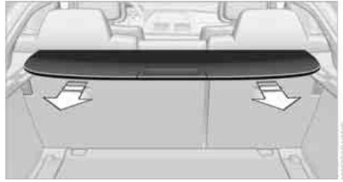
1. Grasp retracted cargo area cover underneath the upper fold on both sides.
