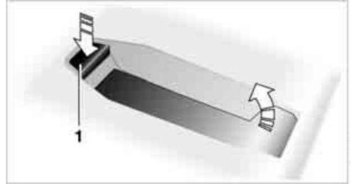
2. Insert the snap-in adapter in the front and press it downward until it engages.
