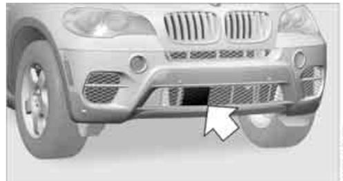
The radar sensor is integrated in the bumper.
