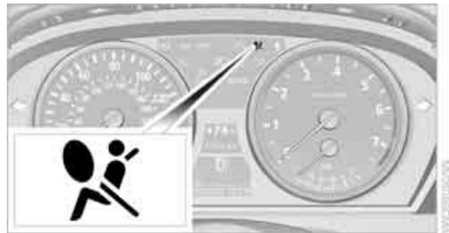
From radio readiness, refer to page 58, the warning lamp lights up briefly, indicating the operational readiness of the entire airbag system and the safety belt tensioners.
