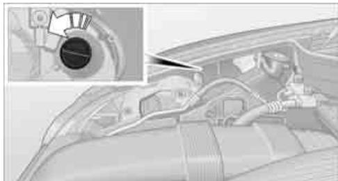
2. Rotate the bulb to the right along with the socket and replace.
