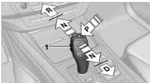
Briefly press the selector lever in the desired direction, beyond a resistance point if necessary. When shifting out of P or into R, simultaneously push the unlock button 1.
