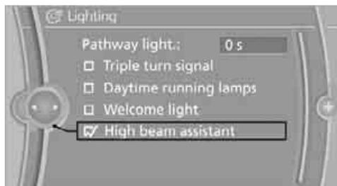
**✓** High-beam Assistant is activated and is stored for the remote control currently in use.
