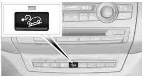
Press the button; the LED lights up. The HDC display is shown in the instrument panel.
