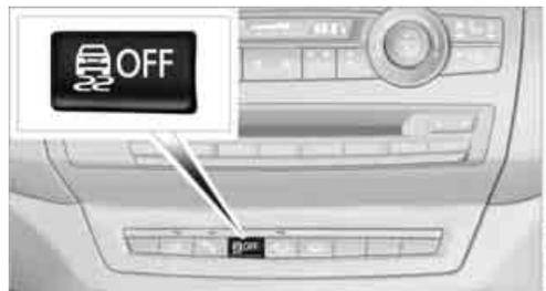
Press the button: the indicator lamp for DSC lights up and TRACTION appears in the instrument panel.
