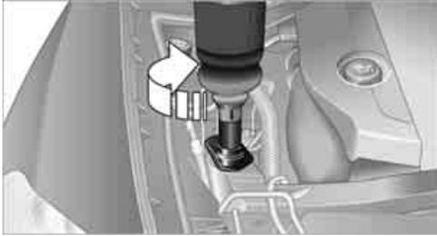
2. Press bottle down, refer to arrow. The reservoir of the vehicle is filled.
