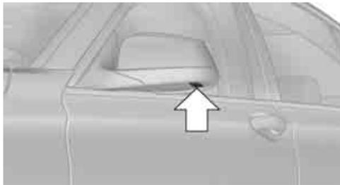
The lenses of the Top View cameras are on the undersides of the exterior mirror housings.
