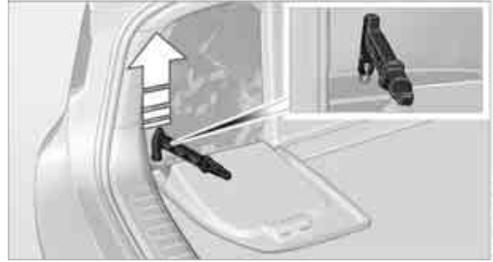
4. Firmly pull the releasing tool upward against the mechanical resistance, refer to arrow, until a considerable increase in force is felt and the parking brake is then clearly heard to release.
