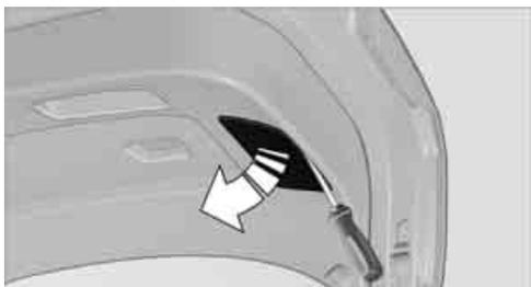
2. Rotate the bulb socket to the left and remove.
