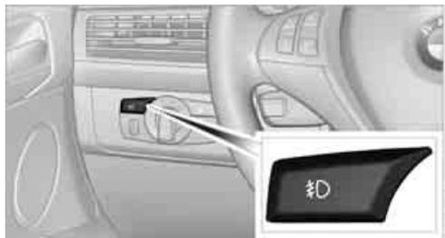
First, switch on the parking lamps or the low beams. The green indicator lamp in the instrument panel lights up whenever the fog lamps are on.
