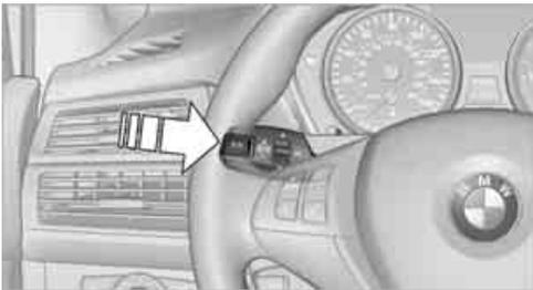
To display the information, press the BC button on the turn signal lever.
