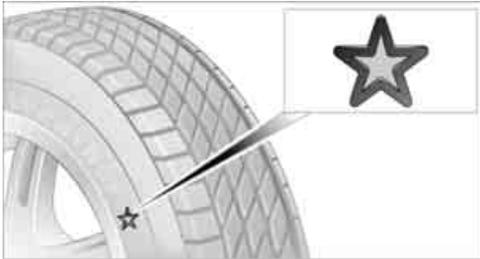
Certain tire makes are recommended by BMW depending on the tire size. You can recognize these from the clearly visible BMW marking on the tire sidewall.
