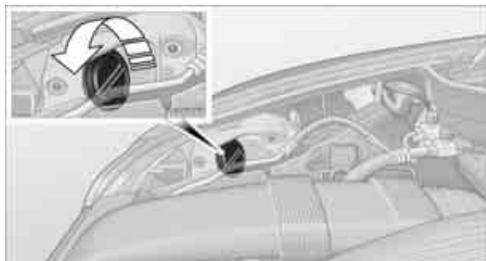
2. Turn the bulbs to the left, pull off the connector and replace.
