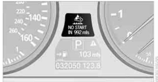
After refilling, the reserve continues to appear after the engine is restarted. After the vehicle has been driven for a few more minutes, this display will disappear.
