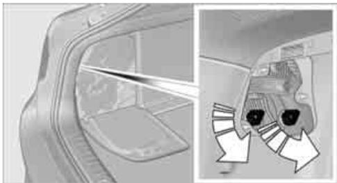
4. Apply gentle pressure to the bulb while turning it to the left for removal and replacement.
