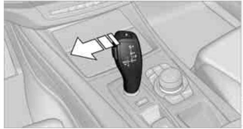
Press selector lever out of transmission position D toward the left:
