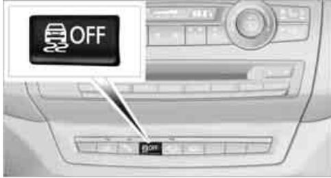
Press and hold the button until the indicator lamp for DSC lights up and DSC OFF appears in the instrument panel, but do not press the button for longer than approx. 10 seconds. DTC Dynamic Traction Control and DSC are deactivated together. Stabilizing interventions are now not carried out.
