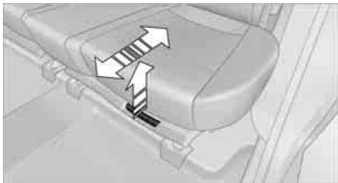
1. Pull the lever and slide the seat into the desired position.
