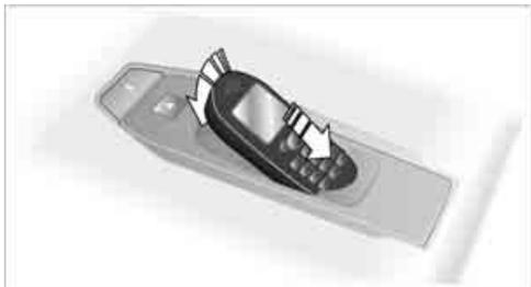
The mobile phone's battery is charged as soon as the vehicle is in radio readiness or the steering is unlocked.
