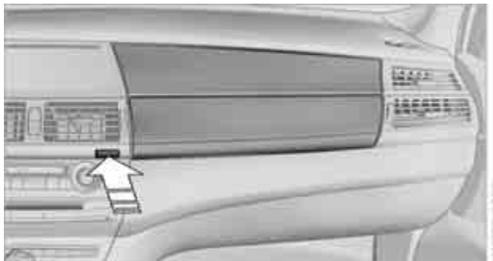
Press the button. The covers open upward and downward and the lighting in the glove compartment switches on.
