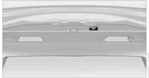
The liftgate closes automatically when you press the button on the inside of the liftgate.
