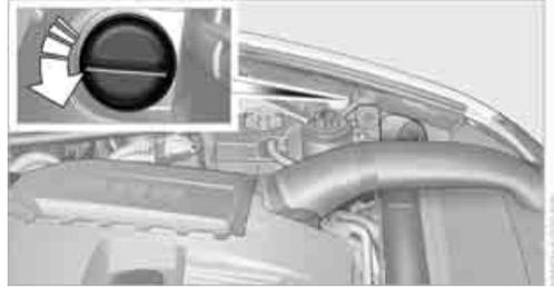
2. Rotate the bulb to the right along with the socket and replace.
