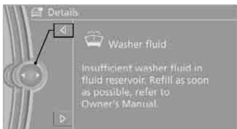
Additional information, e.g. on the cause of a malfunction and on the corresponding need to take action can be displayed via the Check Control, refer to page 82.
