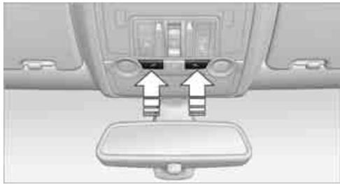
Reading lamps are provided in the front and rear\* adjacent to the interior lamps. Press the button to switch the lamps on and off.
