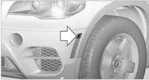
The two camera lenses are located on the sides of the bumper.
