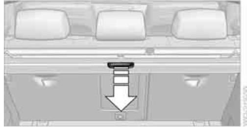
Pull out the luggage compartment roller cover and hook it into the brackets.
