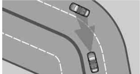
When approaching a curve, the system may react briefly to the vehicles in the next lane due to the bend of the curve. Any deceleration of the vehicle by the system can be compensated for by briefly accelerating. After the accelerator pedal is released, the system becomes active again and independently controls the speed.
