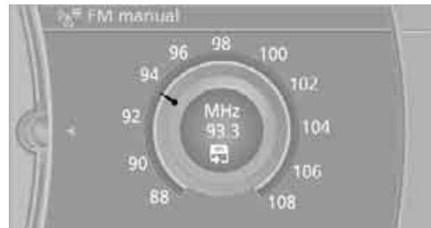
To store the station: press the controller for an extended period.
