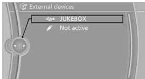
The playback starts with the first track. If an Apple iPhone is connected via the snap-in adapter while an audio device is connected to the AUX-IN connection, the audio signal of the AUX-IN connection will be played.
