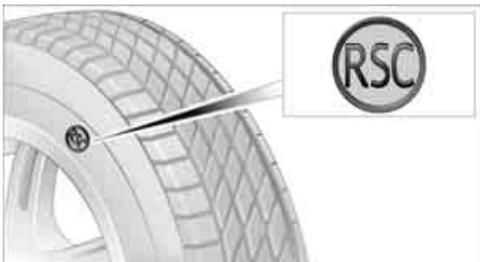
You will recognize run-flat tires by the circular symbol containing the letters RSC on the side of the tire.
