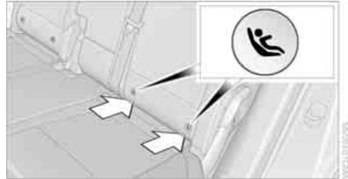
The mounts for the LATCH anchors are located at the points indicated by the arrows.
