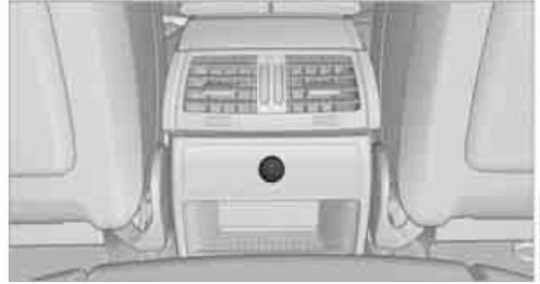
Depending on your vehicle's equipment package, the socket in the rear is covered with a cap or equipped with a lighter. Refer to Cigarette lighter, front, page 130.
