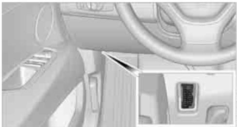
The chief components that make up the emissions content can be checked by a device that uses the OBD socket.
