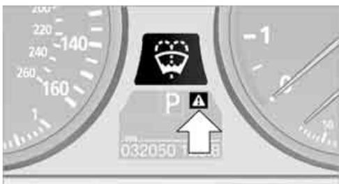
▲ means that a Check Control message has been generated. The symbol continues to be visible even when the Check Control message disappears after a short time. The warning lamps and text messages are stored and can be displayed later, also refer to page 84.
