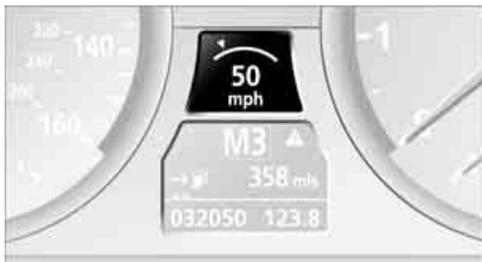
The system stores the current vehicle speed. It is indicated on the speedometer and briefly in the instrument panel.
