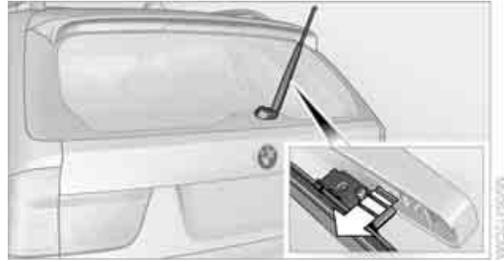
1. Lift off the wiper arm completely and pull off the wiper blade, refer to arrow.
