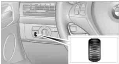
You can control the lighting intensity by using the thumbwheel.
