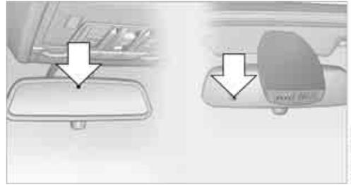
This feature is controlled by two photocells in the interior rearview mirror, one on the front and one on the back.
