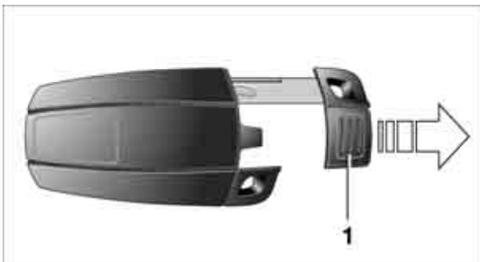
Press button 1 to unlock the key.
