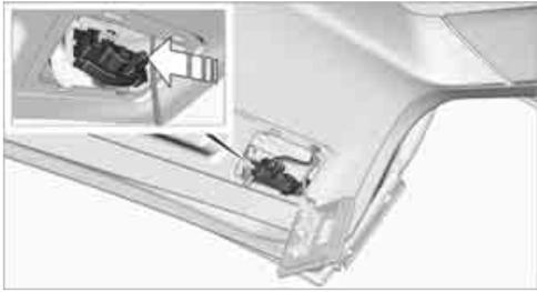
3. Apply gentle pressure to the bulb while turning it to the left for removal and replacement.
