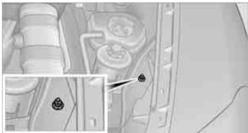
4. Attach the second end of the cable to the negative terminal of the battery or to the engine or body ground of the vehicle to be started.
