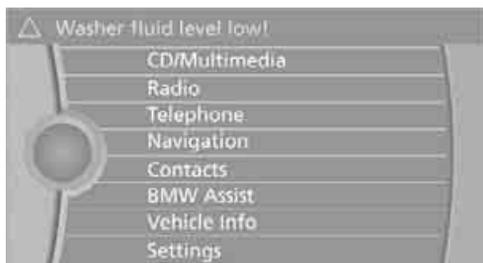
Text messages at the upper edge of the Control Display explain the meaning of the displayed indicator and warning lamps.
