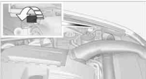
2. Pull the bulb out of the bulb holder and replace.
