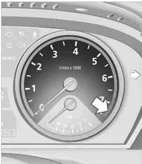
Do not operate the engine with the needle in the red overspeed zone of the gauge, refer to arrow. At high revs in this range, the flow of fuel is interrupted to protect the engine.
