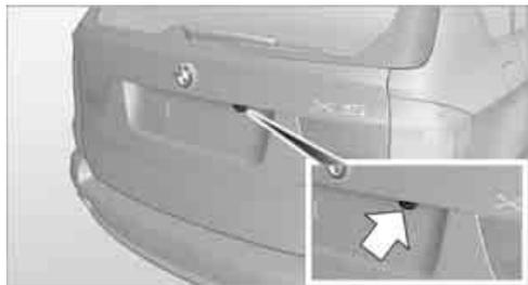
The lens of the rear view camera is under the grasping lip of the liftgate.
