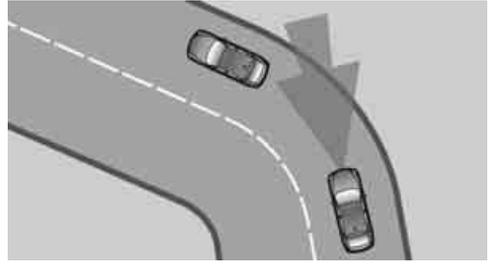
If the desired speed is too high for a curve, the speed is reduced slightly in the curve, although curves cannot be anticipated in advance. Therefore, drive into a curve at an appropriate speed.
