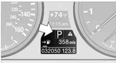
The transmission position is indicated and, in manual mode, the gear currently engaged, e.g. M3.
