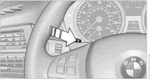
1. With the ignition switched on, press the knob in the instrument panel, refer to page 76, for approx. 5 seconds until the service requirements are displayed.
