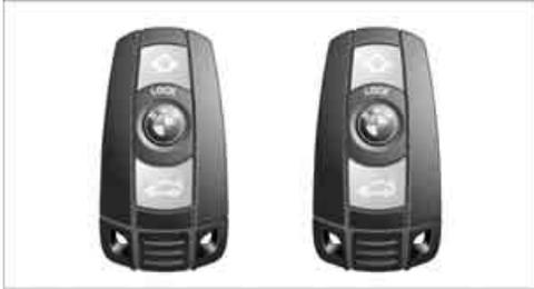
Each remote control contains a battery which is automatically charged in the ignition lock while driving. Drive a longer distance with each remote control at least twice a year to keep the battery charged. For Comfort Access\*, the remote control contains a replaceable battery, refer to page 37.
