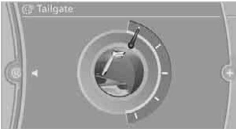
3. Turn the controller until the desired opening height is selected.
