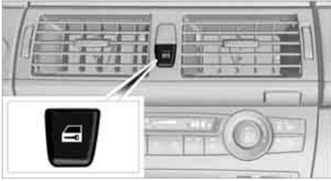
This button serves to unlock or lock doors and the liftgate, with the front doors closed. It does not activate the anti-theft system. The fuel filler flap remains unlocked.
