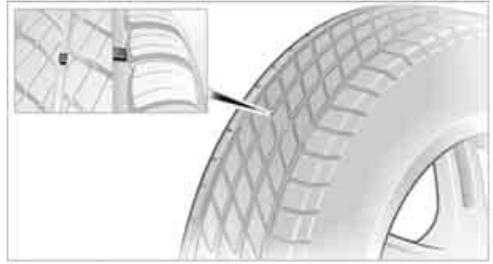
Wear indicators at the tread-groove base are distributed over the tire's circumference and are marked on the side of the tire with TWI – Tread Wear Indicator. If the tire tread has been driven down to the wear indicators, a tread depth of 0.063 in/1.6 mm has been reached.
