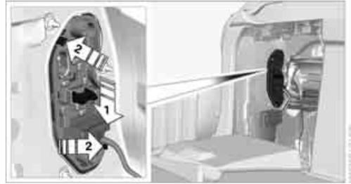
3. Push the button, arrow 1, down, press the catches, arrows 2, outward slightly and remove the bulb holder.
