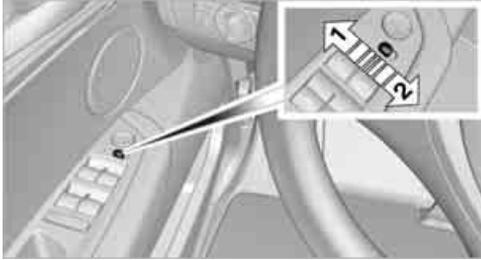
2. Engage transmission position R. The mirror glass tilts downward somewhat on the passenger side. This allows the driver to see the area immediately adjacent to the vehicle – such as a curb – when parking, etc.
