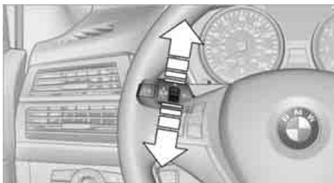
Press the button in the turn signal lever up or down.
