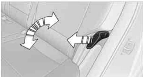
Pull the lever and apply weight to or remove weight from the backrest as needed.
