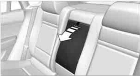
Pull on the loop and fold down the center armrest.
