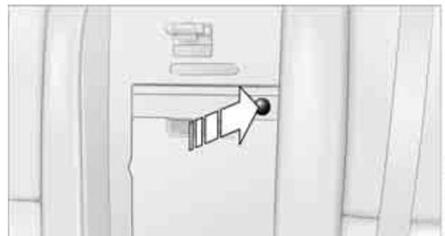
2. Press the button again; the cover in the cargo area opens. If you press the button firmly the first time, this cover also opens.
