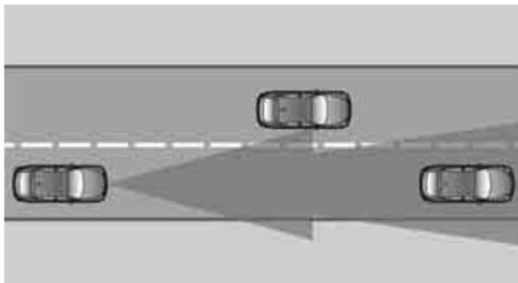
The detection capacity of the system and the automatic braking capacity are limited. For instance, two-wheeled vehicles driving ahead of you might not be detected.
