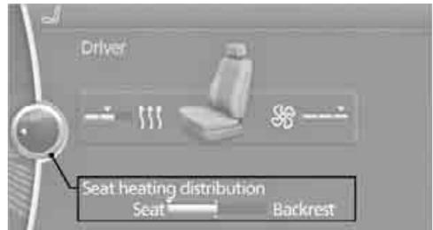
3. Turn the controller to adjust the distribution. The setting is applied.
