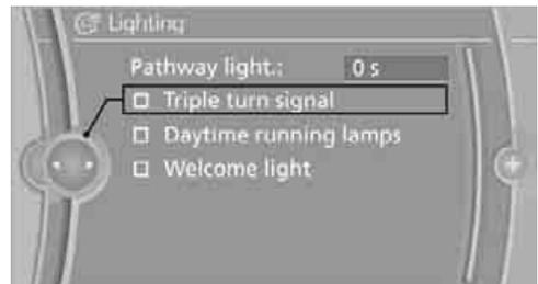
**✓** Triple turn signal activation is activated and is stored for the remote control currently in use.
