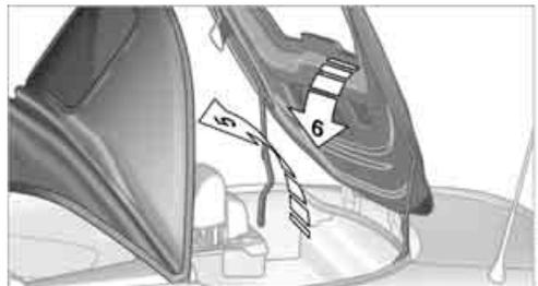
6. Together with another person, press down the front convertible top frame from the outside and on both sides as far as possible.
