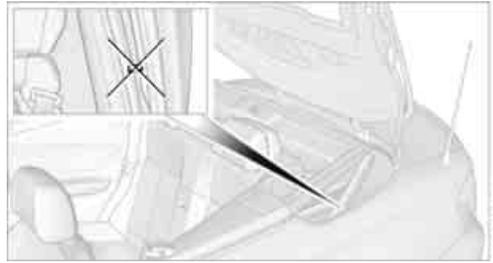
4. Lift out the front part of the convertible top, arrows 4, on both sides and swing it forward. At the same time keep the convertible top box cover from closing, e.g. using your shoulder.
