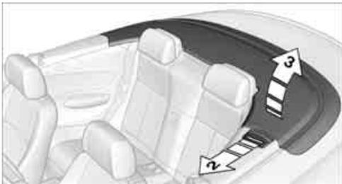
3. The locking pins must have engaged completely. If they are still visible: close the convertible top box cover as far as necessary until the locking bolts engage audibly, then slowly open the cover. During this process, do not close the convertible top box cover completely.
