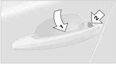
Grasp the handle on the driver's or front passenger door completely, arrow 1. This corresponds to pressing the
