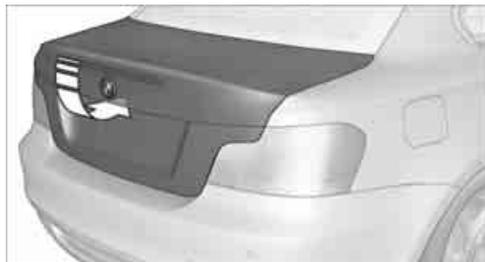
Press the button, see arrow, or the
