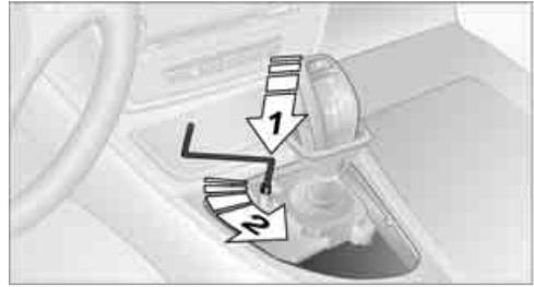
5. Rotate allen wrench until it reaches the stop, arrow 2. The parking lock is unlocked.
