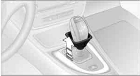
3. Using the allen wrench from the toolkit, refer to page 213, rotate the cover until it reaches the stop, arrow 1, and remove, arrow 2.
