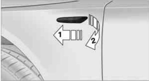
2. While simultaneously lifting the retaining tab, rotate bulb holder to the left and remove.
