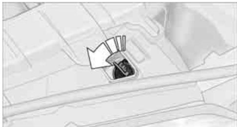
3. Slide the bulb out of the holder and pull off the connector.
