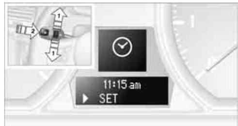
1. Push button **1** in the turn signal/high beam lever up or down repeatedly until the appropriate symbol appears in the display, accompanied by the time and the word "SET".
