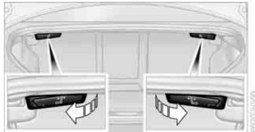
1. To release the rear seat backrest, pull the corresponding lever in the cargo area.
