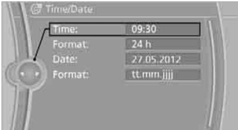
5. Turn the controller to set the hours and press the controller.
