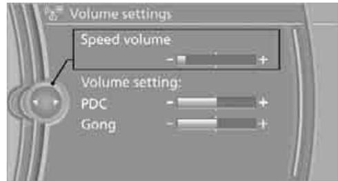
3. Press the controller to confirm the setting.
