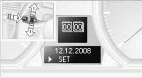
1. Push button **1** in the turn signal/high beam lever up or down repeatedly until the appropriate symbol appears in the display, accompanied by the date and the word "SET".
