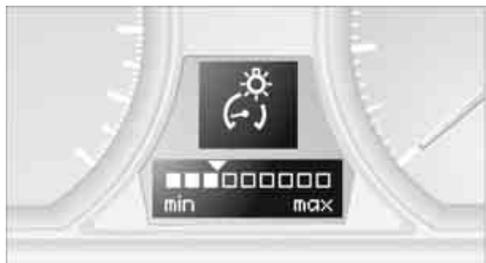
3. Push button **1** up or down to select the desired brightness level.
