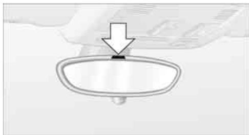
The automatic dimming feature of the interior and exterior mirrors\* is controlled by two photo cells in the interior rearview mirror. One photo cell is in the mirror frame, see arrow; the other is on the back of the mirror.
