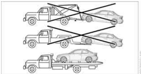
Have the BMW transported with a tow truck with a so-called lift bar, or on a flatbed.
