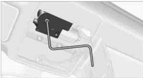
6. Reattach the lamp cover and reinstall the control unit.
