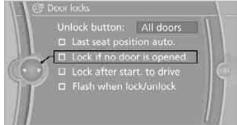
**✔** The function is switched on and is stored for the remote control currently in use.
