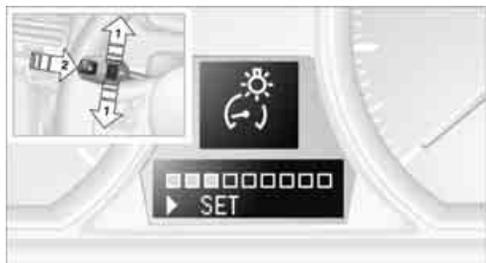
1. Push button **1** in the turn signal/high beam lever up or down repeatedly until the appropriate symbol appears in the display, accompanied by the brightness level and the word "SET".
