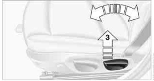
Pull lever **3** and apply your weight to the backrest or lift it off, as necessary.
