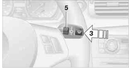
Press the button, arrow **3**. The LED in the button lights up.
