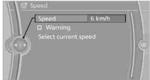
4. Turn the controller until the desired speed is displayed.
