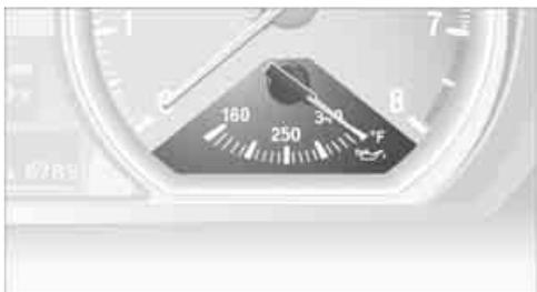
When the engine is at normal operating temperature, the engine oil temperature is between approx. 210 °F/100 °C and approx. 300 °F/150 °C.
