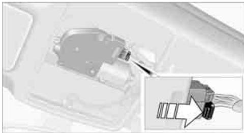
5. Insert the Allen wrench\* supplied with the onboard vehicle tool kit, refer to page 213, into the opening provided. Move the glass roof in the desired direction.
