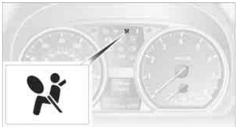
As of radio readiness, refer to page 55, the warning lamp comes on briefly to indicate that the entire airbag system and the belt tensioners are operational.
