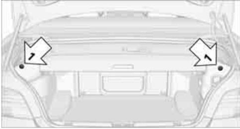
3. If the convertible top is locked, release the two button in the cargo area, arrows 1, using the screwdriver and pull forcefully all the way out. The convertible top box cover is unlocked.
