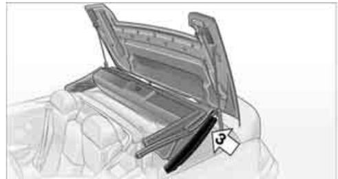
3. Together with the other person, pull the two sides of the convertible top out simultaneously and pivot forward. When doing so, keep the convertible top compartment lid open, arrow **4**, e.g. with your shoulder.
