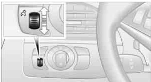
The lighting intensity can be adjusted with the thumbwheel with the parking lamps/low beams switched on.
