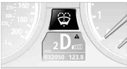
▲ This symbol means that a Check Control message has been generated. The symbol continues to be visible even when the Check Control message disappears after a short time. The warning lamps and text messages are stored and can be displayed later, also refer to page 72.
