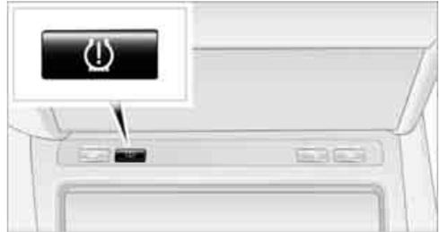
3. Start to drive. The initialization finishes during the trip without providing feedback.
