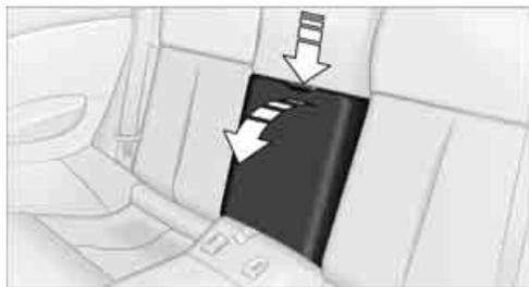
2. Extend the ski bag between the front seats. The zipper facilitates access to the stowed items and drying of the ski bag.
