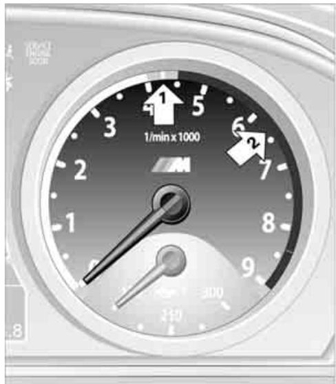
The advance warning field, arrow 1, and the red warning field, arrow 2, change depending on the engine temperature. As the engine temperature rises, the permissible engine speed also increases. Avoid allowing the engine speed to rise as far as the orange warning field whenever possible.
