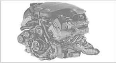
With a 305 cu in/5 liter displacement, the high-speed V10 engine generates a maximum output of 373 kW and a maximum torque of 383 lb ft/520 Nm. Its spontaneous response characteristics yield a very broad usable engine speed range. At the maximum engine speed of 8,250 rpm, the flow of fuel is interrupted in order to protect the engine. Due to the powerful engine dynamics, when the vehicle is at rest, the maximum engine speed is limited to 7,000 rpm.
