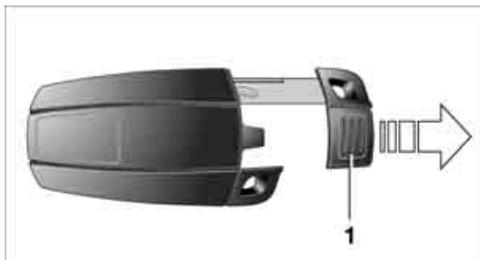
Press button 1 to unlock the key.
