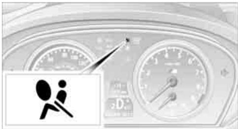
From radio readiness, refer to page 55, the warning lamp lights up briefly, indicating the operational readiness of the entire airbag system and the safety belt tensioners.
