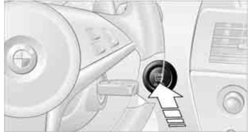
Pressing the Start/Stop button switches the radio readiness or the ignition on and off.
