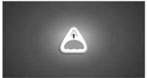
Pull the lever in the cargo area. The luggage compartment lid is unlocked.
