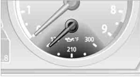
The general operating temperature lies between 175 °F/80 °C and 250 °F/120 °C. Do not exceed a value of approx. 265 °F/130 °C. If the engine oil temperature is too high, the permissible engine speed, and with it the available engine output is reduced.
