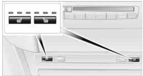
The temperature setting advances one step in its control sequence each time you press the button. The highest temperature is set when three LEDs are lit.
