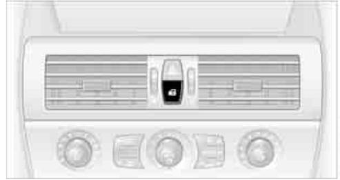
This button serves to unlock or lock doors and the luggage compartment lid, but does not activate the anti-theft system. The fuel filler flap remains unlocked.
