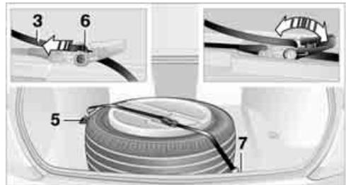
5. Completely open the tensioning lock.
