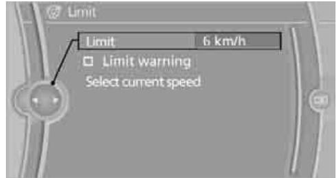
4. Turn the controller until the desired limit is displayed.
