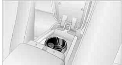
The compartment of the rear center console contains a built-in cupholder and a removable one.
