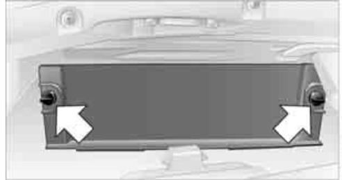
Open the cover in the glove compartment and remove it.
