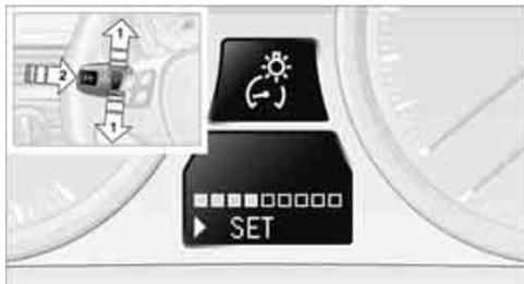
1. Push button **1** up or down repeatedly until the appropriate symbol appears in the display, accompanied by the brightness setting and scale the word "SET".
