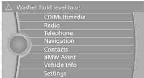
Text messages at the top edge of the Control Display describe the meanings of the indicator and warning lamps.
