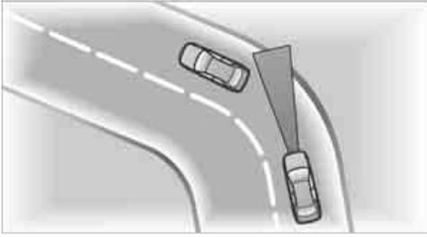
Because of the limited range of the system, it is possible that in curves or on the peaks and valleys of hilly roads, a vehicle ahead may be recognized late, or not at all. Therefore, it is up to the driver to select a speed that is prudent in view of the curves and terrain of the roadway.
