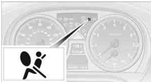
As of radio readiness, refer to page 54, the warning lamp comes on briefly to indicate that the entire airbag system and the belt tensioners are operational.
