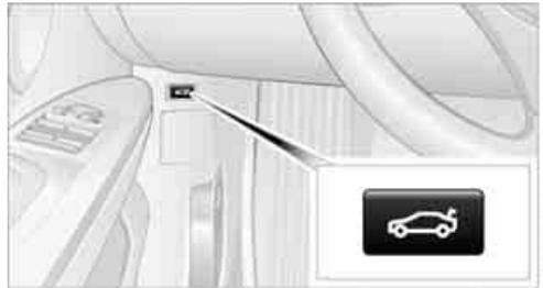
Press the button: the trunk lid/tailgate opens unless it has been locked.
