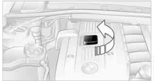
Add a maximum of 1 US quart/1 liter of engine oil no earlier than when a corresponding message appears on the Control Display or, if the car has a diesel engine, when the oil level has dropped to just above the lower marking on the dipstick, refer to page 219.
