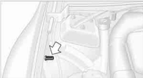
5. Attach the second terminal clamp of the minus/- jumper cable to the negative termi-
