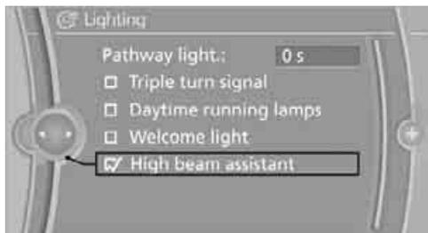
**✓** The high-beam assistant is activated and is stored for the remote control currently in use.
