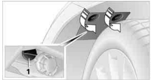
2. Rotate turn signal bulb socket 1 to the left and remove.
