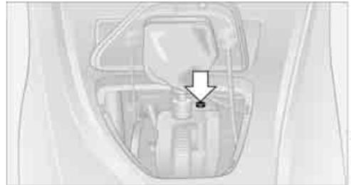
3. Using the screwdriver from the onboard vehicle tool kit, refer to page 229, press the red lever while moving the selector lever to the desired position.
