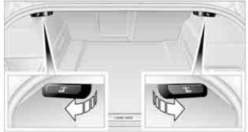
5. The unlocked rear seat backrest moves forward slightly. Fold the backrest forward by the head restraint.
