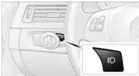
**⚠** The parking lamps or low beams must be switched on for the fog lamps to operate. The green indicator lamp in the instrument cluster lights up whenever the fog lamps are on.
