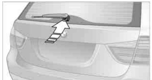
Press the button: the rear window opens slightly. It can now be swung upwards.
