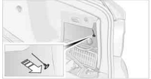
1. Remove the cover from the right-hand side wall of the cargo area.
