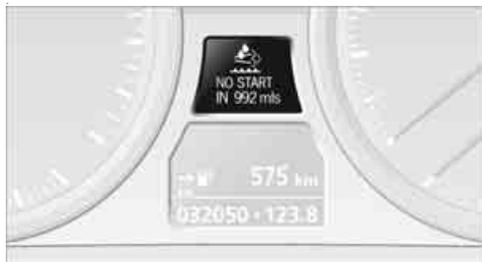
After refilling, the reserve display continues to be displayed after the engine is started. It goes out after the vehicle has been driven for several minutes.
