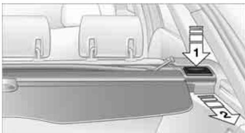
3. Pull the casing out backwards, arrow 2, without tilting it.
