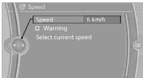
4. Turn the controller until the desired speed is displayed.
