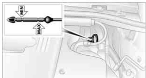
The oil quantity between the two markings on the dipstick is equivalent to approx. 1 US quart/ 1 liter.
