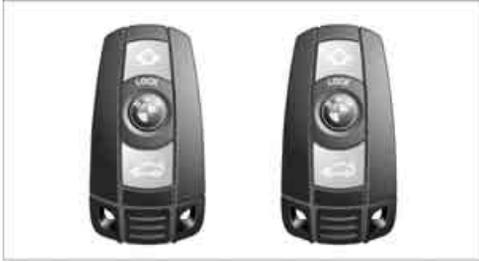
Each remote control contains a rechargeable battery that is automatically recharged when it is in the ignition lock while the car is being driven. Use each remote control at least twice a year for longer road trips in order to maintain the batteries' charge status. In cars with Comfort Access\*, the remote control contains a replaceable battery, refer to page 35.
