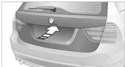
Press the button, see arrow, or the
