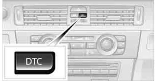
Press the button for at least 3 seconds; the indicator lamps for DSC in the instrument cluster light up. Dynamic Traction Control DTC and DSC have been simultaneously deactivated. Stabilizing and drive-output promoting actions are no longer executed.
