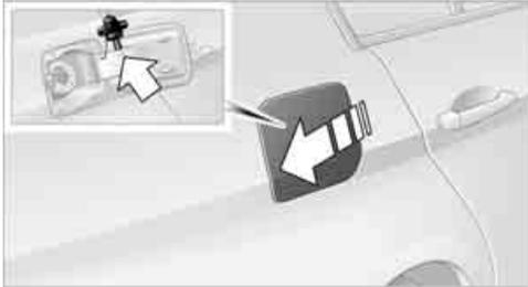
1. Open the fuel filler flap. To do so, lightly press the rear edge.
