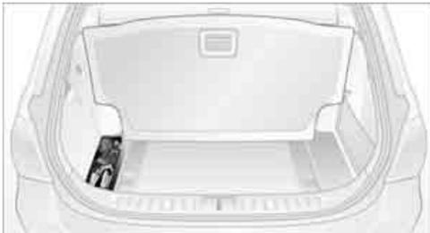
The onboard vehicle tool kit is stored in a compartment on the left-hand side underneath the cargo area floor panel.
