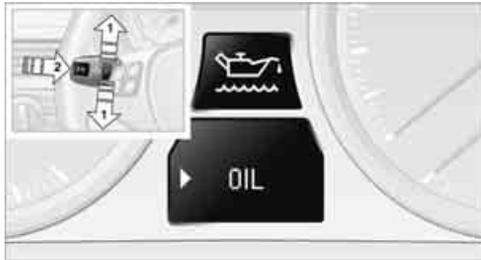
1. Push button **1** in the turn indicator lever up or down repeatedly until the appropriate symbol is shown in the display, accompanied by the word "OIL".
