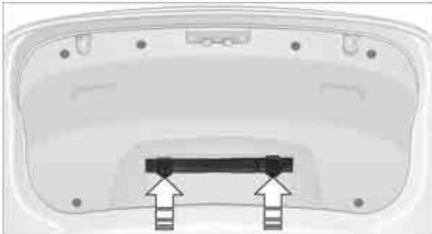
The warning triangle is located in a holder in the trunk lid. Press the tabs to take it out.
