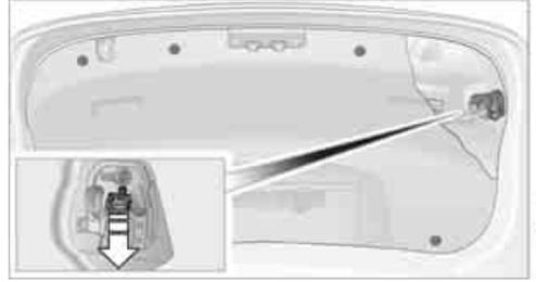
1. Take the warning triangle out of its holder, refer to page 238. Unscrew the holder using the screwdriver from the onboard vehicle tool kit.
