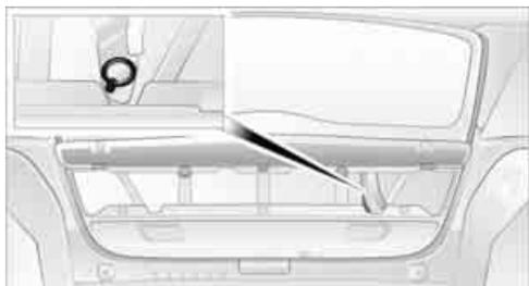
3. Open the tailgate and close the cover again. The tailgate is locked as soon as it is pressed shut.
