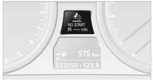
Even if the display indicates -- mls, the engine continues running if it is not switched off and if all other requirements continue to be met, e.g. a sufficient supply of fuel.
