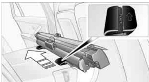
4. Slide the casing into the guides on the backs of the seat backrests.
