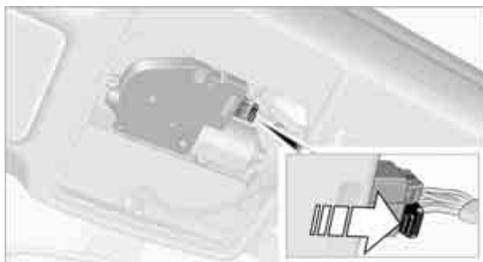
5. Insert the Allen wrench\* supplied with the onboard vehicle tool kit, refer to page 229, into the opening provided. Move the glass roof in the desired direction.
