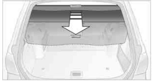
Press the button: the roller cover is raised.
