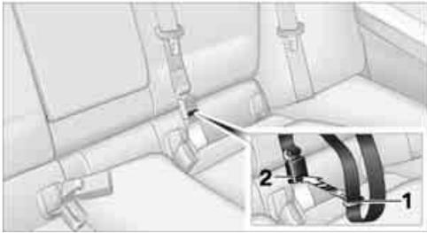
2. Insert the latch plate at the end of the belt into the specially designated fixture on the rear window shelf.
