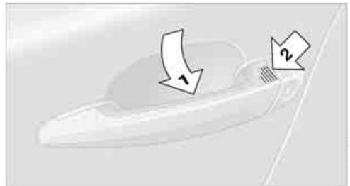
Grasp the handle on the driver's or front passenger door completely, arrow 1. This corresponds to pressing the
