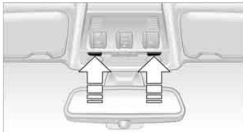
There are reading lamps at the front and rear\*, next to the interior lamps. To switch on and off, press the button.
