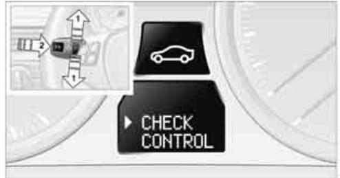
1. Push button 1 in the turn indicator lever up or down repeatedly until the appropriate symbol appears in the display, accompanied by the words "CHECK CONTROL".
