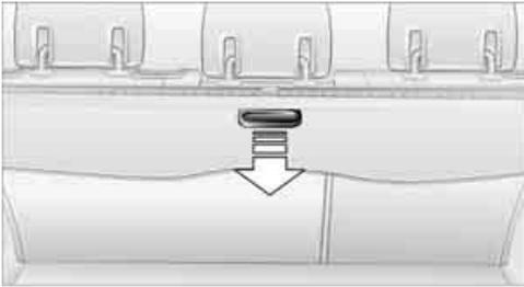
Pull out the cover and hook it into the retaining fixtures.
