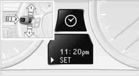
1. Push button **1** in the turn indicator lever up or down repeatedly until the appropriate symbol appears in the display, accompanied by the time and the word "SET".
