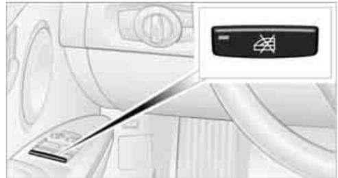
With the safety switch, you can prevent the rear windows from being opened or closed via the switches in the rear passenger area, by children, for example. When the safety function is switched on, the LED comes on.
