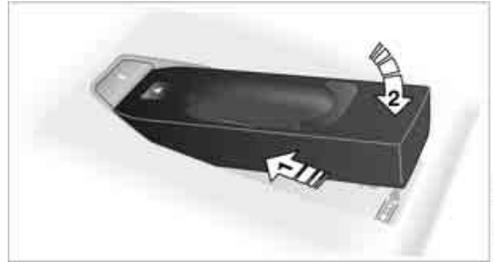
To remove the snap-in adapter:
