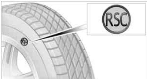
The symbol identifying run-flat tires is a circle with the letters RSC on the sidewall. Run-flat tires comprise a conditionally self-supporting tire and a special rim. The reinforcement in the sidewalls ensures that the tire can continue to be used subject to certain restrictions, even if depressurized.
