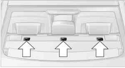
There are three additional anchors for child restraint systems with tether straps, see arrows.
