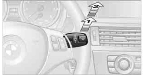
**1** Intermittent operation. When reverse gear is engaged, the system switches to continuous operation.
