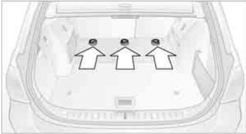
There are three additional anchors under a cover for child restraint systems with tether straps, see arrows.
