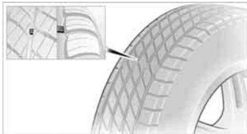
Wear indicators in the base of the tread groove are distributed around the tire's circumference; the letters TWI, for Tread Wear Indicator, on the tire's sidewalls identify tires that incorporate these wear indicators. Once the tire tread has worn down to the wear indicators, the tire has worn to a depth of 1/16 in/1.6 mm.
