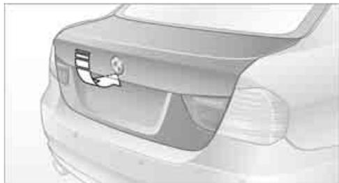
Press the button, see arrow, or the
