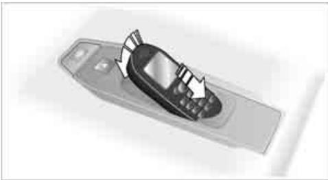
From radio readiness or with the steering unlocked the mobile phone's battery is charged.
