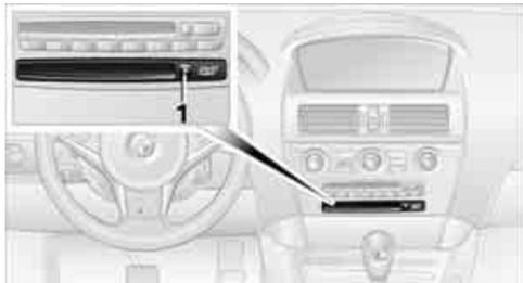
1. Insert the navigation DVD with the labeled side up. The navigation DVD is pulled in automatically.
