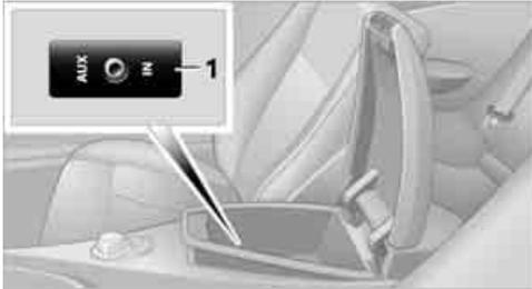
For audio playback via the vehicle loudspeakers, connect the headphones or the line-out connection of the device to the socket **1** with a 1/8 in/3,5 mm jack plug.
