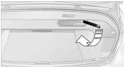
With the convertible top closed, you can increase the luggage compartment capacity: To do so, unfold the handle and press it downward in the direction of travel, refer to arrow. This moves the convertible top compartment floor into the raised position.
