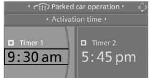
7. Turn the controller to make the adjustment.
