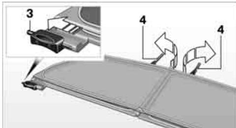
4. Unfold the rear mounts 4.
