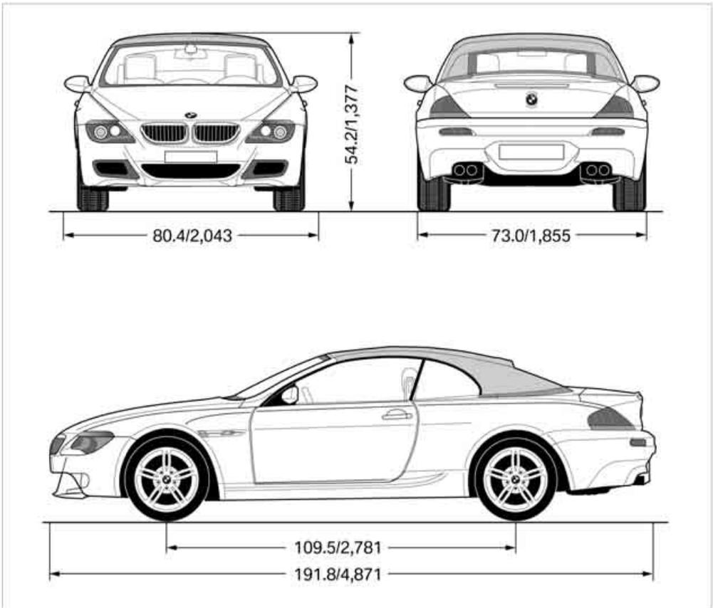
All dimensions given in inches/mm. Smallest turning circle diam.: 41 ft/12.5 m
