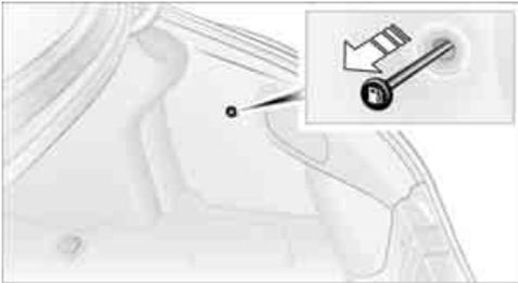
In the event of an electrical malfunction, you can release the fuel filler door manually:
