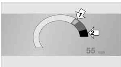
To achieve the best vehicle acceleration with a sporty driving style, shift lights in the Head-Up Display\* indicate the optimum shifting point briefly before reaching the maximum rpm. Refer to Shift lights, page 64.
