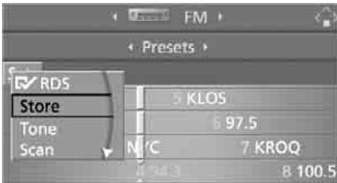
5. Turn the controller until the desired memory position is selected. The number of the memory position appears beside the name or frequency of the station.
