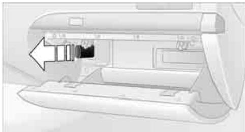
**!** Be sure that the flashlight is switched off when it is inserted into its socket. Failure to comply with this precaution could lead to overcharging and damage. ◀
