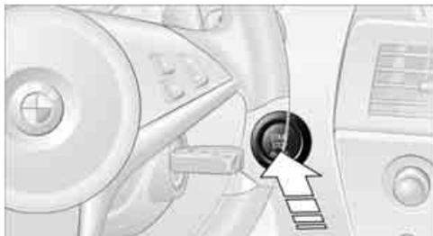
Pressing the Start/Stop button switches the radio readiness or the ignition on and off.
