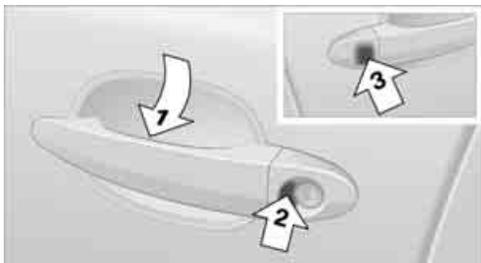
Grasp a door handle fully, refer to arrow 1, but do not touch the surfaces, arrow 2 or 3 when doing so. This corresponds to pressing the button.
