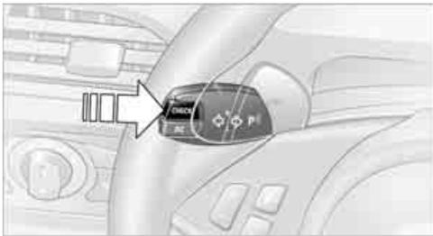
Press the CHECK button in the turn signal lever. Some Check Control messages are displayed until the malfunctions have been rectified. They cannot be hidden. If a number of these malfunctions occur simultaneously, they are displayed in succession.
