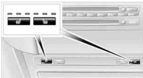
The temperature setting advances one step in its control sequence each time you press the button. The maximum temperature is supplied when three LEDs are lit.
