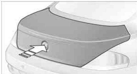
Press the upper half of the BMW emblem or press the
