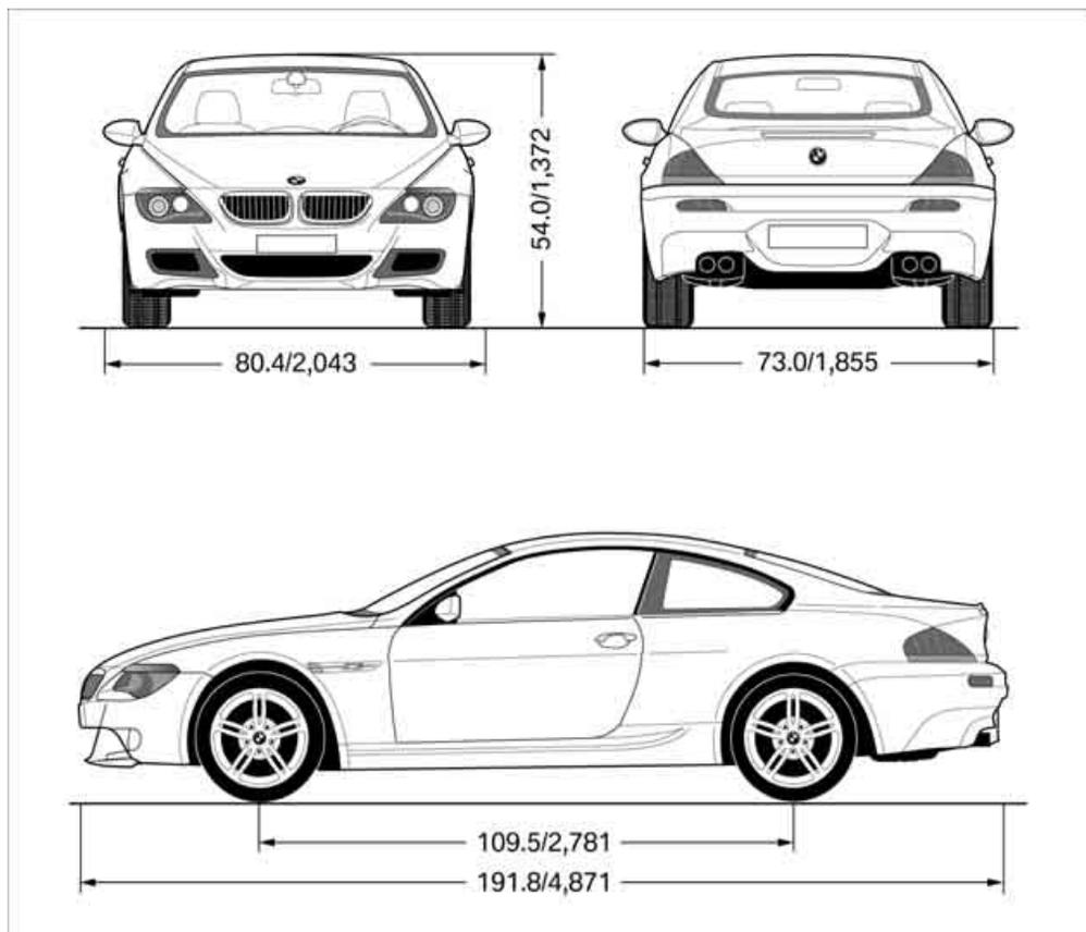
All dimensions given in inches/mm. Smallest turning circle diam.: 41.0 ft/12.5 m
