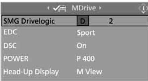
5. Turn the controller to set Drive mode or Sequential mode.
