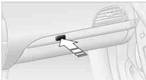
Press the button. The glove compartment opens automatically and the lamps come on.
