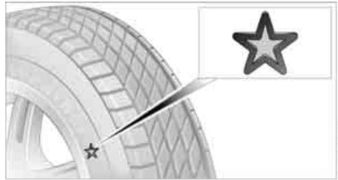
BMW recommends particular tire brands for each tire size. You can recognize these from the clearly visible BMW marking on the tire sidewall. With proper use, these tires meet the highest standards for safety and handling characteristics.
