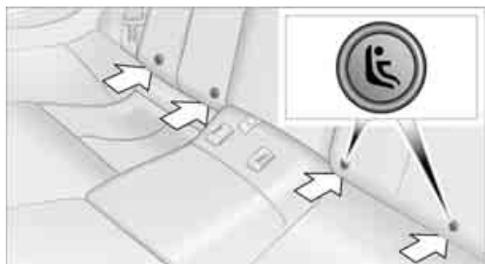
The mounting points for the LATCH anchors are located at the positions indicated by arrows in the gap between the seat and the backrest.
