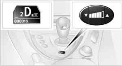
Press the button repeatedly until the desired driving program is displayed in the instrument cluster, refer to page. 63
