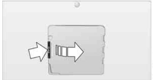
4. Open the loading flap and use the magnetic holder to secure it to the rear panel.
