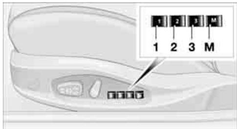
You can store and select three different adjustment settings for the driver's seat, exterior mirrors and steering wheel.
