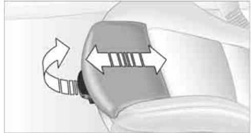
You can also adjust the thigh support manually: Pull the lever and adjust the thigh support in the longitudinal direction.
