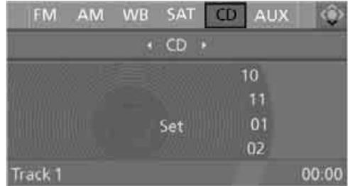
4. With a CD changer, change to the second field from the top and turn the controller until "CD" is selected and press the controller.
