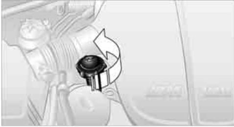
Do not add oil until a value slightly above the minimum of 0.0 US quarts/liters is displayed by the oil level measurement. In this area a message is also shown on the Control Display.
