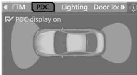
6. Select "PDC display on" and press the controller.
