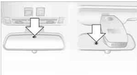
This feature is controlled by two photocells in the inside rearview mirror. One is integrated within the mirror's lens, while the other is located at an offset position on the rear of the mirror housing.
