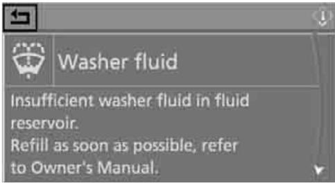
You can display supplementary information regarding most Check Control messages, e.g. as to the cause of a malfunction and corresponding actions to be taken, see below.
