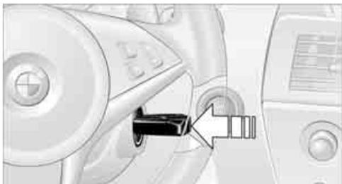
Insert the remote control as far as possible into the ignition lock.
