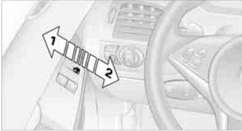
2. Shift into reverse or move selector lever into position R. The mirror glass tilts downward somewhat on the passenger's side. This allows the driver to see the area immediately adjacent to the vehicle – such as a curb – when parking, etc.
