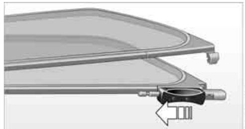
1. Push the handle of the securing pin on the wind deflector on the left side of the vehicle all the way back and release the locking mechanism.
