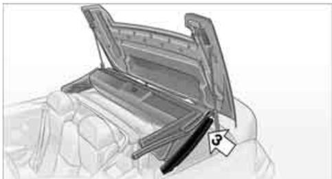
3. Together with the other person, pull the two sides of the convertible top out simultaneously and pivot forward. When doing so, keep the convertible top compartment lid open, arrow 4, e.g. with your shoulder.
