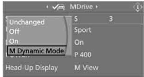
"Unchanged" retains the current setting made outside of MDrive.
