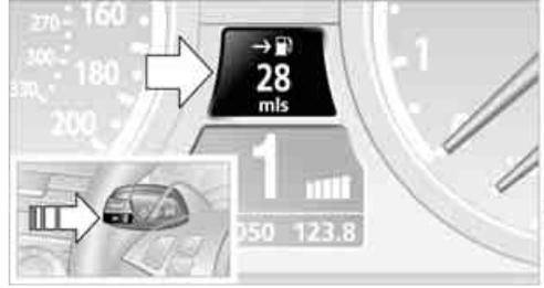
Press the button on the turn signal lever.
