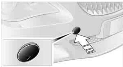
Rear: press the arrow symbol on the cover while prying out the cover upward by hand.
