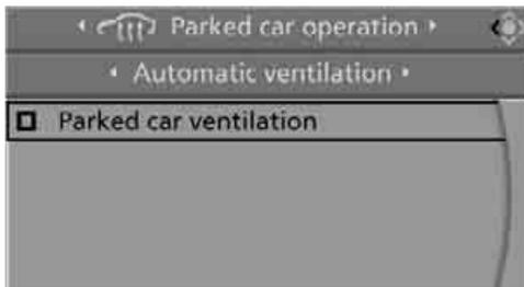
The parked car ventilation is switched on. The
