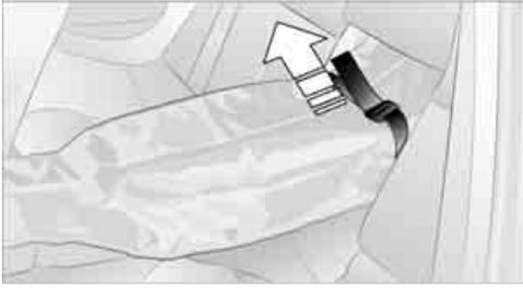
After loading, secure the ski bag and its contents. To do so, tighten the retaining belt at the buckle.
