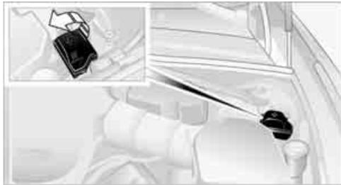
2. Attach one end of the jumper cable plus/+ to the positive terminal of the battery or a jump-starting terminal of the vehicle providing assistance.
