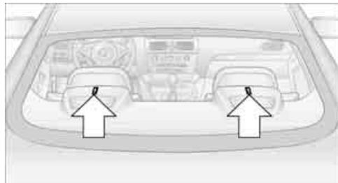
There are two additional mounting points for child restraint systems with a tether strap, refer to arrows.
