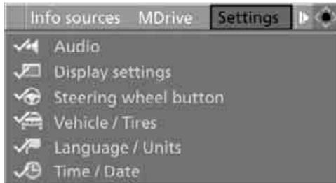
3. Turn the controller until "Settings" is selected and press the controller.
