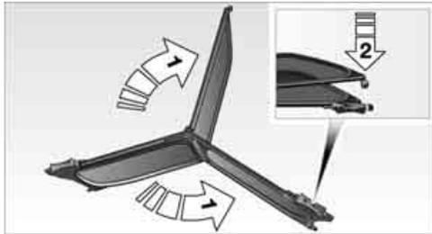
2. Press the upper and lower section together until the locking device engages, refer to arrow 2.
