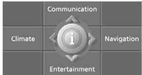
2. Move the controller forward to open "Communication".
