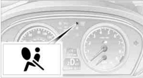
From radio readiness, refer to page 59, the warning lamp lights up briefly, indicating the operational readiness of the entire airbag system and the safety belt tensioners.
