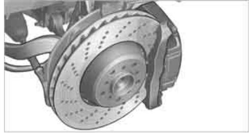
Your BMW M6 has a high-performance brake system with perforated compound brake rotors. Due to the special structural features of these brake rotors, function noises occur during braking, but this has no effect on the performance, operating safety, and stability of the brakes.
