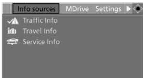
4. Turn the controller until "Service" is selected and press the controller.
