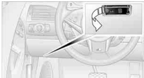
Components which are decisive for the exhaust-gas composition can be checked via the OBD socket with a device.
