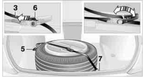
5. Completely open the tensioning lock.
