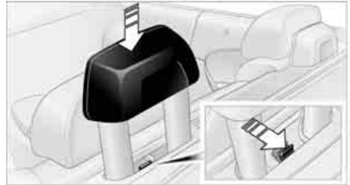
2. Press the rollover protection unit halfway down from above.
