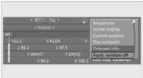
To switch on, change to the assistance window and press the controller.
