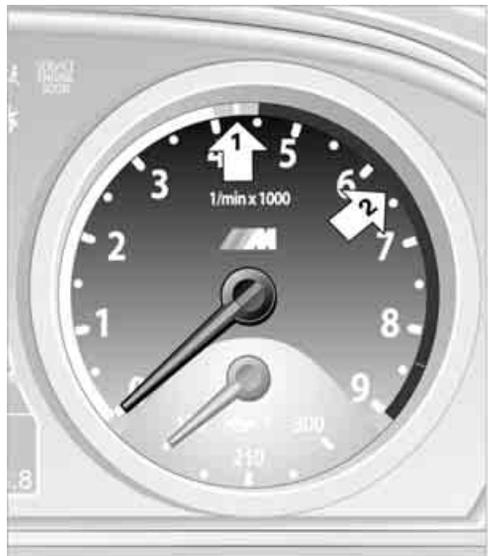
The advance warning field, arrow 1, and the red warning field, arrow 2, change depending on the engine temperature. As the engine temperature rises, the permissible engine speed also increases. Avoid allowing the engine speed to rise as far as the advance warning field whenever possible.
