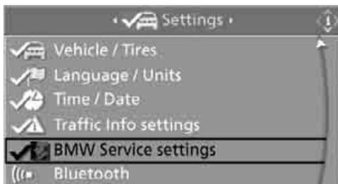
5. Change to upper field if necessary. Turn the controller until "Service Status" is selected and press the controller. The currently available BMW Assist services are displayed.
