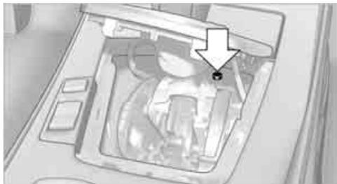
3. Using the screwdriver from the onboard tool kit, refer to page 208, press the red lever while moving the selector lever to the desired position.
