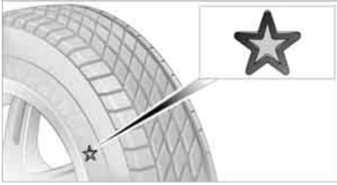
Certain makes of tire are recommended by BMW for each tire size. They are marked with a clearly visible BMW designation on the sidewall of the tire.
