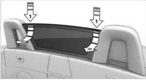
**⚠** The wind deflector must engage firmly, otherwise it could become detached at higher vehicle speeds. ◀
