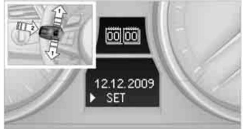
1. Press button **1** in the turn indicator lever up or down repeatedly until the appropriate symbol appears in the display, accompanied by the date and the word "SET".
