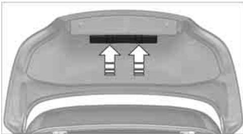
The warning triangle is located in a holder in the luggage compartment lid. Press the tabs to take it out.
