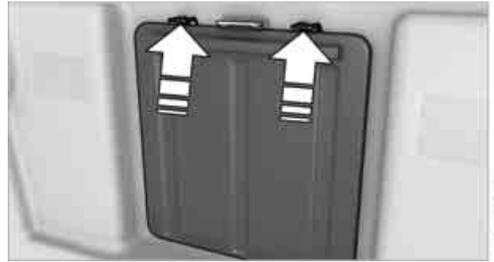
In the cargo bay: Press the handle up and fold the transport bag completely down.
