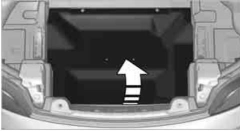
The onboard tool kit is located in the cargo bay under the floor panel.
