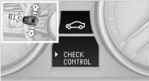
1. Press button **1** in the turn indicator lever up or down repeatedly until the appropriate symbol appears in the display, accompanied by the words "CHECK CONTROL".
