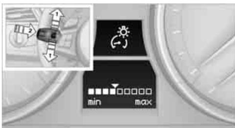
3. Press button 1 up or down to select the desired brightness level.
