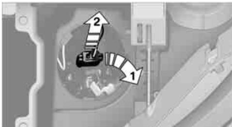
4. Disconnect the plug, change the bulb and reconnect the plug.
