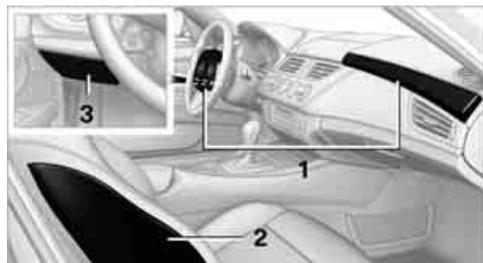
The following airbags are located under the marked covers:
