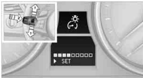
1. Press button 1 up or down repeatedly until the appropriate symbol appears in the display, accompanied by the brightness setting and scale the word "SET".
