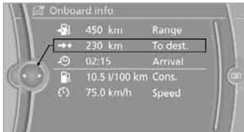
4. Turn the controller until the desired distance is displayed.
