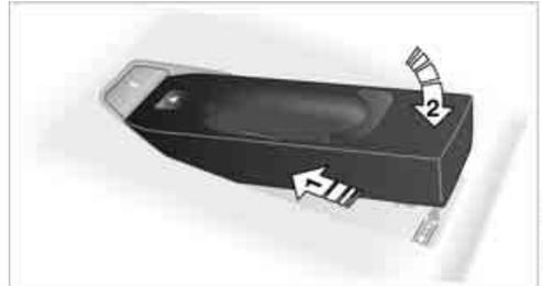
To remove the snap-in adapter:
