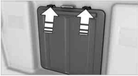
In the cargo bay: Press the handle up and fold the storage compartment completely down.
