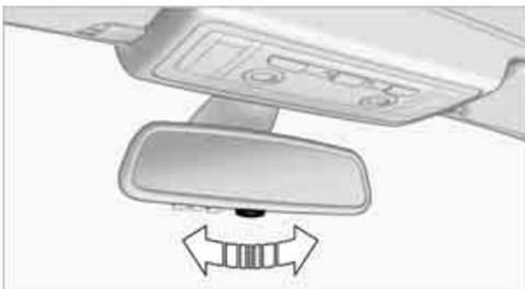
Turn the knob to reduce glare from the headlights of cars behind you when driving at night.
