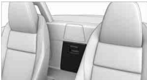
2. In the cargo bay: press the tab up and fold the cover down.
