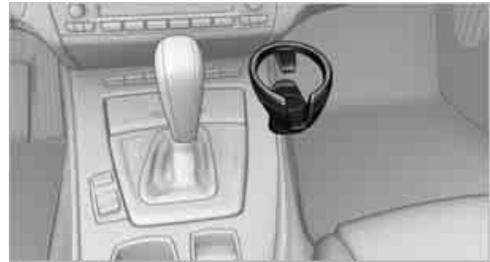
Mount the cup holder onto the center console so that it snaps into place.
