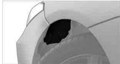
2. Turn both locks in the wheel house to the left and remove the cover.
