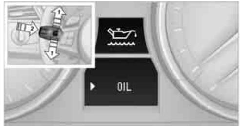
1. Press button 1 in the turn indicator lever up or down repeatedly until the appropriate symbol is shown in the display, accompanied by the word "OIL".
