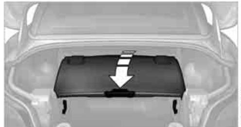
Before opening the hardtop, close the cargo bay partition, arrow, and make sure it engages on both sides.
