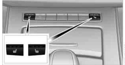
Press once for each temperature level. Three LEDs indicate the highest temperature.
