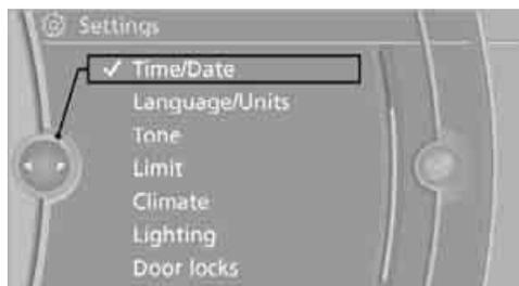
4. Turn the controller until "Time:" is highlighted, and then press the controller.
