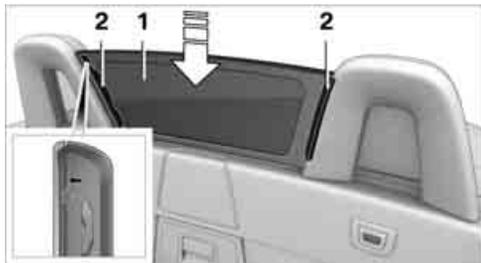
2. Push the wind deflector down, arrow 1, and then push down and forward simultaneously, arrow 2, until it engages.
