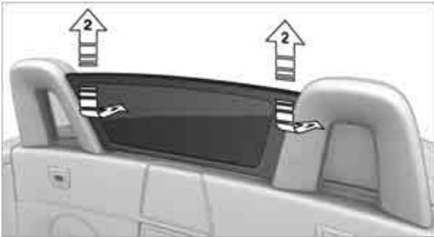
2. Pull the wind deflector upward out of the holders, arrow 2.
