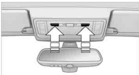
The reading lamps are located next to the interior lamps. To switch on and off, press the button.
