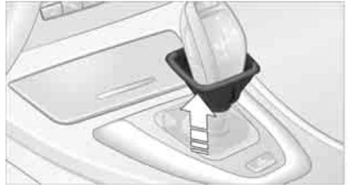
3. Remove the cap using the Allen wrench from the onboard tool kit, refer to page 208.
