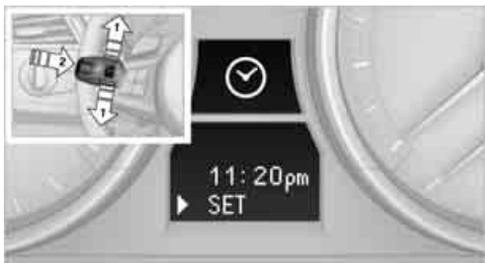
1. Press button 1 in the turn indicator lever up or down repeatedly until the appropriate symbol appears in the display, accompanied by the time and the word "SET".
