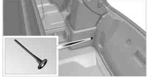
Pull the button in the cargo bay with the fuel pump symbol down. The fuel filler door is released.
