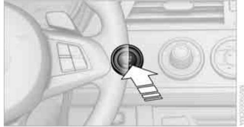
Pressing the start/stop button switches radio readiness or the ignition on or off.
