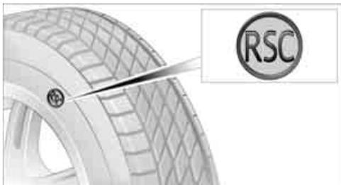
The symbol identifying Run-Flat Tires is a circle with the letters RSC on the sidewall.
