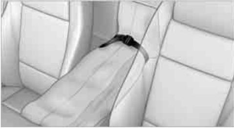
After loading, secure the transport bag and its contents. Tighten the retaining strap on the tensioning buckle for this purpose.
