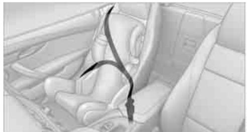
The safety belt for the passenger can be locked to prevent it from being pulled out when it is used to secure child-restraint systems.
