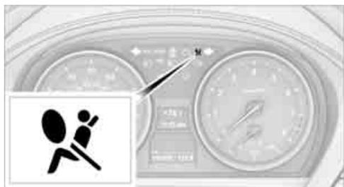
As of radio readiness, refer to page 50, the warning lamp comes on briefly to indicate that the entire airbag system and the belt tensioners are operational.
