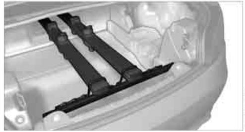
**⚠** Before closing the cargo bay, ensure that the luggage compartment lid cannot be damaged by the skis. ◀
