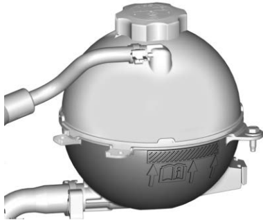
3.6L V6 Engine Coolant Surge Tank
