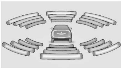
The instrument cluster may have a Park Assist display with bars that show “distance to object” and object location information for the Park Assist system. As the object gets closer, more bars light up and the bars change color from yellow to amber to red.
