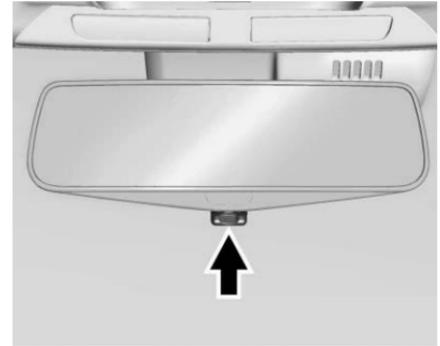
Pull the tab rearward to turn on the display. Push the tab forward to turn it off. When off, the mirror is automatic dimming. Adjust the mirror for a clear view of the area behind the vehicle while the display is off.
