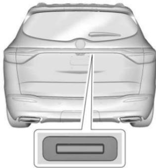
To open the liftgate, press the touch pad under the liftgate handle and lift up.
