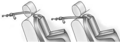
If the position you are using has a fixed head restraint and you are using a single tether, route the tether under the head restraint and in between the head restraint posts or around the outboard side of the head restraint.
