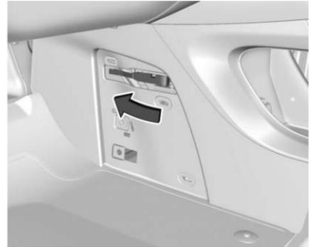
2. Rotate the manual park release lever 90° back to its original position.
