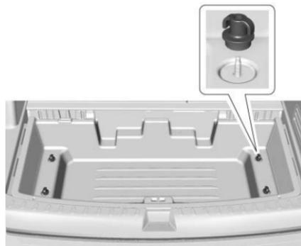
2. Remove the four wing nuts.
