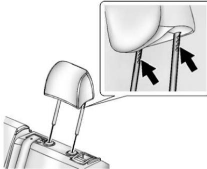
1. Insert the head restraint posts into the holes in the top of the seatback. The notches on the posts must face the driver side of the vehicle.
