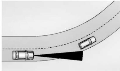
When following a vehicle and entering a curve, ACC may not detect the vehicle ahead and accelerate to the set speed. When this happens, the vehicle ahead indicator will not appear.
