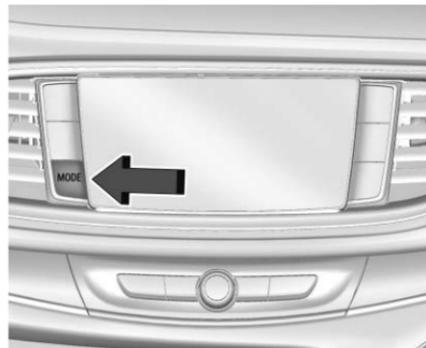
To select the Sport Mode or Tow/Haul Mode, press the MODE switch on the center stack. Pressing the MODE switch will display options of all available ride modes in the DIC and change to the next mode. Subsequent presses will scroll through the available modes.
