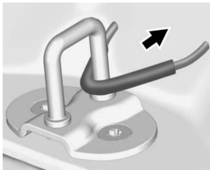
8. Make sure the metal tube is centered at the striker. Push the tube toward the front of the vehicle.
