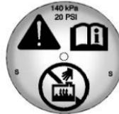
1. Remove the coolant surge tank pressure cap when the cooling system, including the coolant surge tank pressure cap and upper radiator hose, is no longer hot.
