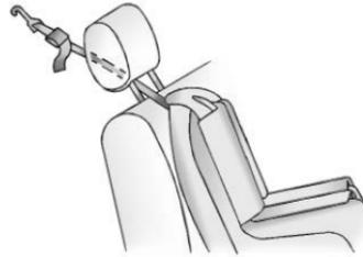
If the position you are using has an adjustable head restraint and you are using a single tether, raise the head restraint
