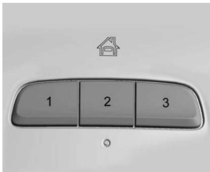
If equipped, the Universal Remote System allows for garage door openers, security systems, and home automation devices to be programmed to work with these buttons in the vehicle.
