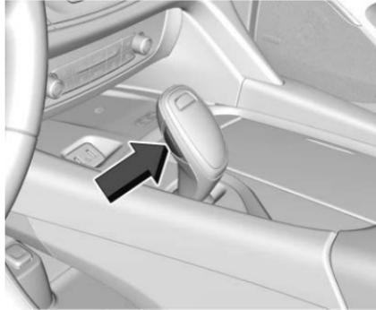
1. With your foot on the brake pedal, press and hold the shift lock release button.
