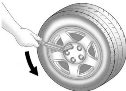
2. Turn the wheel wrench counterclockwise to loosen all the wheel nuts, but do not remove them yet.
