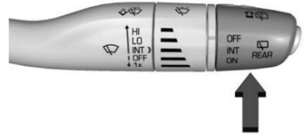
The rear window wiper/washer controls are on the end of the windshield wiper lever.
