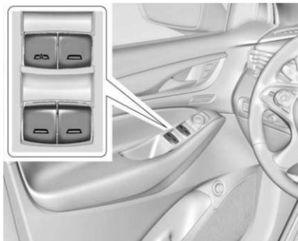
The power windows work when the ignition is on, in ACC/ACCESSORY, or when Retained Accessory Power (RAP) is active. See *Retained Accessory Power (RAP)* ⇨ 203.
