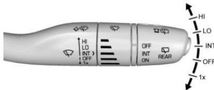
With the ignition on or in ACC/ACCESSORY, move the windshield wiper lever to select the wiper speed.
