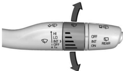
**INT** : Move the windshield wiper lever to INT. Turn the band up for more frequent wipes or down for less frequent wipes.
