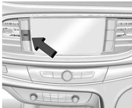
AWD Mode is intended for conditions which demand more traction. In AWD Mode, the AWD system delivers power to all four wheels and the system adjusts as needed to improve traction. Pressing the AWD Mode switch will select AWD Mode. The AWD light will flash briefly while the system is
