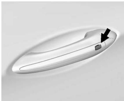
Press the button on the driver door handle when the RKE transmitter is within 1 m (3 ft) of the driver door handle. When unlocking from the driver door, the first press unlocks that door; press again within five seconds to unlock all passenger doors. See *Remote Keyless Entry (RKE) System Operation* ⇨ 29.
