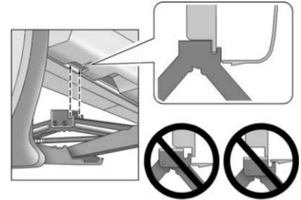
5. Turn the wheel wrench clockwise to raise the jack lift head until the slots in the jack head fit into the metal flange behind the cut out on the plastic molding. Do not raise the vehicle yet.
