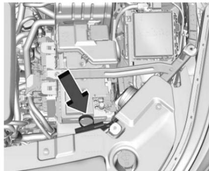
2. Open the hood and unwrap the electrical cord. The bundled cord is on the driver side of the engine compartment, in front of the battery. See *Engine Compartment Overview* ⇨ 267.
