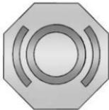
The brake master cylinder reservoir is filled with GM approved DOT 3 brake fluid as indicated on the reservoir cap. See *Engine Compartment Overview* ⇨ 267 for the location of the reservoir.
