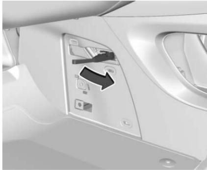
6. Pull the manual park release lever 90° to its latching position.
