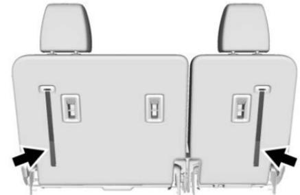
6. Pull the release strap located on the seatback.
