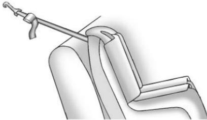
If the position you are using does not have a head restraint and you are using a single tether, route the tether over the seatback.
