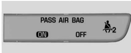
The words ON and OFF will be visible during the system check. When the system check is complete, either the word ON or OFF will be visible. See *Passenger Airbag Status Indicator* ⇨ 137.
