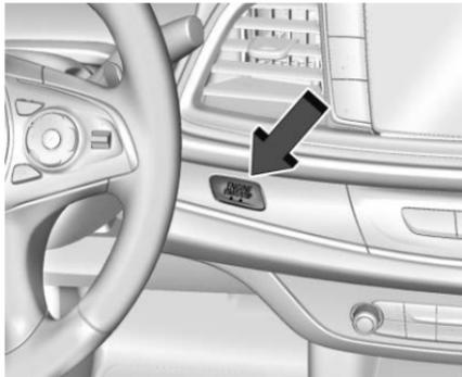
Vehicles with Keyless Access have pushbutton starting.
