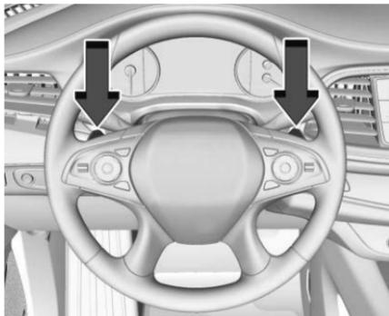
Electronic Range Select (ERS) or Manual Mode allows for the selection of the range of gear positions. Use this mode when driving downhill to limit the top gear and vehicle speed.
