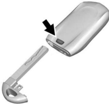
To remove the key, press the button on the bottom of the RKE transmitter and pull the key out. Never pull the key out without pressing the button.
