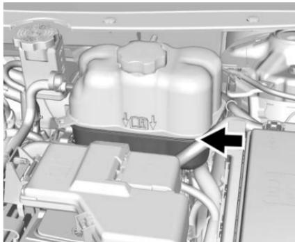
Check to see if coolant is visible in the coolant surge tank. If the coolant inside the coolant surge tank is boiling, do not do anything else until it cools down. If coolant is visible but the coolant level mark is not visible, add a 50/50 mixture of clean, drinkable water and DEX-COOL coolant at the coolant surge tank to the top rib on the middle of the tank, but be sure the
