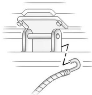
5. Lower the liftgate enough to be able to hook the cable onto the outside portion of the liftgate hinges.
