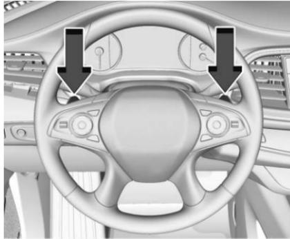
Electronic Range Select (ERS), or Manual Mode, allows for the selection of the range of gear
