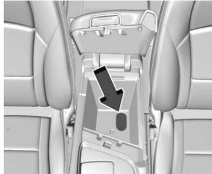
1. Remove the top tray and the rubber mat inside the center console storage area. Place the new transmitter into the transmitter pocket.
