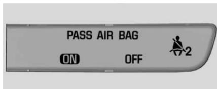
The passenger sensing system turns off the front outboard passenger frontal airbag under certain conditions. No other airbag is affected by the passenger sensing system. See *Passenger Sensing System* ⇨ 89.
