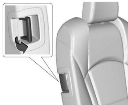
2. Pull the handle on the side of the seat forward and pull the seat forward.
