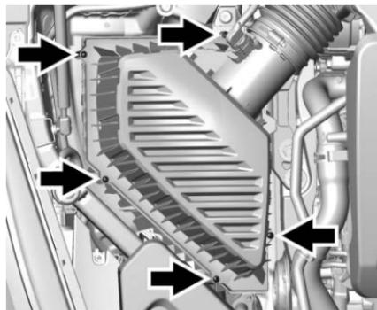
1. Remove the five screws and lift the cover off the air cleaner/filter housing.
