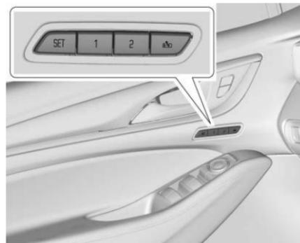
If equipped, memory seats allow two drivers to save and recall their unique seat positions for driving the
