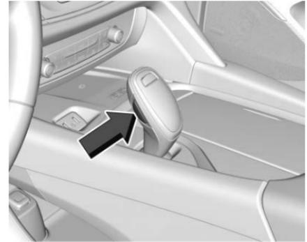
This vehicle is equipped with an electronic transmission. The shift lock release button is designed to prevent inadvertent shifting out of P (Park) unless the ignition is on, the brake pedal is applied, and the shift lock release button is pressed.
