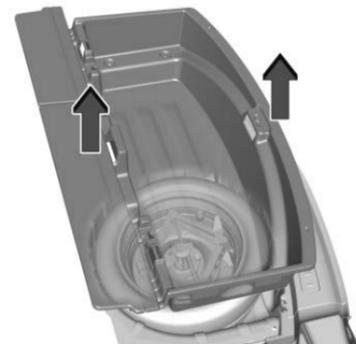
3. Lift up on the cargo management system to access the spare tire.
