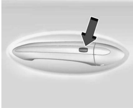
The RKE transmitter must be within 1 m (3 ft) of the liftgate or door being opened. Press the button on the door handle to open. See *Remote Keyless Entry (RKE) System Operation* ⇨ 29.
