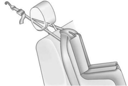
If the position you are using has an adjustable head restraint and you are using a dual tether, raise the head restraint and route the tether around the head restraint posts.
