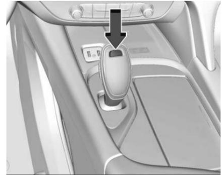
2. Press the P button on the shift lever.
