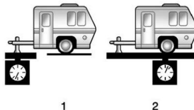
The trailer tongue weight (1) should be 10–15% of the loaded trailer weight (2). Some specific trailer types, such as boat trailers, fall
