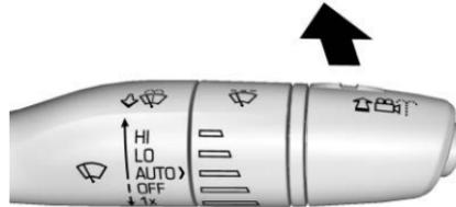
If equipped, push the windshield wiper lever forward to spray washer fluid on the rear camera lens. The lever returns to its starting position when released. See *Rear Camera Mirror* ⇨ 53.
