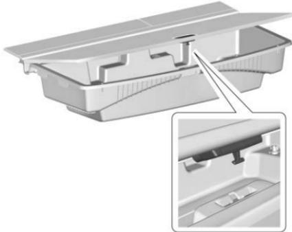
3. Make sure to properly latch the top of the load floor.
