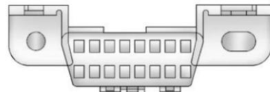
The DLC is under the instrument panel to the left of the steering wheel. Connecting devices that are not used to perform an Emissions Inspection/Maintenance test or to service the vehicle may affect vehicle operation. See *Add-On Electrical Equipment* ⇨ 262. See your dealer if assistance is needed.
