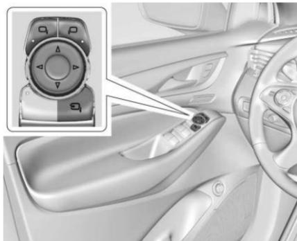
If equipped, press
