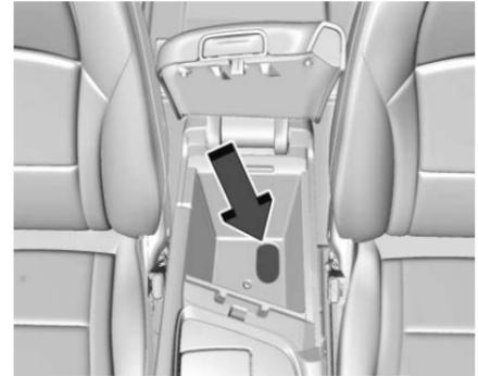
3. Remove the top tray and the rubber mat inside the center console storage area. Place the new transmitter into the transmitter pocket.
