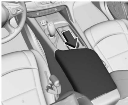
The center console has storage under the armrest. Pull up on the latch, and lift to open.
