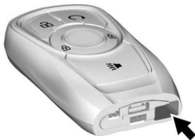
2. Insert a flat, thin object and remove the back cover.
