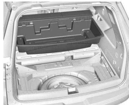
4. The cargo management system can be placed on the lowered third row seats while accessing the spare tire.
