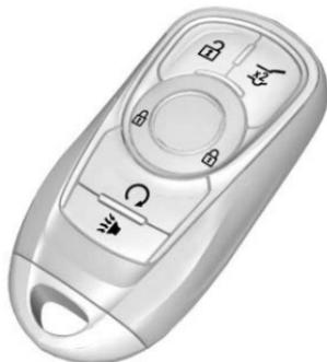
The Remote Keyless Entry (RKE) transmitter may be used to lock and unlock the doors from up to 60 m (197 ft) away from the vehicle.
