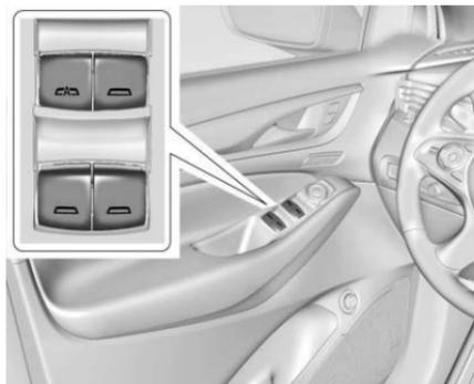
Power windows work when the ignition is on, in ACC/ACCESSORY, or in Retained Accessory Power (RAP). See *Retained Accessory Power (RAP)* ⇨ 203.
