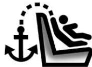
To assist in locating the top tether anchors, the top tether anchor symbol is near the anchor.
