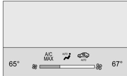
The climate control status display appears briefly when the climate controls on the center stack are adjusted. The air delivery mode can be adjusted on the climate control display.
