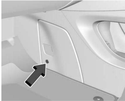
3. Use a flat-bladed tool to remove the fastener located in the lower front corner of the interior trim panel on the center console to the right of the accelerator pedal.
