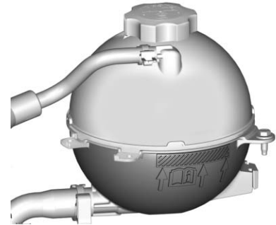
3.6L V6 Engine Coolant Surge Tank
