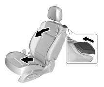
To fold the seatback, lift the release lever and fold the seatback forward. The seat will slide forward.
