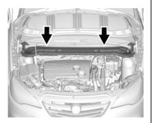
The air intake in front of the windshield in the engine compartment must be kept clear to allow air intake. Remove any leaves, dirt, or snow.
