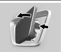
2. Push the tool to disengage the clip and remove the sidemarker housing. Do not use excessive force.
