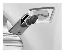
Turn the bulb socket 90° counterclockwise and remove it from the housing.
