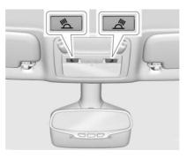
nor a : Press the button near each lamp to turn it on or off.
