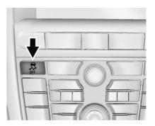
Do not repeatedly brake or accelerate heavily when TCS is off. The vehicle driveline could be damaged.
