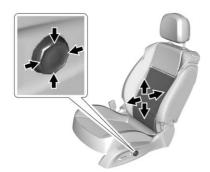
If equipped, press and hold the front of the switch to increase lumbar support, or the rear of the switch to decrease lumbar support.
