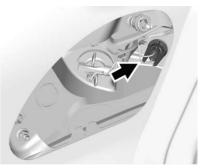
2. Remove the bulb holder by turning it counterclockwise.
