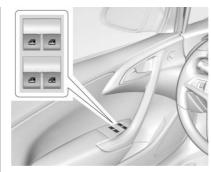
Power windows work when the ignition is on, in ACC/ACCESSORY, or when Retained Accessory Power (RAP) is active. See *Retained Accessory Power (RAP)* ⇔ *148*.
