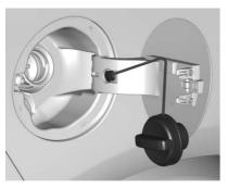
Turn the fuel cap counterclockwise to remove. While refueling, hang the tethered fuel cap from the hook on the fuel door.
