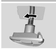
3. Turn the bulb holder counterclockwise and remove it from the housing.
