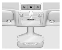
The interior lamps control in the overhead console controls both the front and rear interior lamps.
