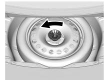
3. Turn the retainer nut counterclockwise to remove it.
