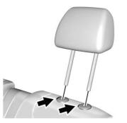
2. Press both buttons on the head restraint posts at the same time, and pull up on the head restraint.
