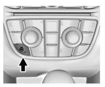
If equipped with a heated steering wheel, press to turn it on or off. A light on the button displays when the feature is turned on. The steering wheel takes about three minutes to start heating.
