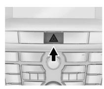
A: Press to make the front and rear turn signal lamps flash on and off. This warns others that you are having trouble. Press again to turn the flashers off.
