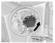
Turn the bulb holder counterclockwise to disengage. Remove the bulb holder from the reflector.
