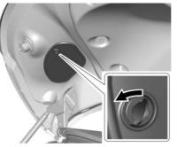
The cover is inside the trunk lid. Remove the screw on the cover with a tool and turn clockwise to remove the cover.
