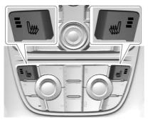
If equipped, the controls are on the climate control panel. The engine must be running to operate the heated seats.
