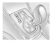
Move the shift lever from D (Drive) to the left into the (+) or (-) manual position.
