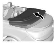
4. With an additional person, lift the tonneau cover from both sides to approximately the half raised position.
