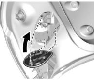
5. Close the cover by inserting the fastener clips first. Lock the cover by turning the screw clockwise with a tool.
