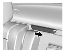
1. Remove the cover from the mount between the rear head restraints by sliding it toward the driver side of the vehicle.
