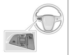
☆: Press to turn the cruise control system on or off. A white indicator comes on in the instrument cluster when cruise is turned on.
