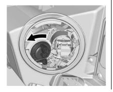
2. Turn the bulb socket counterclockwise and remove it from the reflector.
