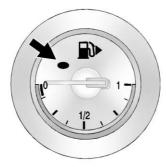
This light comes on for a few seconds when the ignition is turned on as a check to indicate it is working. If it does not come on, have it fixed. The low fuel warning light comes on and a chime sounds when the vehicle is low on fuel. The light turns off when fuel is added to the fuel tank.
