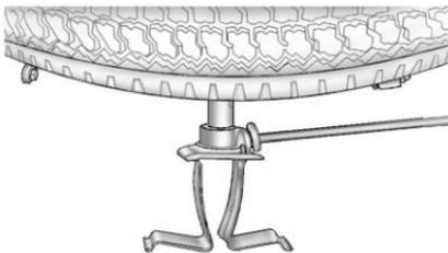
8. Attach the jack handle, extension, and wheel wrench to the jack and place it (with the wheel blocks) under the vehicle toward the front of the rear bumper.
