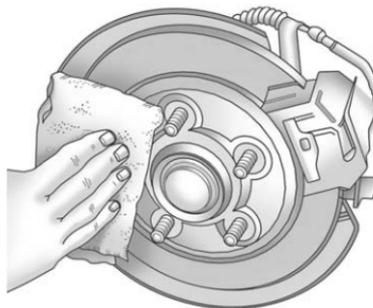
7. Remove any rust or dirt from the wheel bolts, mounting surfaces, and spare wheel.
