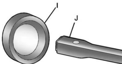
5. Insert the open end of the extension (J) through the hole in the rear bumper (I) (hoist shaft access hole).
