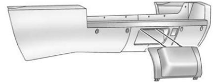
1. Turn the fasteners on the lower tabs 90 degrees counterclockwise.
