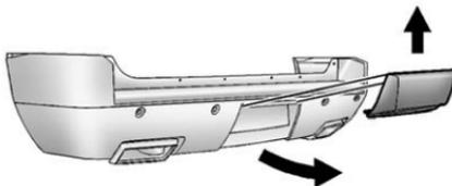
1. Turn the fasteners on the lower tabs 90 degrees counterclockwise.
