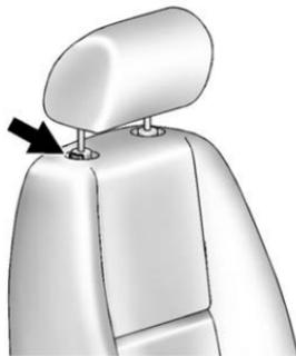
The height of the head restraint can be adjusted. Pull the head restraint up to raise it. Try to move the head restraint to make sure that it is locked in place.
