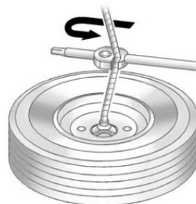
7. Use the wheel wrench hook to pull the hoist cable closer to assist in reaching the spare tire.
