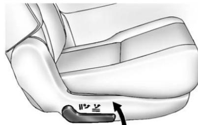
1. Lift the lever on the outboard side of the seat.
