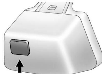
The light sensor is located on the inside of the vehicle in front of the inside rearview mirror.
