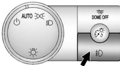
The fog lamp button is located on the left side of the instrument panel.
