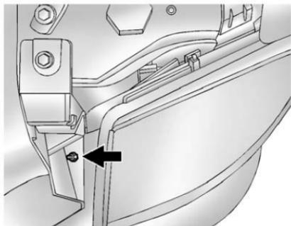
7. Locate the vertical headlamp aiming screws, which are under the hood near each headlamp assembly.
