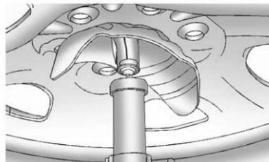
9. Position the center lift point of the jack under the center of the spare tire.
