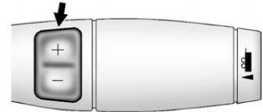
The DSC switch is located on the shift lever.
