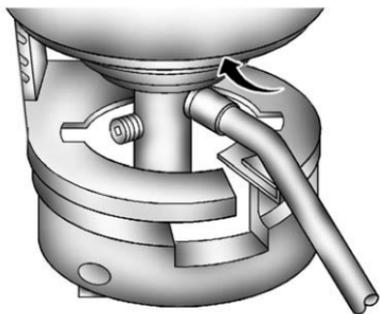
4. Turn the tire sealant canister (B) so the inflator filling hose is aligned with the slot in the compressor.
