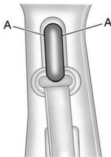
Squeeze the buttons (A) on the sides of the height adjuster and move the height adjuster to the desired position.
