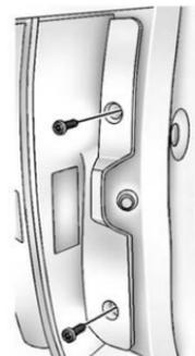
2. Remove the two screws from the taillamp assembly.
