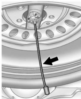
1. Check under the vehicle to see if the cable end is visible. If the cable is not visible proceed to Step 6.
