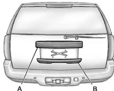
The liftglass or liftgate cannot be opened if the rear wiper is in motion. Attempting to open the liftglass or liftgate while the rear wiper is in motion will cause the release of the liftglass or liftgate to delay until the wipers are parked off the liftglass.
