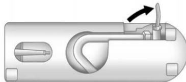
1. Unlock the air only hose (F) from the tire sealant canister (B) by pulling up on the lever.
