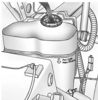
3. Fill the coolant surge tank with the proper mixture to the FULL COLD mark.
