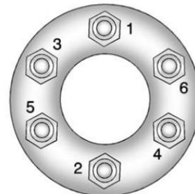
11. Tighten the nuts firmly in a crisscross sequence as shown by turning the wheel wrench clockwise.
