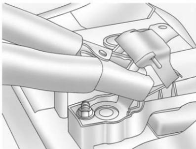
6. Connect the red positive (+) cable to the positive (+) terminal of the vehicle with the dead battery. Use a remote positive (+) terminal if the vehicle has one.
