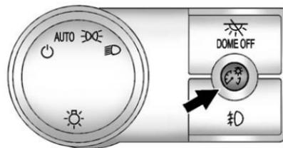
**(Instrument Panel Brightness):** This feature controls the brightness of the instrument panel lights and is located next to the exterior lamps control.
