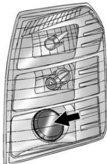
2. Locate the center of the projector lens of the low-beam headlamp.
