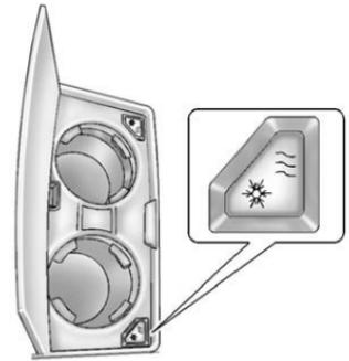
To set to cool mode, press and release the button; the ❄️ shows blue. Press and release again to turn it off.
