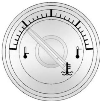
This gauge shows the engine coolant temperature.
