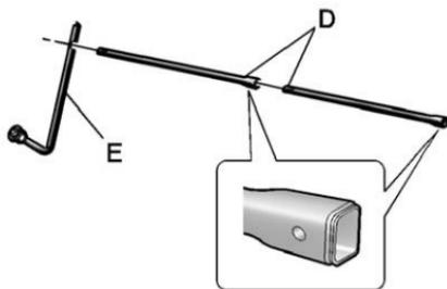
4. Assemble the two jack handle extensions (D) and wheel wrench (E), as shown.
