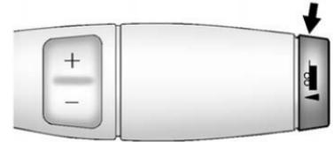
The vehicle has a Tow/Haul Mode. The Tow/Haul Mode adjusts the transmission shift pattern to reduce shift cycling, providing increased performance, vehicle control, and transmission cooling when driving down steep hills and mountain grades, towing, or hauling heavy loads.
