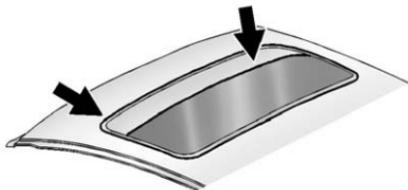
Dirt and debris may collect on the sunroof seal or in the track. This could cause an issue with sunroof operation or noise. It could also plug the water drainage system. Periodically open the sunroof and remove any obstacles or loose debris. Wipe the sunroof seal and roof sealing area using a clean cloth, mild soap, and water. Do not remove grease from the sunroof.
