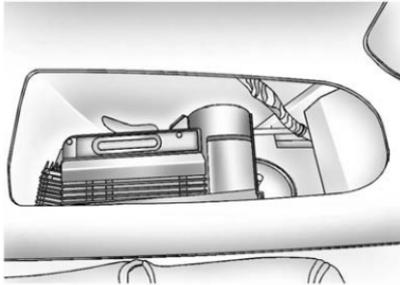
2. Locate the tire sealant and compressor kit.
