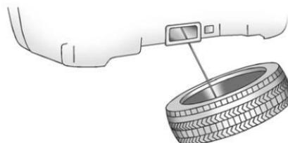
2. Tilt the tire toward the vehicle. Separate the tire/wheel retainer from the guide pin. Pull the pin through the center of the wheel. Tilt the retainer down and through the center wheel opening.
