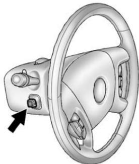
Push the control up or down to tilt the steering wheel up or down.
