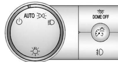
The exterior lamps control is located on the instrument panel to the left of the steering wheel.
