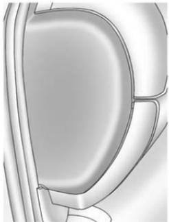
The instrument panel fuse block access door is located on the driver side edge of the instrument panel. Pull off the cover to access the fuse block.
