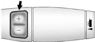
The vehicle has Driver Shift Control (DSC). DSC controls the vehicle's transmission and vehicle speed while driving down hill or towing a trailer by allowing you to select a desired range of gears.
