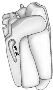
3. Lift the lever again to release the rear of the seat from the floor. The seat will tumble forward.
