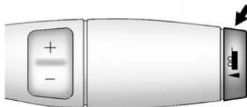
Pressing this button at the end of the shift lever turns on and off the tow/haul mode.
