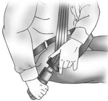
3. Push the latch plate into the buckle until it clicks. If you find that the latch plate will not go fully into the buckle, see if you are using the correct buckle.
