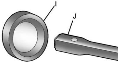
4. Insert the open end of the extension (J) through the hole in the rear bumper (I) (hoist shaft access hole).
