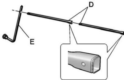
3. Assemble the two jack handle extensions (D) and wheel wrench (E), as shown.
