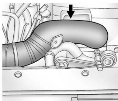
4. With the coolant surge tank pressure cap off, start the engine and let it run until the upper radiator hose can be felt getting hot. Watch out for the engine cooling fan.
