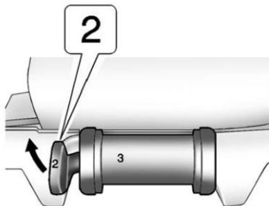
4. Unlatch the seat from the floor by lifting lever “2” next to the carrying handle on the rear of the seat, near the bottom.
