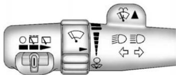
The front and rear wiper controls are located on the turn and lane-change lever.
