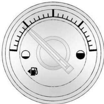
When the ignition is on, the fuel gauge shows about how much fuel the vehicle has left in the tank.
