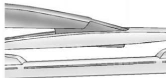
2. Pull the wiper blade assembly away from the backglass. The backglass wiper blade will not lock in a vertical position, so care should be used when pulling it away from the vehicle.
