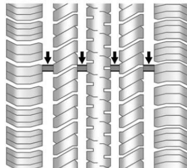
Treadwear indicators are one way to tell when it is time for new tires. Treadwear indicators appear when the tires have only 1.6 mm (1/16 in) or less of tread remaining. Some commercial truck tires may not have treadwear indicators. See *Tire Inspection* on page 10-57 and *Tire Rotation* on page 10-58 for additional information.
