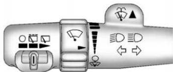
The front wiper control is located on the turn and lane-change lever. Turn the band with the wiper symbol to control the windshield wipers.
