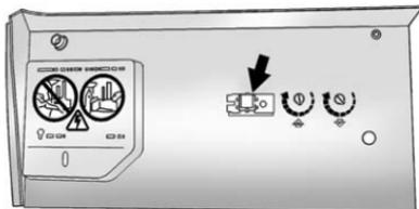
2. In the garage, locate the garage door opener receiver (motor-head unit). Find the "Learn" or "Smart" button. It can usually be found where the hanging antenna wire is attached to the motor-head unit and may be a colored button. Press this button. After pressing this button, complete the following steps in less than 30 seconds.
