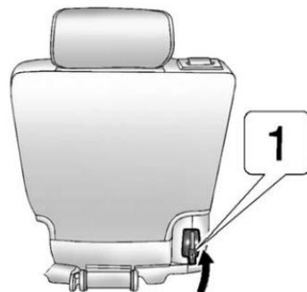
3. Lift the release lever "1" on the bottom rear of the seatback on the outboard side of the seat, and the seatback folds forward.
