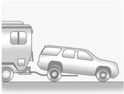
Use the following procedure to dinghy tow a two-wheel-drive vehicle from the rear:
