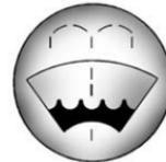
Open the cap with the washer symbol on it. Add washer fluid until the tank is full. See *Engine Compartment Overview* on page 10-6 for reservoir location.
