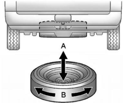
7. Make sure the tire is stored securely. Push, pull (A), and then try to turn (B) the tire. If the tire moves, use the wheel wrench to tighten the cable.
