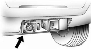
The vehicle has a seven-pin universal heavy-duty trailer connector attached to the rear bumper beam next to the integrated trailer hitch.
