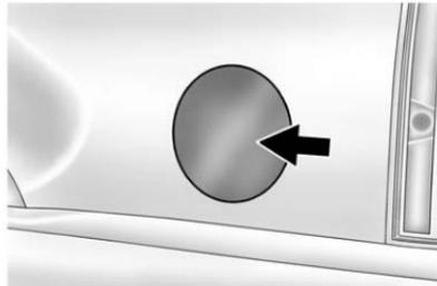
To open the fuel door, push the rearward center edge in and release and it will open.
