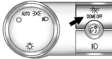
**DOME OFF** (Dome Off): Press the button in and the dome lamps remain off when a door is opened. Press the button again to return it to the extended position so that the dome lamps come on when a door is opened.
