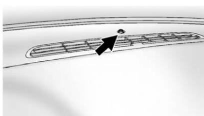
The vehicle has a light sensor located on the top of the instrument panel which regulates when the automatic headlamps turn on. Do not cover the sensor, otherwise the headlamps will come on whenever the ignition is on.
