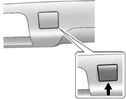
2. Open the hoist shaft access cover on the bumper to access the spare tire lock.
