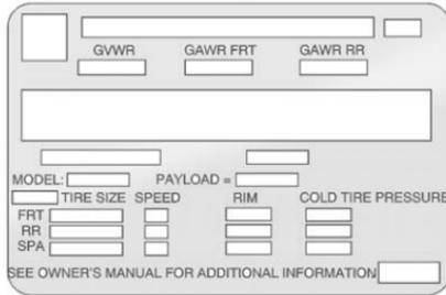
A vehicle specific Certification/Tire label is attached to the rear edge of the driver door. The label shows the size of your vehicle's original tires and the inflation pressures needed to obtain the gross weight capacity of your vehicle. This is called Gross Vehicle Weight
