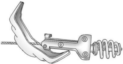
Once the retainer is separated from the pin, tilt the retainer and pull it through the center of the wheel along with the cable and latch.
