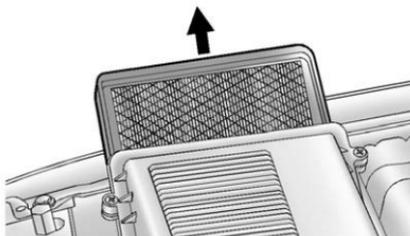
3. Remove the engine air cleaner/filter from the housing. Care should be taken to dislodge as little dirt as possible.
