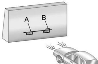
9. Make sure that the light from the headlamp is positioned at the bottom edge of the horizontal tape line. The lamp on the left (A) shows the correct headlamp aim. The lamp on the right (B) shows the incorrect headlamp aim.
