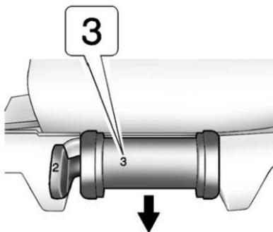
3. Unlatch the seat from the floor by pulling the handle at the rear of the seat "3 Removal Only" toward the rear of the vehicle.
