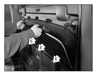
5. Load the rear glass into the storage pocket in the Midgate<sup>®</sup>, guiding the lower edge of the rear glass behind the three rear glass retaining tabs (E). Hold the rear glass flat against the storage pocket, with grab handles facing you, until the next step.
