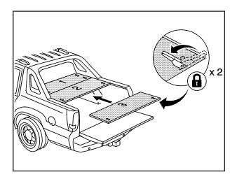
7. Push the latches away from you, starting with the left latch, to lock the panel in place. You should hear a click when each latch locks correctly.
