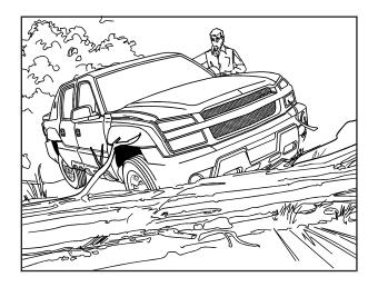
If your vehicle stalls when you are crossing an incline, be sure you, and any passengers, get out on the uphill side, even if the door there is harder to open. If you get out on the downhill side and the vehicle starts to roll over, you will be right in its path.
