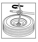
Use the wheel wrench hook that allows you to pull the hoist cable towards you, to assist in reaching the spare tire.
