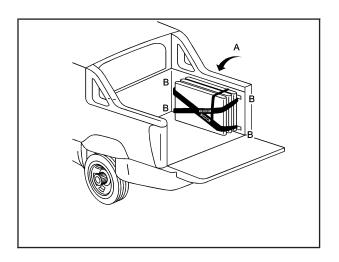
5. Place the primary straps over the three cargo covers (A). Fasten the four strap clips (B).
