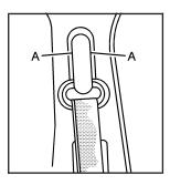
To move it down, squeeze the buttons (A) on the sides of the height adjuster and move the height adjuster to the desired position.
