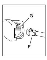
Insert the open end of the extension (F) through the hole in the rear bumper (G) (hoist shaft access hole).
