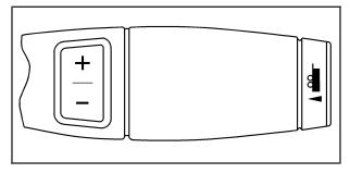
Press the button at the end of the shift lever to enable/disable the Tow/Haul mode.
