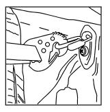
Secure the storage strap system in the cargo storage area by attaching the six clips on the cargo strap system to the tie down locations on either side of the storage area.
