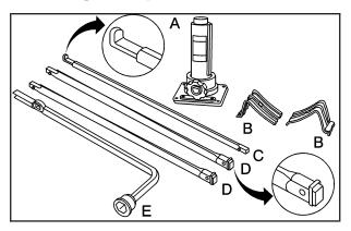
The tools that are needed include the jack (A), the wheel blocks (B), the jack handle (C), the jack handle extensions (D), and the wheel wrench (E).
