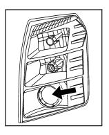
2. Locate the center of the projector lens of the low-beam headlamp.
