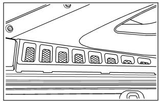
The top drain grates are located near the rear glass on both sides of the vehicle. Clean the grates and drains if there is a blockage. To remove each drain grate, do the following:
