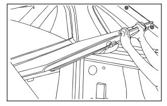
Starting with cargo panel 1, place the latches in the unlocked position. Place cargo panel 1 on the cargo area rails while holding the back of the cargo panel up.
