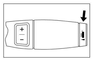
Your vehicle has a tow/haul mode. The tow/haul mode adjusts the transmission shift pattern to reduce shift cycling, providing increased performance, vehicle control, and transmission cooling when towing or hauling heavy loads.
