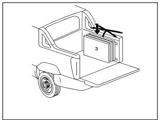
4. Store cargo panel 3 by loading the cargo panel with latches up and facing away from you.
