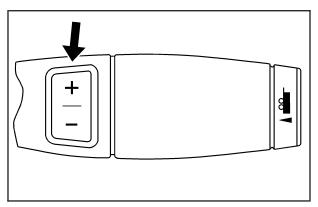
Your vehicle has a Driver Shift Control (DSC). The DSC controls the vehicle's transmission and vehicle speed while driving down hill or towing a trailer by allowing you to select a desired range of gears.
