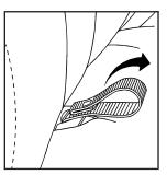
Pull the seat loop located where the seatback and seat cushion meet. The seat cushion will release and allow you to tilt it toward the front of the vehicle.
