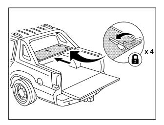
Push both left latches away from you to lock the latches. Remember that there are four latches total for panel 1. You should hear a click when each latch locks correctly. Lock the remaining two right latches on panel 1.
