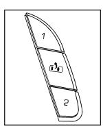
The controls for this feature are located on the driver's door, and are used to program and recall memory settings for the driver's seat, outside mirrors, and the adjustable throttle and brake pedal feature, if your vehicle has it.
