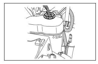
3. Fill the coolant surge tank with the proper mixture, to the FULL COLD mark.
