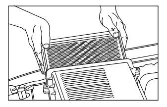
Remove the engine air cleaner/filter from the housing. Care should be taken to dislodge as little dirt as possible.
