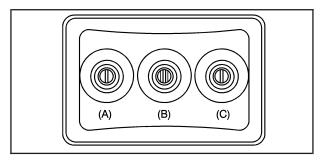
The A/V jacks are located on the rear of the floor console. The A/V jacks allow audio or video signals to be connected from an auxiliary device such as a camcorder or a video game unit to the RSE system. Adapter connectors or cables (not included) may be required to connect the auxiliary device to the A/V jacks. Refer to the manufacturer's instructions for proper usage.
