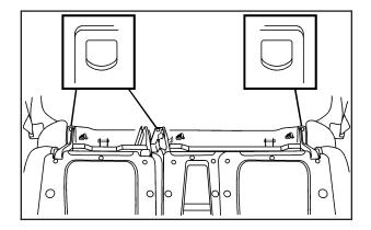
The top tether anchors are located on the back of the rear seat frame above the floor for each rear seating position. Fold down the rear seatback(s) to access the anchors. See *Rear Seat Operation on page 1-10*. Be sure to use an anchor located on the same side of the vehicle as the seating position where the child restraint will be placed.
