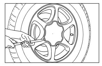
To remove the center cap, place the chiseled end of the wheel wrench in the slot on the wheel and gently pry the cap out.
