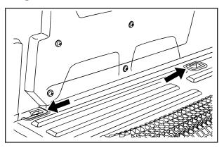
Your vehicle also has four cargo-area floor drains located under the cargo mat near the sides of the cargo area. These drains should be cleaned periodically to allow water to exit the cargo area.
