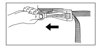
7. Close both cross locks at the center of the strap system to secure tightly.
