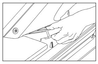
Grasp the edges of the grate and pull it out from the vehicle. Flush the drain with clean water. To replace the drain grate do the following:
