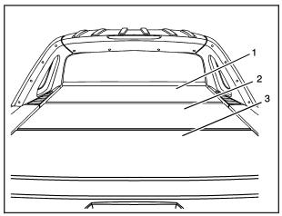
Before removing the cargo panel(s), notice the numbers embossed on the upper center portion of each panel. The panels are labeled 1, 2 and 3. Corresponding numbered labels are also on the bottom of the panels. These numbers on the top and bottom of the panels will be used as reference in the steps for removing, storing and reinstalling the panels.
