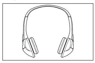
The RSE includes two 2-channel wireless headphones that are dedicated to this system. Channel 1 is dedicated to the DVD player, while Channel 2 is dedicated to RSA selections. These headphones are used to listen to media such as CDs, DVDs, MP3s, DVDAs, radio, any auxiliary source connected to A/V jacks, or the auxiliary input jack, if your vehicle has this feature. The wireless headphones have an On/Off button, channel 1/2 switch, and a volume control.
