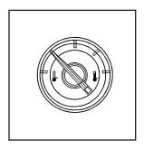
This gage shows the engine coolant temperature.
