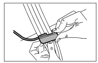
Place the guide over the belt and insert the two edges of the belt into the slots of the guide.
