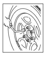
3. Use the wheel wrench to loosen all the wheel nuts.
