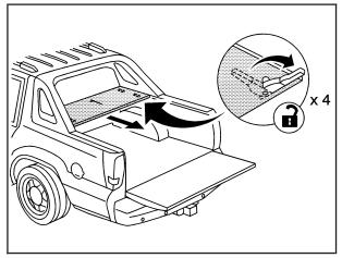
Remove cargo panel 1, but notice that there are four latches to release (two left-side and two right-side latches). Set the panel aside.
