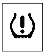
When a low tire pressure condition is detected, the TPMS illuminates the low tire pressure warning light located on the instrument panel cluster.
