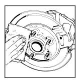
Remove any rust or dirt from the wheel bolts, mounting surfaces, and spare wheel. 8. Install the spare tire.
