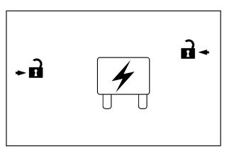
The underhood fuse block is located in the engine compartment, on the driver side of the vehicle. To access the fuse/relay block, push in on the tabs on the end of the fuse/relay block cover and lift.
