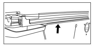
The side rail channels are located on top of both sides of the cargo area. You may want to flush them out with clean water if you notice any debris collecting inside of them.
