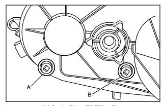
(A) Drain Plug (B) Filler Plug
