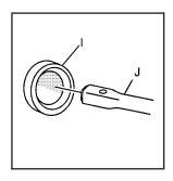
4. Insert the open end of the extension (J) through the hole in the rear bumper (I) (hoist shaft access hole).
