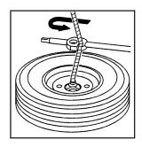
7. Use the wheel wrench hook that allows you to pull the hoist cable towards you, to assist in reaching the spare tire.
