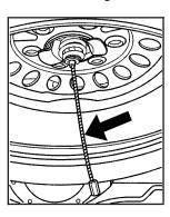
Check under the vehicle to see if the cable end is visible. If the cable is not visible, proceed to Step 6.
