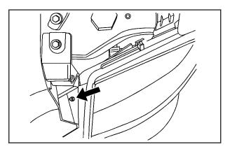
Locate the vertical headlamp aiming screws, which are under the hood near each headlamp assembly.
