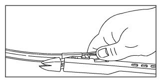
3. Install the new blade onto the arm connector and make sure the grooved areas are fully set in the locked position.
