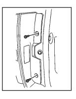
Remove the two screws from the taillamp assembly.
