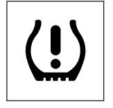
As an added safety feature, your vehicle has been equipped with a tire pressure monitoring system (TPMS) that illuminates a low tire pressure telltale when one or more of your tires is significantly under-inflated.
