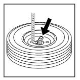
15. Tilt the tire retainer at the end of the cable and pull it through the wheel opening. Pull the tire out from under the vehicle.
