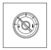
This gage shows the engine coolant temperature.
