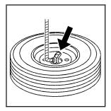
Tilt the tire retainer (G) downward and through the wheel opening. Make sure the retainer is fully seated across the underside of the wheel.
