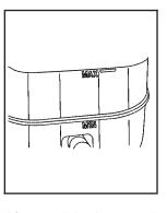
Look at the brake fluid reservoir. The fluid level should be above MIN. If it is not, have your brake system checked to see if there is a leak.
