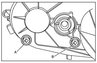
(A) Drain Plug (B) Filler Plug
