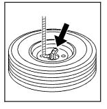
8. Tilt the tire retainer (G) at the end of the cable when the tire has been lowered, so it can be pulled up through the wheel opening.
