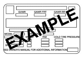
A vehicle specific Certification/Tire label is attached to the rear edge of the driver's door. The label shows the size of your vehicle's original tires and the inflation pressures needed to obtain the gross weight capacity of your vehicle. This is called Gross Vehicle Weight Rating (GVWR). The GVWR includes the weight of the vehicle, all occupants, fuel, and cargo.
