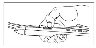
2. Squeeze the grooved areas on each side of the blade, and rotate the blade assembly away from the arm connector.
