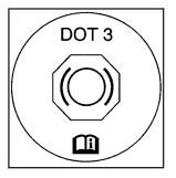
Your brake master cylinder reservoir is filled with DOT-3 brake fluid. See *Engine*Compartment Overview on page 402 for the location of the reservoir.
