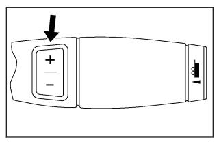
Your vehicle has a Driver Shift Control (DSC). The DSC controls the vehicle's transmission and vehicle speed while driving down hill or towing a trailer by allowing you to select a desired range of gears.
