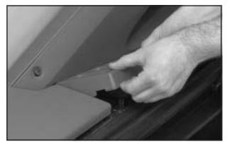
Grasp the edges of the grate and pull it out from the vehicle. Flush the drain with clean water.
