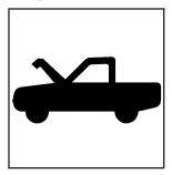
Pull the handle with this symbol on it. It is located inside the vehicle to the lower left of the steering wheel.
