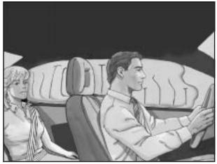
The roof-mounted rollover airbag for the driver and the person seated directly behind the driver is located in the ceiling above the side windows.
