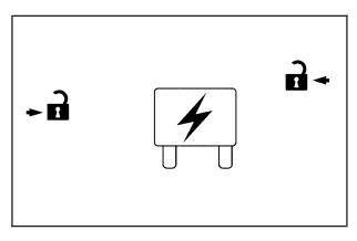
The underhood fuse block is located in the engine compartment, on the driver's side of the vehicle. To access the fuse/relay block, push in on the tabs on the end of the fuse/relay block cover and lift.
