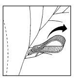
Pull the seat loop located where the seatback and seat cushion meet. The seat cushion will release and allow you to tilt it toward the front of the vehicle. Notice: Folding a rear seat with the safety belts still fastened may cause damage to the seat or the safety belts. Always unbuckle the safety belts and return them to their normal stowed position before folding a rear seat.
