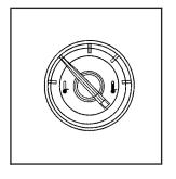
This gage shows the engine coolant temperature.
