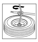
6. Use the wheel wrench hook that allows you to pull the hoist cable towards you, to assist in reaching the spare tire.
