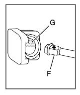
4. Insert the open end of the extension (F) through the hole in the rear bumper (G) (hoist shaft access hole).
