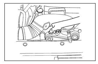
With the coolant surge tank pressure cap off, start the engine and let it run until you can feel the upper radiator hose getting hot. Watch out for the engine cooling fan.
