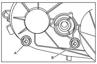
(A) Drain Plug (B) Filler Plug
