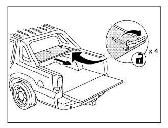
5. Remove cargo panel 1, but notice that there are four latches to release (two left-side and two right-side latches). Set the panel aside.
