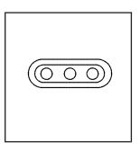
The URPA display is located above the rear window towards the center of the vehicle and can be seen by looking over your right shoulder.
