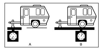
The trailer tongue weight (A) should be 10 percent to 15 percent of the total loaded trailer weight (B), up to a maximum of 600 lbs (272 kg) with a weight carrying hitch. The trailer tongue weight (A) should be 10 percent to 15 percent of the total loaded trailer weight (B), up to the maximum of 1,000 lbs (454 kg) with a weight distributing hitch.
