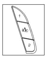
The controls for this feature are located on the driver's door, and are used to program and recall memory settings for the driver's seat, outside mirrors, and the adjustable throttle and brake pedal feature, if your vehicle has it.
