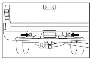
2. Turn the bulb socket counterclockwise and pull the bulb socket out of the connector.
