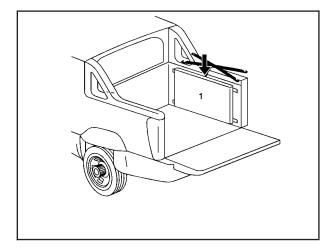
2. Starting with cargo panel 1, load the cargo panel with latches up and facing away from you.
