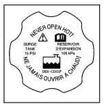
You can remove the coolant surge tank pressure cap when the cooling system, including the coolant surge tank pressure cap and upper radiator hose, is no longer hot.
