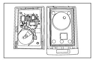
To replace the battery in this type of RKE transmitter do the following:
