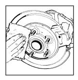
Remove any rust or dirt from the wheel bolts, mounting surfaces, and spare wheel. 7. Install the spare tire.
