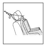
If the position you are using has an adjustable head restraint and you are using a dual tether, route the tether around the head restraint.
