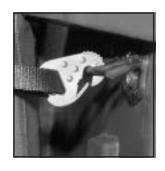
Secure the storage strap system in the cargo storage area by attaching the six clips on the cargo strap system to the tie down locations on either side of the storage area.
