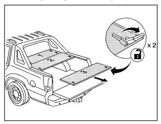
2. Remove cargo panel 3 by pulling the left and right cargo panel latches, located on the bottom of each cargo panel, toward you to unlock the cargo panel latches.
