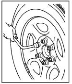
2. Use the wheel wrench to loosen all the wheel nuts. Turn the wheel wrench counterclockwise to loosen the wheel nuts. Do not remove the wheel nuts yet.
