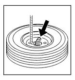
Tilt the tire retainer at the end of the cable when the tire has been lowered, so it can be pulled up through the wheel opening.
