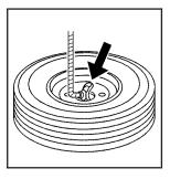
14 Tilt the tire retainer at the end of the cable and pull it through the wheel opening. Pull the tire out from under the vehicle
