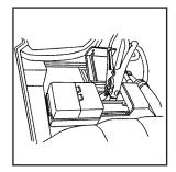
6. Connect the red positive (+) cable to the positive (+) terminal of the vehicle with the dead battery.
