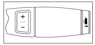
Press the button at the end of the shift lever to enable/disable the tow/haul mode.
