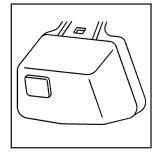
The light sensor is located on the inside of the vehicle in front of the inside rearview mirror.
