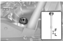
Liquid-cooled intercooler coolant/2.5 T-GDi
