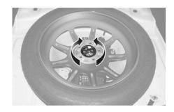
Turn the winged hold down bolt counterclockwise to remove the spare tire.
