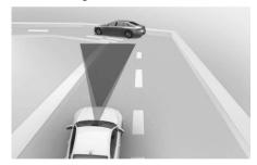
Your vehicle speed can be reduced due to a vehicle in the adiacent lane.
