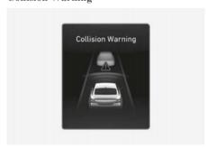
To warn the driver of a collision, the "Collision Warning" warning message appears, and the warning light blinks on the instrument cluster with a warning sound and the steering wheel vibrates.
