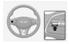
Press the IIO switch to temporarily pause the set speed limit. The set speed limit will turn off but the Speed Limit (SLIMIT) indicator will stay on.
