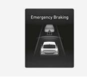
To warn the driver that emergency braking will be assisted, the "Emergency Braking" warning message appears and the warning light blinks on the instrument cluster with a warning sound and the steering wheel vibrates.
