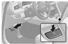
To release EPB (Electronic Parking Brake):
