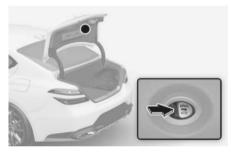
Your vehicle is equipped with an emergency trunk safety release lever located inside the trunk. When someone is inadvertently locked in the trunk, the trunk can be opened by moving the lever in the direction of the arrow and pushing the trunk lid to open.
