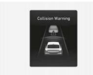
To warn the driver of a collision, the "Collision Warning" warning message appears and the warning light blinks on the instrument cluster with a warning sound and the steering wheel vibrates.
