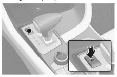
To shift the gear to P (Park), press the **P** button while depressing the brake pedal. If you turn the engine off in R (Reverse) or
