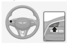
To turn Smart Cruise Control off, press the Driving Assist ( $\mathcal{C}_{\mathcal{C}}$ ) button.
