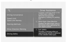
With the engine on, select **Setup** > **Vehicle** > **Driver Assistance** > **Driving Safety** > **Exit Safety** from the Settings menu in the infotainment system to set whether to use each function.
