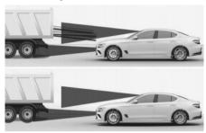
If the vehicle in front of you has cargo that extends rearward from the cab, or when the vehicle in front of you has higher ground clearance, additional special attention is required. Forward Collision-Avoidance Assist may not be able to detect the cargo extending from the vehicle. In these instances, you must maintain a safe braking distance from the rearmost object, and if necessary, steer your vehicle and depress the brake pedal to reduce your driving speed in order to maintain distance.
