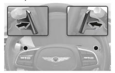
The paddle shifter allows the driver to shift gear without taking one's hands off the steering wheel.
