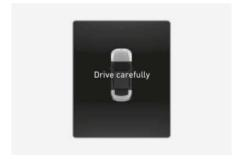
When the vehicle is stopped due to emergency braking, the "**Drive carefully**" warning message will appear on the instrument cluster.
