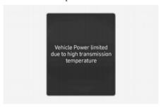
If you continue to drive with overheated transmission, the above warning message appears and self-protection mode restricts the power output of the vehicle.
