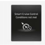
If the Driving Assist button, + switch, - switch or IIO switch is operated when Smart Cruise Control operating conditions are not satisfied, the "Smart Cruise Control conditions not met" will appear on the instrument cluster, and an audible warning will sound.
