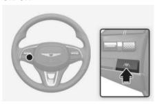
With the engine on, shortly press the Lane Driving Assist (/⊚\) button located on the steering wheel to turn on Lane Following Assist. The gray or green ⊖ indicator light will appear on the instrument cluster.
