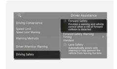
With the engine on, select **Setup** > **Vehicle** > **Driver Assistance** > **Driving Safety** > **Forward Safety** from the Settings menu in the infotainment system to set whether to use each function.
