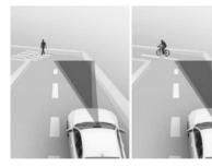
Forward Collision-Avoidance Assist may not detect a vehicle, a powered two-wheeler, and a pedestrian or a cyclist in front of you when driving on curved roads adversely affecting the performance of the sensors. This may result in no warning, braking assist when necessary.
