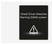
When Driver Attention Warning is not working properly, the "Check Driver Attention Warning (DAW) system" warning message will appear on the instrument cluster for several seconds, and the master (△) warning light and the driver's attention (□) warning light will illuminate on the instrument cluster. If this occurs, have your vehicle inspected by an authorized retailer of Genesis Branded products.
