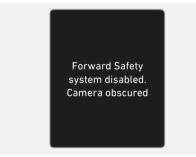
When the front windshield where the front view camera is located, or sensor is covered with foreign material, such as snow or rain, it can reduce the detecting performance and temporarily limit or disable Lane Keeping Assist.
