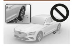
Never start or run the engine while an AWD vehicle is raised on a jack. The vehicle can slip or roll off of a jack causing serious injury or death to you or those nearby.
