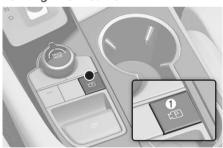
Press the Parking/View button (1) to turn on Rear View Monitor.
