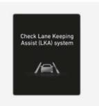
When Lane Keeping Assist is not working properly, the "Check Lane Keeping Assist (LKA) system" warning message will appear and the yellow indicator light will illuminate on the instrument cluster. If this occurs, have your vehicle inspected by an authorized retailer of Genesis Branded products.
