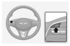
Press the Driving Assist ((C)) button to turn Manual Speed Limit Assist off. The Speed Limit ((SLIMIT) indicator will go off.
