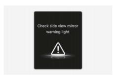
When the side view mirror warning light is not working properly, the "Check side view mirror warning light" warning message will appear on the instrument cluster for several seconds, and the master (△) warning light will illuminate on the instrument cluster. If this occurs, have your vehicle inspected by an authorized retailer of Genesis Branded products.
