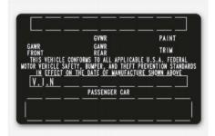
The certification label is located on the driver's door sill at the center pillar and shows the maximum allowable weight of the fully loaded vehicle. This is called the GVWR (Gross Vehicle Weight Rating). The GVWR includes the weight of the vehicle, all occupants, fuel and cargo. This label also tells you the maximum.
