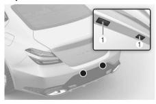
If the LED light (1) does not operate, have the system inspected by an authorized retailer of Genesis Branded products.
