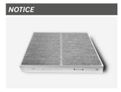
Install a new cabin air filter in the correct direction with the arrow symbol ( $\downarrow$ ) facing downwards, to prevent noise and reduce effectiveness.
