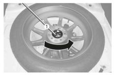
If it is hard to loosen the tire hold-down wing bolt by hand, you can loosen it easily using the jack handle.
