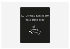
When the conversion from Auto Hold to EPB is not working properly a warning will sound and a message will appear.
