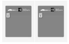
If the speed limit of the road changes during the operation of Manual Speed Limit Assist or Smart Cruise Control, an arrow in the direction of up or down appears to inform the driver that the set speed needs to be changed. At this time, the driver can change the set speed according to the speed limit by using the + or - switch on the steering wheel.
