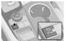
Press the Parking Safety (P<sub>N</sub>) button to turn on Forward/Reverse Parking Distance Warning. Press the button again to turn off the function.
