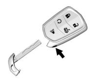
This key, inside the Remote Keyless Entry (RKE) transmitter, is used for the driver door. To remove the key, press the button on the side of the RKE transmitter near the bottom, and pull the key out. Never pull the key out without pressing the button.
