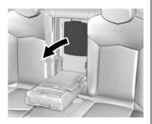
Some vehicles have a rear seat pass-through door in the center of the rear seatback. Fold down the center armrest and pull the latch to open the door. See *Armrest Storage*  $\Rightarrow$  115.
