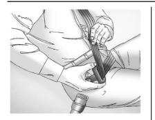
If the webbing locks in the latch plate before it reaches the buckle, tilt the latch plate flat to unlock.
