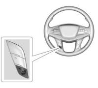
If equipped with a heated steering wheel, press to turn on or off. An indicator next to the button is lit when the feature is turned on.
