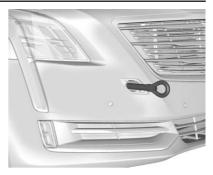
Install the tow eye into the socket and turn it until it is fully tightened. When the tow eye is removed, reinstall the cover with the notch in the original position.
