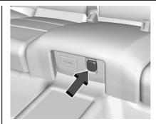
The vehicle has an accessory power outlet on the rear seat trim panel.
