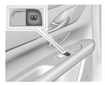
The rear door panels have controls for the rear sunroof sunshade. Press 🔳 to open or close.
