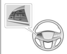
(6): Press to turn the system on and off. A white indicator appears in the instrument cluster when turned on.
