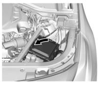
Lift the fuse block cover to access the fuses.
