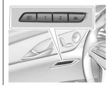
If equipped, memory seats allow two drivers to save and recall their unique seat positions for driving the vehicle, and a shared exit position for getting out of the vehicle. Other feature positions may also be saved, such as power mirrors and power steering wheel, if equipped. Memory positions are linked to RKE transmitter 1 or 2 for automatic memory recalls.
