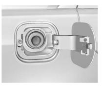
To open the fuel door, push and release the rearward center edge of the door. If equipped, the fuel door is locked when the vehicle doors are locked. Press a on the RKE transmitter to unlock.
