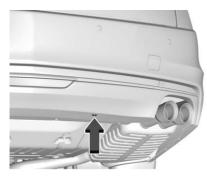
Clean the recessed lens using a soft, dampened cloth.
