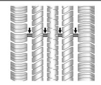
Treadwear indicators are one way to tell when it is time for new tires. Treadwear indicators appear when the tires have only 1.6 mm (1/16 in) or less of tread remaining. See *Tire Inspection*  $\Rightarrow$  *349* and *Tire Rotation*  $\Rightarrow$  *350*.
