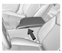
Press the button and lift to access the storage area. There are two USB ports inside. See the infotainment manual.
