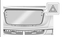
$\triangle$ : Touch this button to make the front and rear turn signal lamps flash on and off. Touch again to turn the flashers off.
