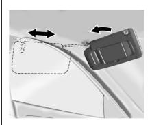
Pull the sun visor down to block glare. Detach the sun visor from the center mount to pivot to the side window, or to extend along the rod.
