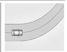
When entering a curve, Super Cruise may not detect the lane markings and may not adjust the steering enough to stay in your lane of travel. When this happens, you will need to steer the vehicle.
