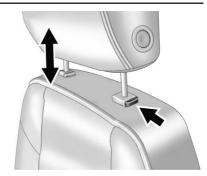
Pull the head restraint up to raise it. Try to move the head restraint to make sure that it is locked in place.
