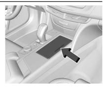
There are cupholders in the center console. Push and release on the passenger side of the cover to access the cupholders.
