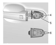
2. Insert the two tabs (6) at the back of the cap between the seal (5) and the metal base (4).
