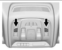
Press 🐨 or 场 next to each overhead console reading lamp.
