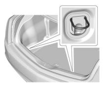
The cargo tie-downs can be used to secure small loads and the convenience net. See *Convenience Net* ⇔ *117*, if equipped.
