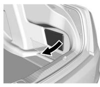
The rear compartment fuse block is behind a cover on the passenger side.
