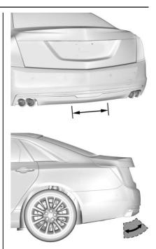
To operate, kick your foot straight up in one swift motion under the center of the rear bumper at the location of the projected logo, then pull it back.
