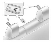
The top tether anchors are behind the rear seat, on the filler panel. Open the covers to access the anchors. Be sure to use an anchor on the same side of the vehicle as the seating position where the child restraint will be placed.
