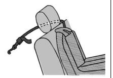
If the position you are using has an adjustable head restraint and you are using a single tether, route the tether around the inboard side of the head restraint.
