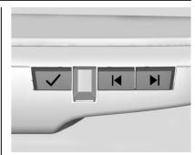
Press  $\checkmark$  to scroll through the adjustment options.
