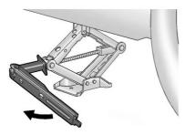
Raise the vehicle by turning the jack handle clockwise. Raise the vehicle far enough off the ground so there is enough room for the road tire to clear the ground.
