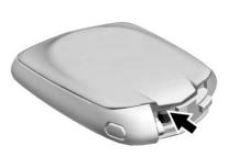
Separate the two halves of the 2. transmitter using a flat tool inserted into the bottom center of the transmitter. Do not use the key slot.
