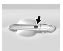
Press the lock/unlock button when the RKE transmitter is within 1 m (3 ft) of the driver door handle. When unlocking from the driver door, the first press unlocks that door; press again within five seconds to unlock all passenger doors. See *Remote Keyless Entry (RKE) System Operation*  $\Rightarrow$  29.
