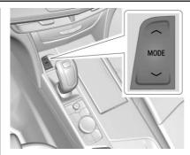
The Driver Mode Control has multiple modes: Tour, Sport, Snow/Ice, and Track. The Track Mode is available for V-Series models only. All modes have preset vehicle settings for use in different driving conditions. For further detail see "Mode Description".
