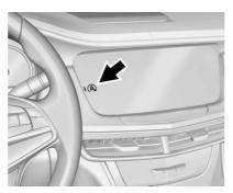
The automatic engine Stop/Start function can be disabled by touching A on the center stack. Auto Stop is enabled each time you start the vehicle.
