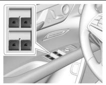
Power windows work when the ignition is on, in ACC/ACCESSORY, or when Retained Accessory Power (RAP) is active. See *Retained Accessory Power* (*RAP*)  $\Leftrightarrow$  205.
