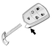
Press the button on the side of 1. the RKE transmitter near the bottom and pull the key out. Never pull the key out without pressing the button.
