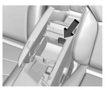
5. Place the new transmitter in the transmitter pocket. The center console storage area will need to be opened.
