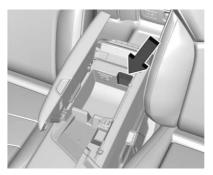
4. Place the new transmitter into the transmitter pocket. The center console storage area will need to be opened.
