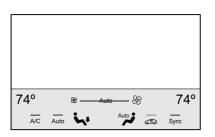
The climate control status display appears briefly when the climate control buttons on the center stack are adjusted.
