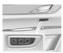
If equipped, press 2 to tilt the front of the seat fully downward and to move the entire seat fully rearward. The seat will also move to this position when the rear door is opened.
