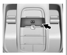
If equipped, press and release the switch. The rear window sunshade will fully extend. To close the sunshade, press and release the switch again. The sunshade will fully close.
