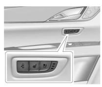
If equipped, press 🔁 to tilt the front of the seat fully downward and to move the entire seat fully rearward. The seat will also move to this position when the rear door is opened.
