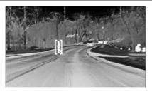
With the Front Pedestrian Braking system turned on, Night Vision provides a red Head-Up Display (HUD) alert when the system detects that the vehicle is approaching a pedestrian ahead much too quickly. In addition, an alert beeps or the Safety Alert Seat pulses, if equipped. See *Front Pedestrian Braking (FPB) System* ⇔ 263.
