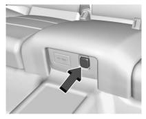
The vehicle has an accessory power outlet on the rear seat trim panel.
