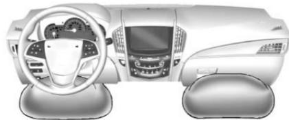
The driver knee airbag is below the steering column. The front outboard passenger knee airbag is below the glove box.
