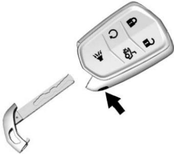
This key, inside the Remote Keyless Entry (RKE) transmitter, is used for the driver door, rear folding seats and rear seat pass-through door.
