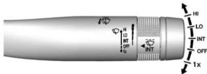
With the ignition in ACC/ACCESSORY or ON/RUN/START, move the lever to select the wiper speed.
