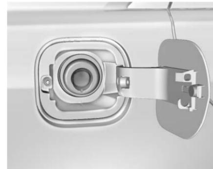
To open the fuel door, push and release the rearward center edge of the door. The fuel door is locked when the vehicle doors are locked. Press
