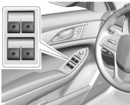
The driver power window switches control all the windows. The passenger switch only controls that window.
