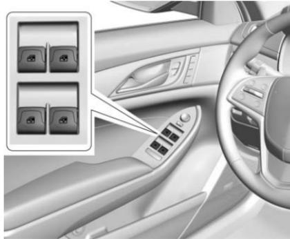
The windows work when the vehicle is in ON/RUN or ACC/ACCESSORY, or when Retained Accessory Power (RAP) is active. See *Retained Accessory Power (RAP)* ⇨ 208.
