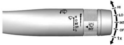
With the ignition in ACC/ACCESSORY or ON/RUN/START, move the windshield wiper lever to select the wiper speed.
