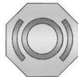
The brake master cylinder reservoir is filled with GM approved DOT 3 brake fluid as indicated on the reservoir cap. See *Engine Compartment Overview* ⇨ 265 for the location of the reservoir.
