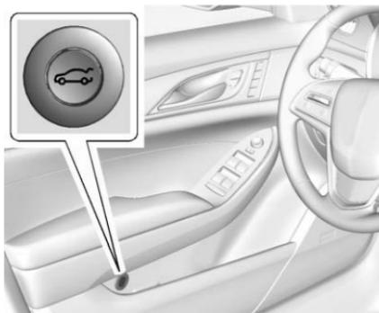
To open the trunk, the vehicle must be off or the shift lever must be in P (Park).
