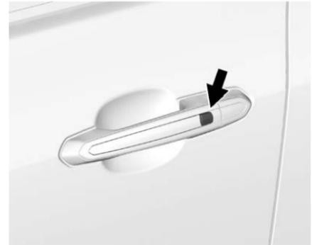
Use the Keyless Access system to lock and unlock the door. When the doors are locked and the Remote Keyless Entry (RKE) transmitter is within 1 m (3 ft) of the driver door handle, press the lock/unlock button. When unlocking from the driver door, the first press unlocks that door; press
