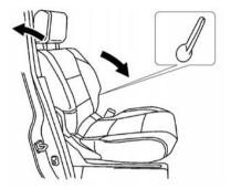
Lift the latch on the inboard side of the seatback to release the seat.
