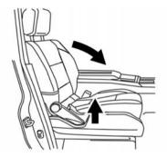
Lift the lever fully and fold the seatback forward until it disengages.
