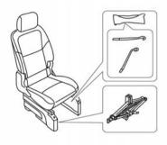
The jack and tools are located under the front passenger seat.
