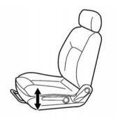
To lift the seat, pull up or push down the lever to adjust the seat.
