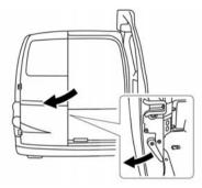
To open the driver side back door, pull the latch release at the inside edge of the door.
