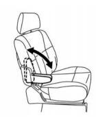
There is an armrest on the inboard side of the driver seat. To raise or lower the armrest, push up or pull down on the armrest.
