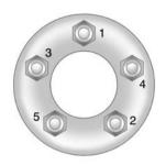
Use the wheel wrench to tighten the nuts firmly. Turn the wheel wrench clockwise and in a crisscross sequence, as shown.
