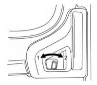
From the inside, slide the lever forward (2) to lock and rearward (1) to unlock.
