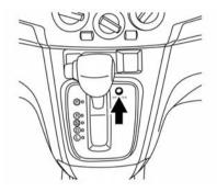
If the battery is discharged, the shift lever may not be moved from the P (Park) position even with the foot brake pedal depressed.
