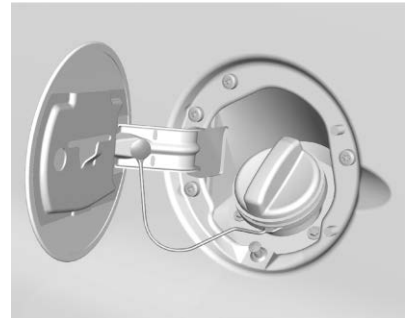
The fuel cap is behind a hinged fuel door on the driver side of the vehicle.
