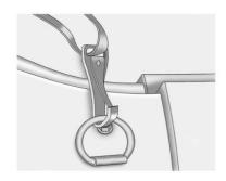
Attach one end of the strap to a cargo tie-down in the rear of the vehicle.
