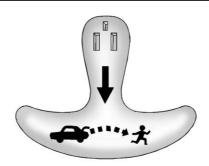
There is a glow-in-the-dark emergency trunk release handle on the underside of the trunk lid. This handle will glow following exposure to light. Pull the release handle down to open the trunk from the inside.
