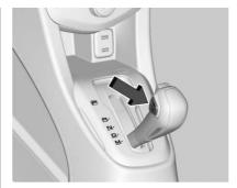
Press the + (plus) end of the button on the side of the shift lever to upshift, or press the -(minus) end of the button to downshift.
