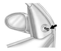
Move the control up, down, or side to side to adjust the mirror.
