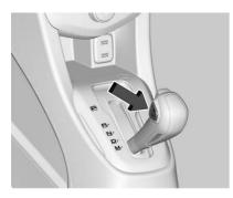
Press the + (plus) end of the button on the side of the shift lever to upshift, or press the -(minus) end of the button to downshift.
