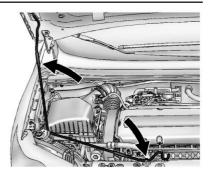
Lift the hood and release the hood prop from its retainer, located in front of the engine compartment. Securely place the hood prop into the slot on the underside of the hood.
