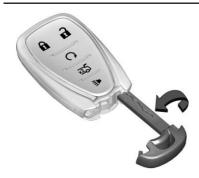
Separate the two halves of the transmitter using the key or a flat tool inserted into the area near the key slot.
