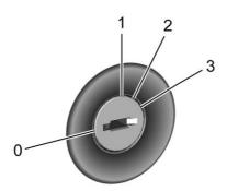
The ignition switch has four different positions.
