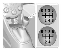
The vehicle may be equipped with a 5-speed or 6-speed manual transmission.
