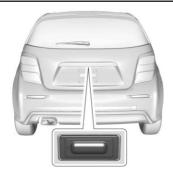
To open the liftgate from the outside, press a on the RKE transmitter to unlock all doors, then use the touch pad.
