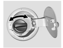
The fuel cap is behind a hinged fuel door on the passenger side of the vehicle.
