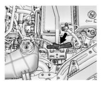
Open the hood and unwrap the electrical cord. The cord is located in the driver side of the engine compartment, near the battery. It is shipped from the factory with a tie holding it in place. Use care in removing the tie so that the cord is not damaged. Check the heater cord for damage. If it is damaged, do not use it. See your dealer for a replacement. Inspect the cord for damage yearly.
