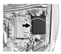
The engine compartment fuse block is on the driver side of the vehicle, near the battery.
