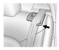
1. Make sure the seat belt is in the retainer hook.
