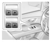
Power windows work when the ignition is on, in ACC/ACCESSORY, or when Retained Accessory Power (RAP) is active. See Retained Accessory Power (RAP) ▷ 187.
