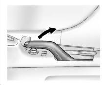
With the brake pedal applied, pull up firmly on the parking brake handle without pressing the release button.
