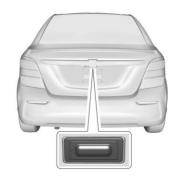
To lock the trunk from the outside press  $\bigcirc$  on the RKE transmitter.
