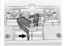
Go to the front of the vehicle and move the secondary hood release lever toward the right side of the vehicle.
