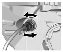
Remove the turn signal lamp bulb socket from the headlamp assembly by turning counterclockwise.
