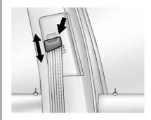
The adjuster can be moved up by pushing the slide/trim up. To move the adjuster down, press the release button and move it down.
