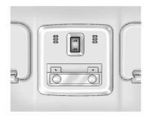
If equipped, the sunroof only operates when the ignition is on or Retained Accessory Power (RAP) is active. See Retained Accessory Power (RAP) ⇒ 187.
