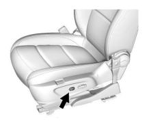
If equipped, press the front or rear of the switch to increase or decrease lumbar support. Release the switch when the desired level of support is reached.
