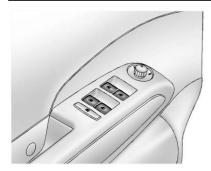
If equipped, the power windows work when the ignition is on, in ACC/ACCESSORY, or when Retained Accessory Power (RAP) is active. See Retained Accessory Power (RAP)
