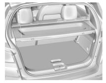
The load compartment cover can be used to conceal objects under it, or it can be removed and placed on the bottom of the load compartment to carry larger loads.
