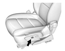
If available, press the front or rear of the switch to increase or decrease lumbar support. Release the switch when the desired level of support is reached.
