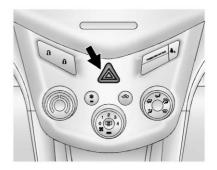
: Press and momentarily hold this button to make the front and rear turn signal lamps flash on and off. This warns others that you are having trouble. Press and momentarily hold again to turn the flashers off.
