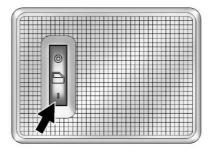
The dome lamp controls are in the headliner above the rear seats.
