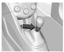
The manual transmission is equipped with a reverse lockout ring. To shift into R (Reverse), press down the clutch pedal, lift up the ring on the shift lever, and shift into R (Reverse). Let up on the clutch pedal slowly while pressing the accelerator pedal.
