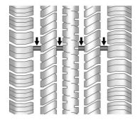
Treadwear indicators are one way to tell when it is time for new tires. Treadwear indicators appear when the tires have only 1.6 mm (1/16 in) or less of tread remaining. See *Tire Inspection*  $\Rightarrow$  263 and *Tire Rotation*  $\Rightarrow$  264.
