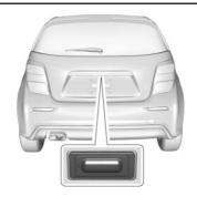
To open the liftgate from the outside, press on the RKE transmitter to unlock all doors, then use the touch pad.
