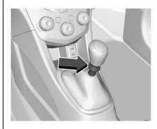
R (Reverse): To back up, press down the clutch pedal, lift up the reverse lockout ring on the shift lever, and shift into R (Reverse). Let up on the clutch pedal slowly while pressing the accelerator pedal.
