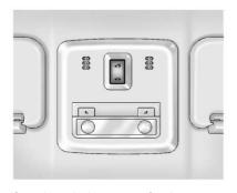
If equipped, the sunroof only operates when the ignition is on or Retained Accessory Power (RAP) is active. See Retained Accessory Power (RAP)
