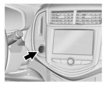
The vehicle may be equipped with an electronic keyless ignition with pushbutton start.
