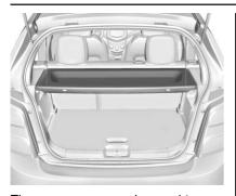
The cargo cover can be used to cover items in the rear of the vehicle.
