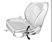
If equipped, move the lever up or down to manually raise or lower the seat.
