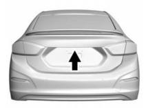
To open the trunk from outside the vehicle, press twice on the Remote Keyless Entry (RKE)
