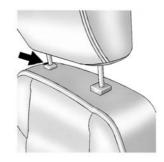
To lower the head restraint, press the button located on the top of the seatback and push the head restraint down. Try to move the head restraint after the button is released to make sure it is locked in place.
