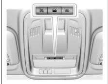
: Press to turn the lamps on automatically when a door is opened.
