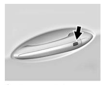
If equipped, press the button on the driver door handle when the RKE transmitter is within 1 m (3 ft) of the driver door handle. When unlocking from the driver door, the first press unlocks that door; press again within five seconds to unlock all passenger doors.
