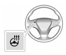
**3**: If equipped, press to turn on or off. A light on the button displays when the feature is turned on.
