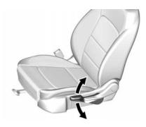
If equipped, move the lever up or down to manually raise or lower the seat.
