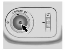
If equipped with front fog lamps, the button is on the exterior lamp control, on the outboard side of the steering wheel.
