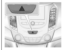
: Press to make the front and rear turn signal lamps flash on and off. This warns others that you are having trouble. Press again to turn the flashers off.
