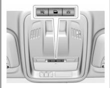
: Press to turn the lamps on automatically when a door is opened.
