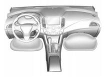
The driver knee airbag is below the steering column. The front outboard passenger knee airbag is below the glove box.
