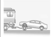
To tow the vehicle with the two rear wheels on the ground and the front wheels on a dolly:
