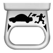
There is a glow-in-the-dark emergency trunk release handle on the trunk lid. The handle will glow following exposure to light. Pull the release handle to open the trunk from the inside.
