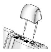
Press both buttons on the head restraint posts at the same time, and pull up on the head restraint.
