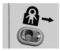
The safety lock is on the inside edge of the rear doors. To use the safety lock:
