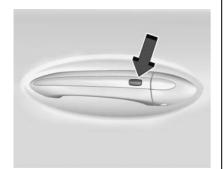
If equipped, the RKE transmitter must be within 1 m (3 ft) of the trunk or door being opened. Push the button on the door handle to open. See "Keyless Access Operation" in Remote Keyless Entry (RKE) System Operation (Key Access)
