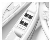
Using the window switch, press to open or pull to close the window.
