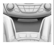
The instrument panel fuse block is in the center of the console, under the climate controls. To access the fuses:
