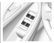
Power windows work when the ignition is on, in ACC/ACCESSORY, or in Retained Accessory Power (RAP). See Retained Accessory Power (RAP) ⇒ 215.
