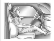
If a person of adult size is sitting in the front outboard passenger seat, but the off indicator is lit, it could be because that person is not sitting properly in the seat or that the child restraint locking feature is engaged. Use the following steps to allow the system to detect that person and enable the front outboard passenger frontal airbag and knee airbag:
