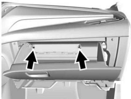
4. Release the retainer clips holding the service door. Open the service door and remove the old filter.
