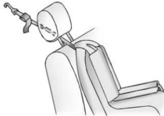
If the position you are using has an adjustable headrest or head restraint and you are using a single tether, route the tether under the headrest or head restraint and in between the headrest or head restraint posts.
