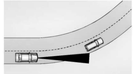
When following a vehicle and entering a curve, ACC may not detect the vehicle ahead and accelerate to the set speed. When this happens the vehicle ahead indicator will not appear.
