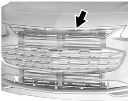
The vehicle may have a shutter system designed to help increase fuel economy. Keep the shutter system clean for proper operation.
