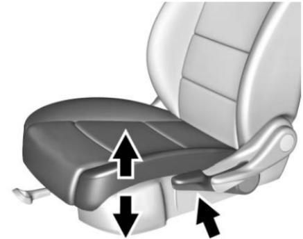
Move the lever on the outboard side of the seat up or down to manually adjust the seat height.
