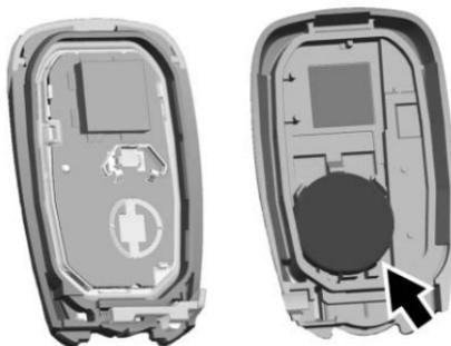
3. Remove the battery by pushing on the battery and sliding it toward the bottom of the transmitter.
