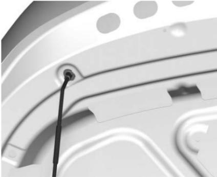
4. Securely place the hood prop rod into the slot on the underside of the hood.
