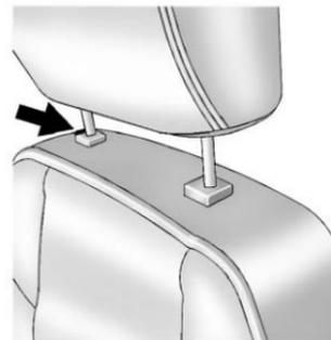
The height of the head restraint can be adjusted. Pull the head restraint up to raise it. Try to move the head restraint to make sure that it is locked in place.
