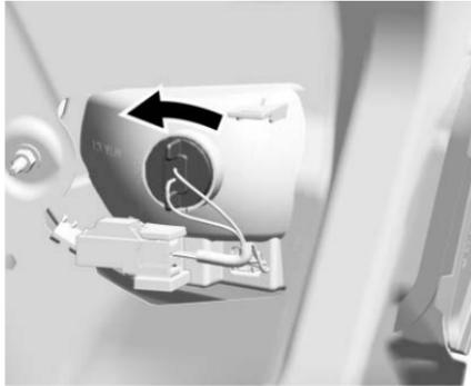
3. Remove the bulb socket by turning counterclockwise and pulling straight out.
