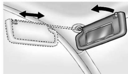
Pull the sun visor down to block glare. Detach the sun visor from the center mount to pivot to the side window, or to extend along the rod, if available.
