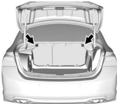
4. Open the trunk and pull the seatback release lever to fold the rear seat.
