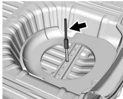
2. Screw the extension bolt onto the end of the spare tire stow bolt by hand.
