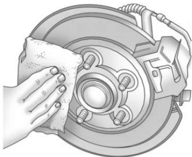
13. Remove any rust or dirt from the wheel bolts, mounting surfaces, and spare wheel.
