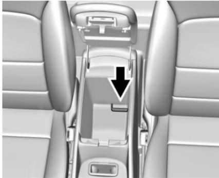
4. Place the new transmitter into the transmitter pocket with the buttons facing toward the rear of the vehicle. The transmitter pocket is inside the center console storage area.
