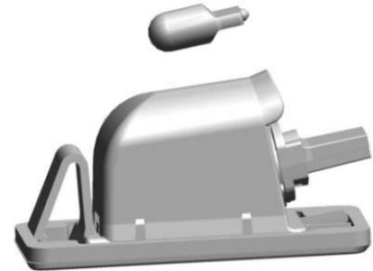
3. Turn the bulb socket counterclockwise to remove it from the lamp assembly.
