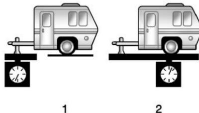
The trailer tongue (1) should weigh 10–15% of the total loaded trailer weight (2). After loading the trailer, weigh the trailer and then the tongue, separately, to see if the weights are proper. If they are not, adjustments might be made by moving some items around in the trailer.
