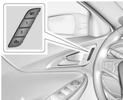
If equipped, memory seats allow two drivers to store and recall their unique seat positions for driving the vehicle, and a shared exit position for getting out of the vehicle. Other feature positions may also be set, such as power mirrors, if equipped. Memory positions are linked to RKE transmitter 1 or 2 for automatic memory recalls.
