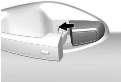
3. Slide the cap forward and press the forward edge to install the cap in place.
