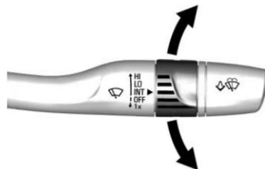
**INT** : Move the lever up to INT for intermittent wipes, then adjust the band to control the frequency of wipes.
