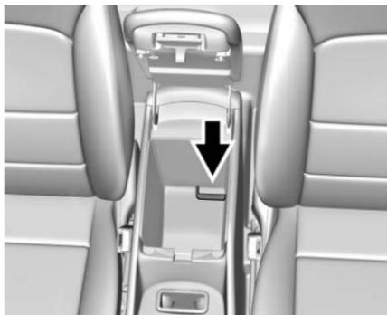
3. Place the first new transmitter into the transmitter pocket with the buttons facing the rear of the vehicle. The transmitter pocket is inside the center console storage area.
