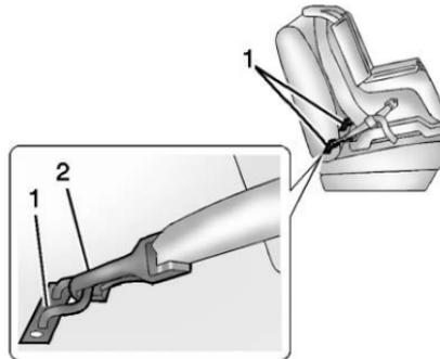
Lower anchors (1) are metal bars built into the vehicle. There are two lower anchors for each LATCH
