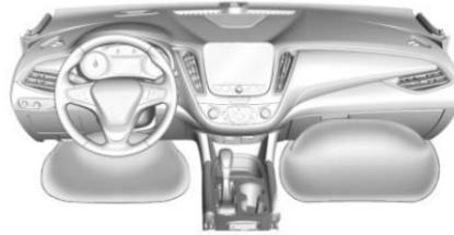
The driver knee airbag is below the steering column. The front outboard passenger knee airbag is below the glove box.
