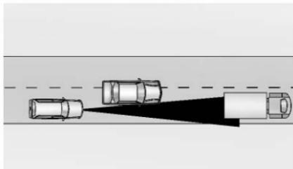
ACC will not detect a vehicle ahead until it is completely in the lane. The brake may need to be manually applied.
