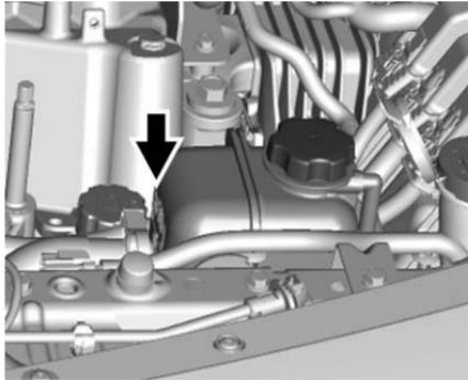
Check to see if coolant is visible in the power electronics coolant reservoir. If coolant is visible but the coolant level is below the indicated mark, there could be a leak in the cooling system.
