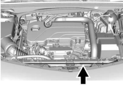
3. Lift the hood and pull the prop rod by the sleeve from the retainer, located above the radiator.
