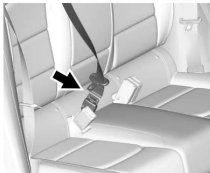
3. Disconnect the rear seat belt mini-latch, using a key in the slot on the mini-buckle.
