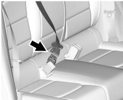
3. Reconnect the rear seat belt mini-latch to the mini-buckle. Do not let it twist.
