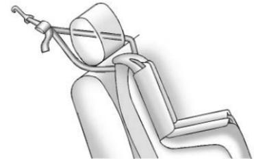
If the position you are using has an adjustable headrest or head restraint and you are using a dual tether route the tether around the headrest or head restraint.
