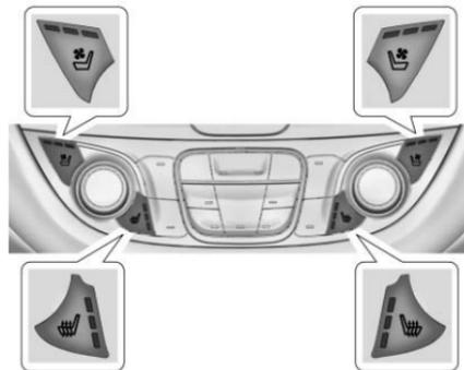
If available, the buttons are on the climate control panel. To operate, the engine must be running.
