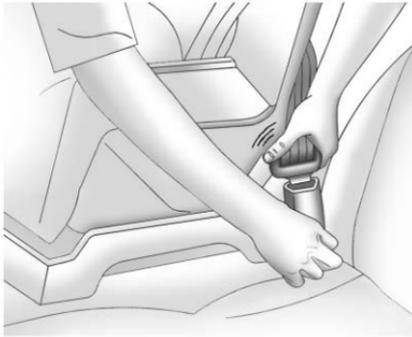
3. Push the latch plate into the buckle until it clicks. If the latch plate will not go fully into the buckle, check if the correct buckle is being used.
