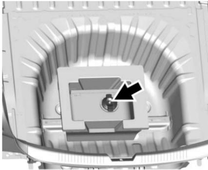
3. Turn the wing nut counterclockwise to remove the tire sealant and compressor kit bag.
