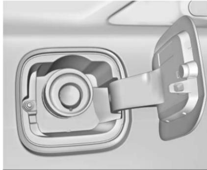
The vehicle has a capless refueling system and does not have a fuel cap. The filling nozzle must be fully inserted and latched prior to starting fuel flow.
