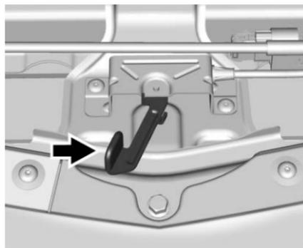
2. Go to the front of the vehicle to find the secondary release handle. The handle is under the front edge of the hood near the center. Slide the secondary hood release handle toward the driver side of the vehicle.
