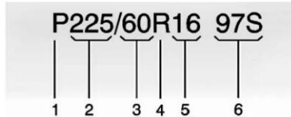
**(1) Passenger (P-Metric) Tire** : The United States version of a metric tire sizing system. The letter P as the first character in the tire size means a passenger vehicle tire engineered to standards set by the U.S. Tire and Rim Association.
