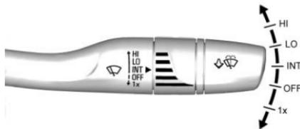
With the ignition on or in ACC/ACCESSORY, move the lever to select the wiper speed.
