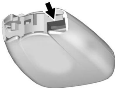
2. Separate the two halves of the transmitter using a flat tool inserted into the area near the key slot.
