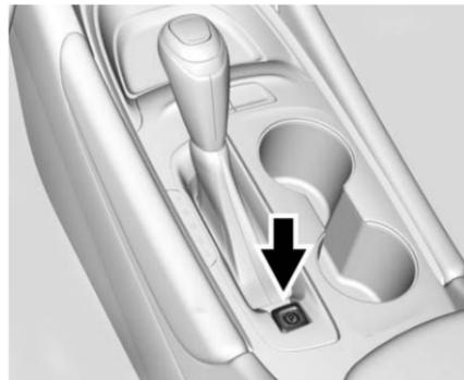
The vehicle may have an Electric Parking Brake (EPB). The EPB can always be activated, even if the ignition is off. To prevent draining the battery, avoid repeated cycles of the EPB system when the engine is
