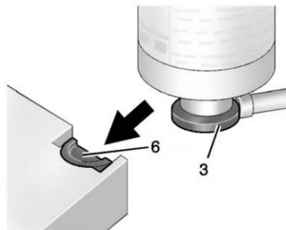
5. Slide the base of the tire sealant canister (3) into the slot on the top of the compressor (6) to hold it upright.
