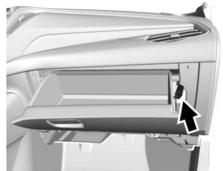
2. Disconnect the glove box door dampener arm from the glove box door assembly.
