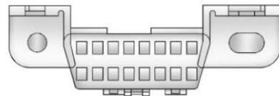
The DLC is under the instrument panel to the left of the steering wheel. Connecting devices that are not used to perform an Emissions Inspection/Maintenance test or to service the vehicle may affect vehicle operation. See *Add-On Electrical Equipment* ⇨ 272. See your dealer if assistance is needed.
