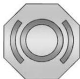
The brake master cylinder reservoir is filled with GM approved DOT 3 brake fluid as indicated on the reservoir cap. See *Engine Compartment Overview* ⇨ 278 for the location of the reservoir.
