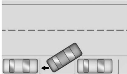
APA will instruct the vehicle to stop once a large enough space is found. Follow the instructions in the DIC. When instructed to drive in reverse, shift to R (Reverse) to engage automatic steering. The steering wheel will briefly vibrate as a reminder to remove hands from the steering wheel. Check surroundings and continue braking or accelerating as needed, and be prepared to stop to avoid vehicles, pedestrians, or objects.
