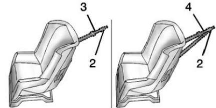
A top tether (3,4) is used to secure the top of the child restraint to the vehicle. A top tether anchor is built into the vehicle. The top tether attachment hook (2) on the child restraint connects to the top tether anchor in the vehicle in order to reduce the forward movement and rotation of the child restraint during driving or in a crash.
