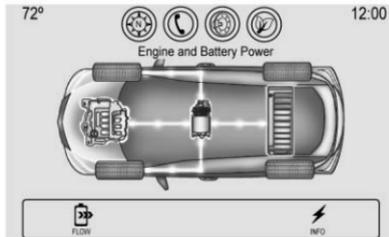
The Power Flow screens indicate the current operating condition. The screens show energy flow between the engine, generator, and high voltage battery. These components will be highlighted when they are active.
