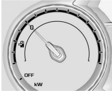
The power gauge indicates the vehicle's power usage in propelling or slowing the vehicle. The green area indicates regenerative braking. The white area indicates power provided by the engine and/or battery. The yellow area shows high power usage. Operating the vehicle closer to the zero power position both during acceleration and braking will result in higher efficiency.
