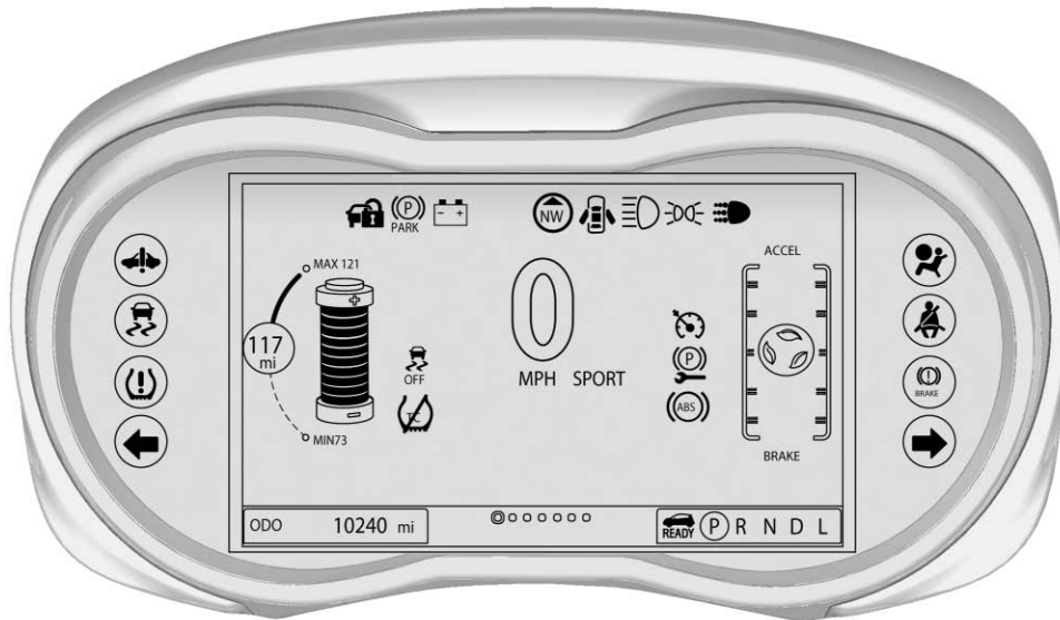
English Cluster with Enhanced Battery Gauge and Driver Efficiency Gauge Shown, Others and Metric Similar
