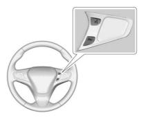
If equipped with OnStar<sup>®</sup> or a Bluetooth<sup>®</sup> system, press to interact with those systems. See OnStar Overview ⇔ 383, Bluetooth (Infotainment Controls) ⇔ 181 or Bluetooth (Overview) ⇔ 180, or "Bluetooth (Overview)" in the infotainment manual. ↔ : Press to reject an incoming call or end a current call. Press to mute or unmute the infotainment system when not on a call.
