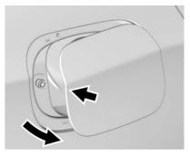
The fuel cap is behind a hinged fuel door on the passenger side of the vehicle. To open the fuel door, push and release the rearward center edge of the door.
