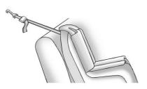
If you are using a single tether in the center seating position, or the rear outboard head restraint has been removed, route the single tether over the seatback.
