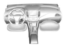
The driver knee airbag is below the steering column. The front outboard passenger knee airbag is below the glove box.
