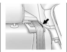
2. Unbuckle the rear safety belt and make sure the safety belt is in the guide on top of the seatback.
