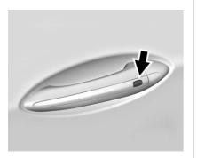
If equipped, press the button on the driver door handle when the RKE transmitter is within 1 m (3 ft) of the driver door handle. When unlocking from the driver door, the first press unlocks that door; press again within five seconds to unlock all passenger doors. See *Remote Keyless Entry (RKE) System Operation (Key Access)* \$ 34 or *Remote Keyless Entry (RKE) System Operation (Keyless Access)* \$ 36.
