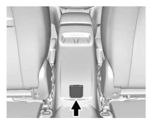
The power outlet is on the rear of the center console.
