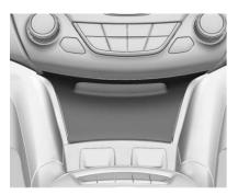
The instrument panel fuse block is in the center of the console, under the heater, ventilation, and air conditioning controls. To access the fuses:
