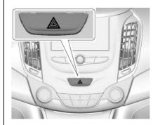
A: Press to make the front and rear turn signal lamps flash on and off. This warns others that you are having trouble. Press again to turn the flashers off.
