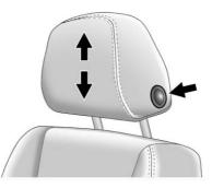
The height of the head restraint can be adjusted. To raise or lower the head restraint, press the button located on the side of the head restraint, and pull up or push the head restraint down, and release the button. Pull and push on the head restraint after the button is released to make sure that it is locked in place.
