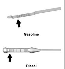
If the oil is below the cross-hatched area at the tip of the dipstick and the engine has been off for at least 15 minutes, add 1 L (1 qt) of the recommended oil and then recheck
