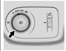
The exterior lamp control is to the left of the steering column on the instrument panel.
