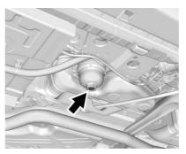
The fuel filter is under the vehicle on the driver side in front of the left rear tire. For replacement of the filter, see *Fuel Filter Replacement* (*Diesel*)  $\Rightarrow$  258. Also see *Maintenance Schedule*  $\Rightarrow$  352 for recommended draining and replacement intervals.
