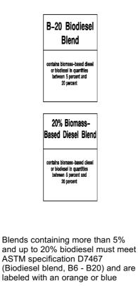
pump label. To reduce the risk of poor quality fuel, purchase biodiesel blends from a fuel supplier or fueling station that sells BQ-9000<sup>®</sup> certified biodiesel. See www.bq-9000.org for a list of certified marketers. For detailed information on the use of biodiesel, see *Biodiesel*  $\Rightarrow$  253.
