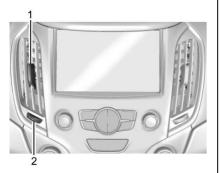
Move the slats (1) to change the direction of the airflow.
