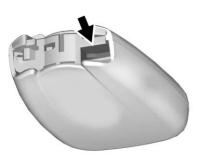
2. Separate the two halves of the transmitter using a flat tool inserted into the area near the key slot.
