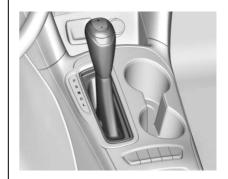
**P**: This position locks the drive wheels. It is the best position to use when starting the engine because the vehicle cannot move easily.
