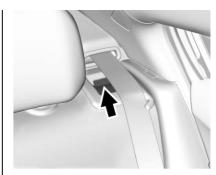
A tab near the seatback lever retracts when the seatback is locked in place.
