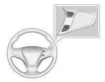
If equipped with OnStar<sup>®</sup> or a Bluetooth<sup>®</sup> system, press to interact with those systems. See OnStar Overview ⇔ 383, Bluetooth (Infotainment Controls) ⇔ 181 or Bluetooth (Overview) ⇔ 180, or "Bluetooth (Overview)" in the infotainment manual. ↔ : Press to reject an incoming call or end a current call. Press to mute or unmute the infotainment system when not on a call.
