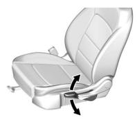
If equipped, move the lever up or down to manually raise or lower the seat.
