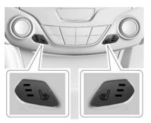
If equipped, the controls are on the center stack. The engine must be running to operate the heated seats.
