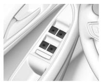
The windows work when the vehicle is in ON/RUN, ACC/ACCESSORY, or Retained Accessory Power (RAP). See *Retained Accessory Power (RAP)* ⇔ 219.
