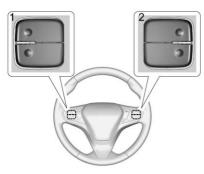
The favorite and volume switches are on the back of the steering wheel.
