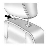
To lower the head restraint, press the button located on the top of the seatback and push the head restraint down. Try to move the head restraint after the button is released to make sure it is locked in place. The rear outboard head restraints are designed to be removed. See "Head Restraint Removal and Reinstallation" under *Lower Anchors and Tethers for Children (LATCH System)* ⇔ 92.
