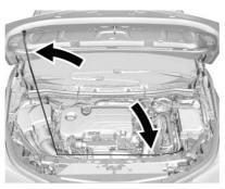
Go to the front of the vehicle and lift the hood and release the hood prop from its retainer, located above the radiator. Securely place the hood prop into the slot on the underside of the hood. To close the hood:
