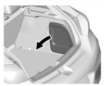
2. Open and remove the storage compartment door. Store the door under the rear floor storage cover.
