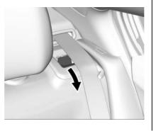
Reach under the safety belt and pull the lever on top of the seatback to unlock the seatback. A tab near the seatback lever moves forward when the seatback is unlocked.
