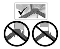
Position the jack lift head at the jack location nearest the flat tire. The location is indicated by a notch on the bottom edge of the body side.
