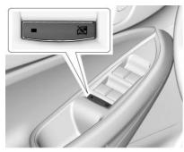
This feature stops the rear door passenger window switches from working.
