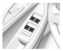
Press the switch down to open the window. Pull the switch up to close it. See *Power Windows* ⇔ 55.
