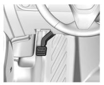
With the brake pedal applied, push the parking brake pedal down. See *Shifting Into Park*  $\Rightarrow$  219 or *Parking*  $\Rightarrow$  221.
