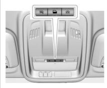
$\stackrel{}{\not\sim}$ : Press to turn the lamps off, even when a door is open.
