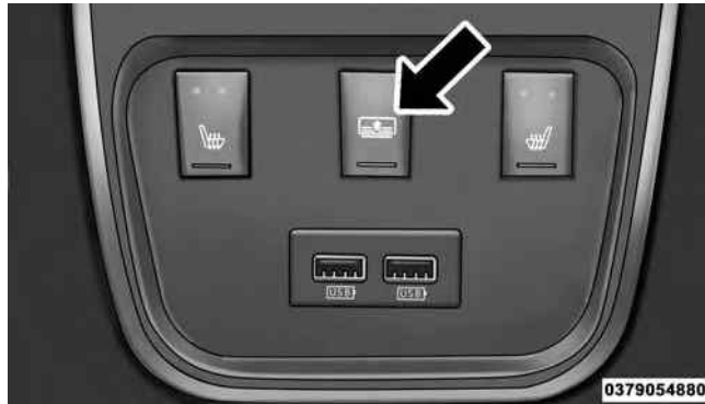
Power Sunshade Switch
