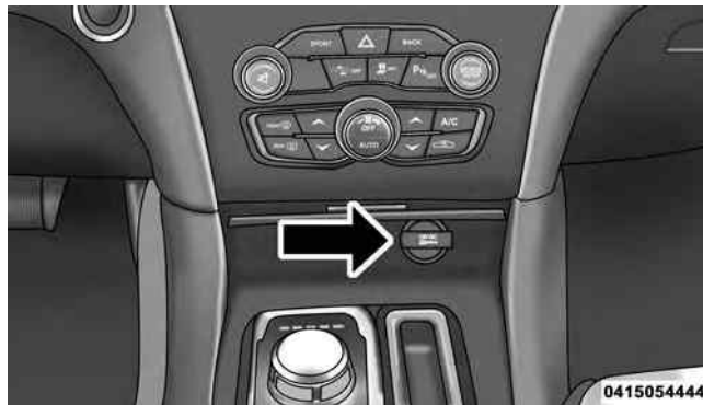
Front Power Outlet
