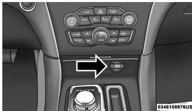
Front Power Outlet
