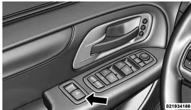
Power Vent Window Switch Open/Close
