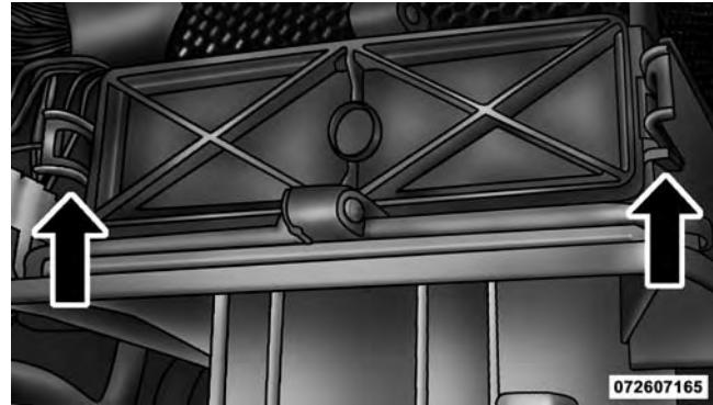
A/C Air Filter Replacement
