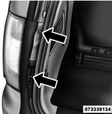
Tail Lamp Mounting Screws
