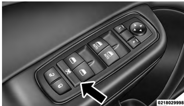
Window Lockout Switch
