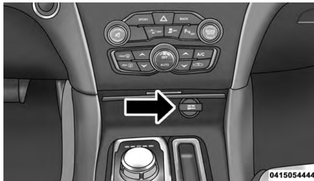
Front Power Outlet
