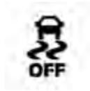
The “ESC OFF Indicator Light” indicates the customer has elected to have the Electronic Stability Control (ESC) in a reduced mode.
