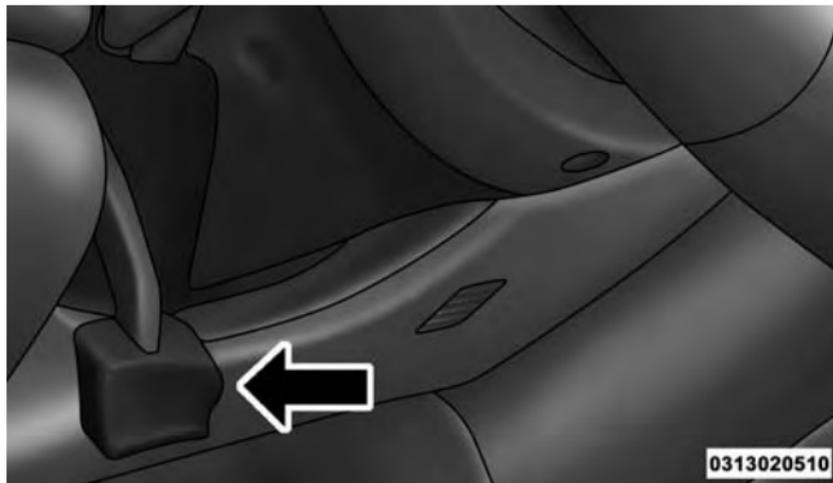
Tilt/Telescoping Steering Control Handle
