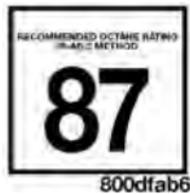
These engines are designed to meet all emissions regulations and provide optimum fuel economy and performance when using high quality unleaded “Regular” gasoline having a posted octane number of 87 as specified by the (R+M)/2 method. The use of higher octane “Premium” gasoline is not required, as it will not provide any benefit over “Regular” gasoline in these engines.
