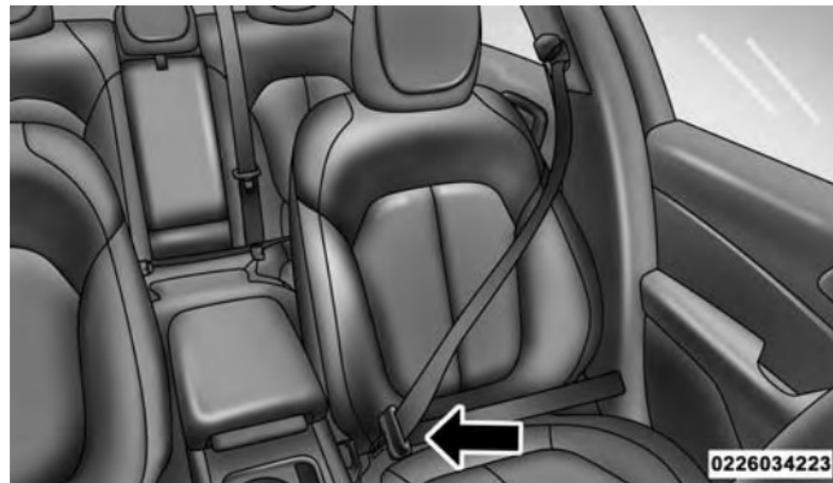
**Inserting Latch Plate Into Buckle**
