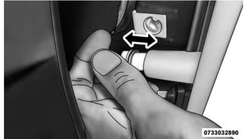
**Front Side Marker Lamp Bulb Removal**
