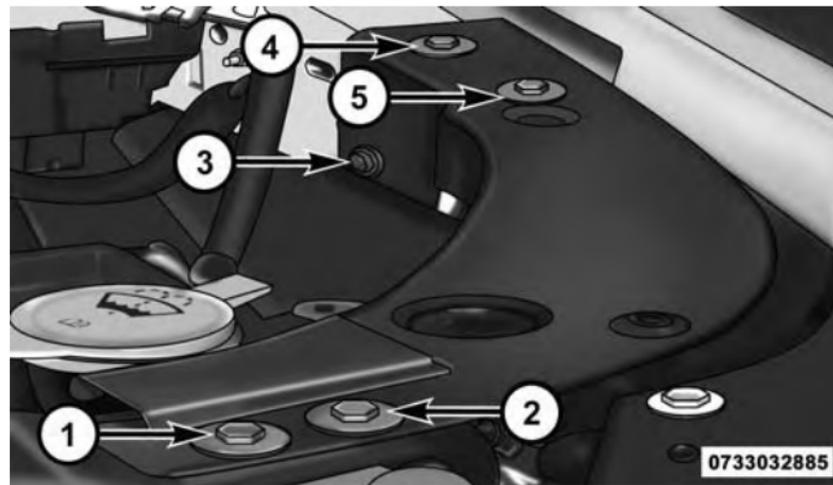
**Brace Bolt Tightening Sequence**
