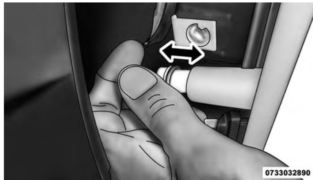
Front Side Marker Lamp Bulb Removal
