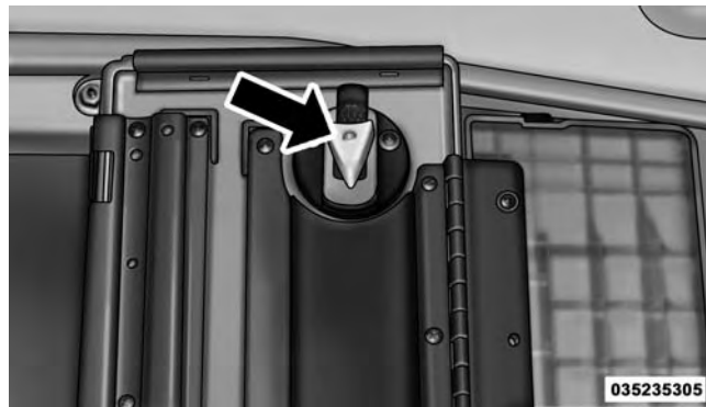
Storage Bin Cover Emergency Release Lever
