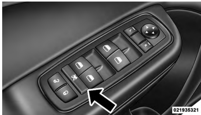
Window Lockout Switch
