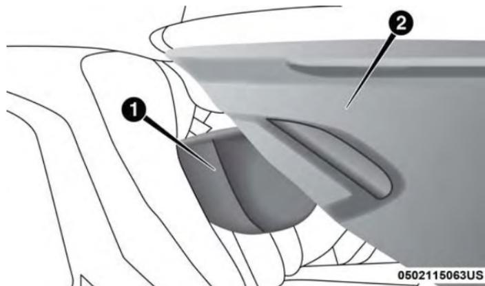
Car Seat With Head Restraint Folded
