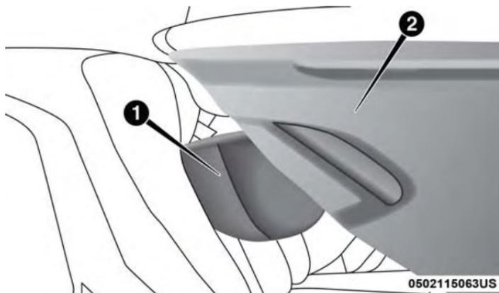
Car Seat With Head Restraint Folded
