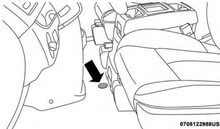
Winch Cover Assembly Plug (If Equipped)
