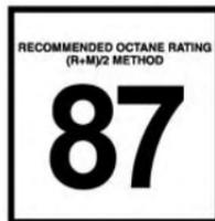
This engine is designed to meet all emissions regulations and provide excellent fuel economy and performance when using high-quality unleaded “Regular” gasoline having an octane rating of 87 as specified by the (R+M)/2 method. The use of higher octane “Premium” gaso-
